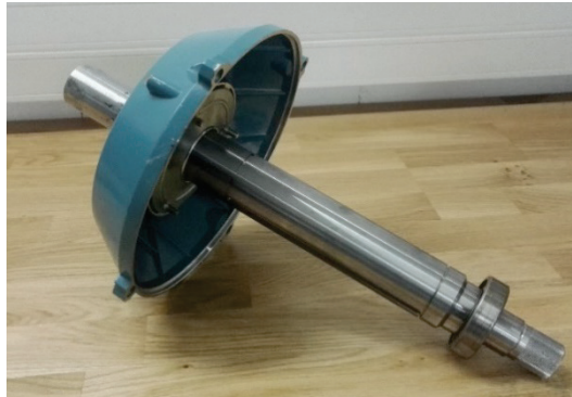
Figure 5.14. Replacement of the rotor of SynRM with the shaft.
