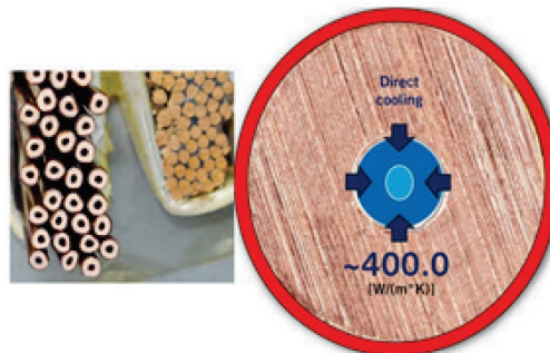
Figure 1.9. Example of direct conductor cooling [10].
