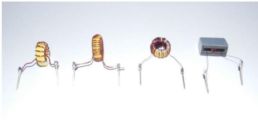
Figure 10. Cores with secondary windings
