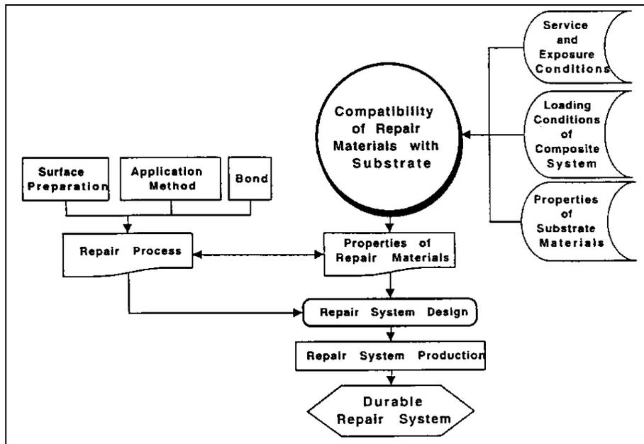
Figure 2.3.2 Factors affecting the durability of concrete repair systems according to Emmons and Vaysburd 1995 [9]
