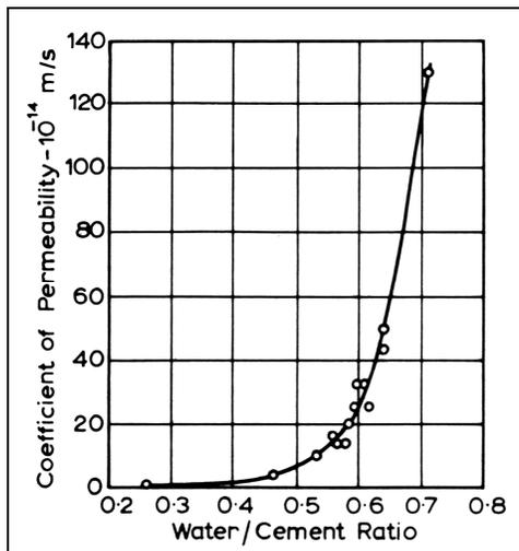
Figure 2.6 Relation between permeability and water/cement ratio for mature cement pastes (93% of cement hydrated)
