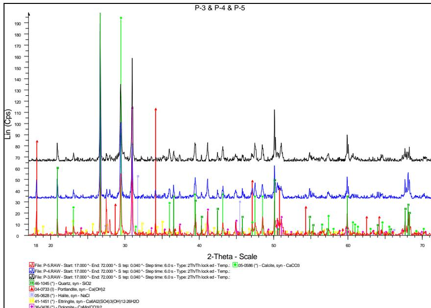
Figure 5.17 Powder diffractogram of X ray analysis of Papisaare hydroplane hangar column concrete, samples from the depth of 40 mm (sample P3) up to 100 mm (sample P5) from the outer surface
