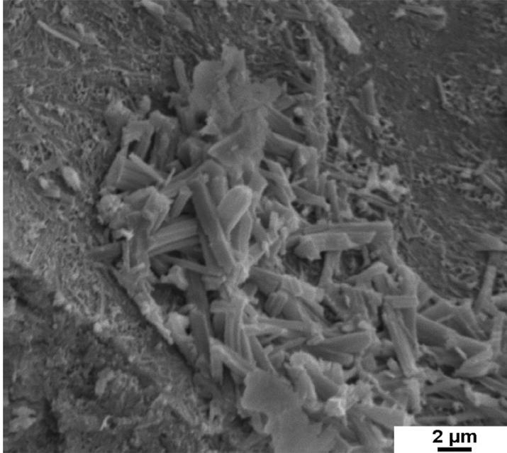
Figure 5.24 Concrete fracture surface taken in the depth of 40-50 mm of the hydroplane hangar shell
