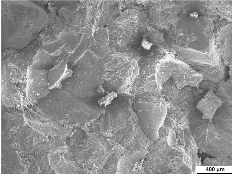
Figure 5.29 Concrete fracture surface taken in the depth of 20-40 mm (sample P2) of the Papisaare hydroplane hangar reinforced concrete column
