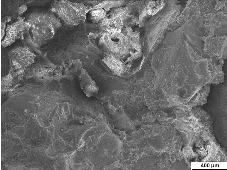
Figure 5.25 Concrete fracture surface taken in the depth of 20-40 mm (sample L2) of the hydroplane hangar reinforced concrete column
