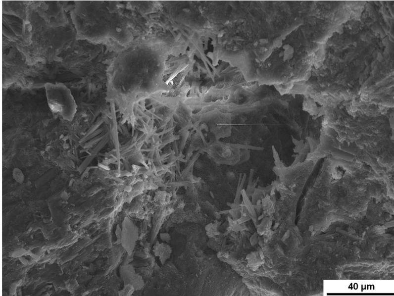
Figure 5.32 Concrete fracture surface taken in the depth of 80-100 mm (sample P5) of the Papisaaire hydroplane hangar reinforced concrete column
