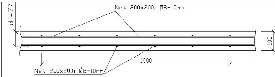
Figure 6.7 Section of the reinforced concrete shell roof
