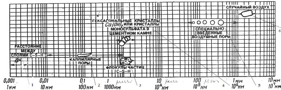
Figure 2.4 Structure of the cement stone: 1 – distance between the layers of C-S-H crystals; 2 – capillary pores; 3 – C-S-H crystals; 4 –  $\text{Ca}(\text{OH})_2$  crystals and crystals of mono sulfate; 5 – entrained air; 6 – air bubbles [10]
