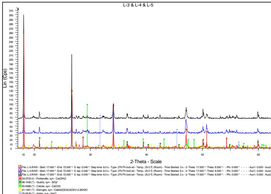
Figure 5.14 Powder diffractogram of X ray analysis of the Tallinn hydroplane hangar column concrete samples from the depth of 40 mm (sample L3) up to 100 mm (sample L5) from the outer surface
