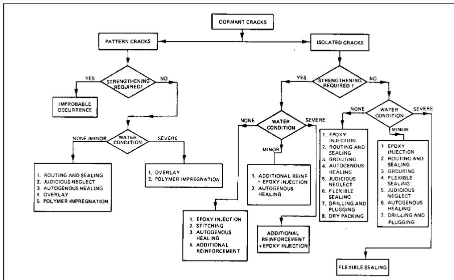
Figure 2.3.4 Selection of repair method for dormant cracks after Johnson [9]
