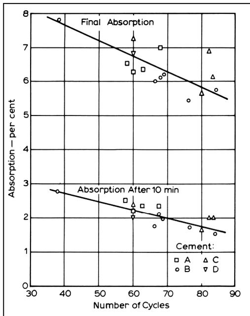
Figure 2.15 Relation between the absorption of concrete and the number of cycles of freezing and thawing required to cause a 2% reduction in the mass of the specimen [1]
