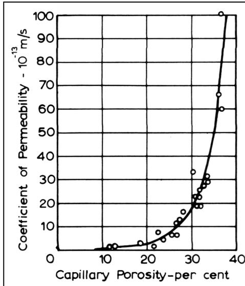
Figure 2.5 Relation between permeability and capillary porosity of cement paste [1]
