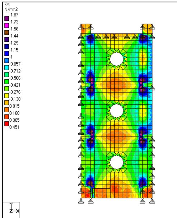
Figure 6.3 Diagram of the normal stresses  $f_x$
