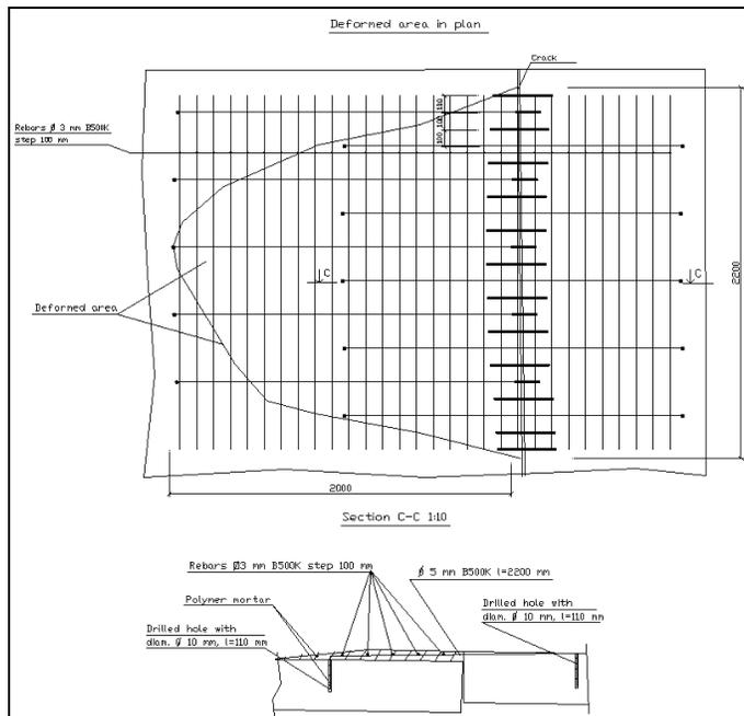
Figure 7.2 Structural solution – deformed area A
