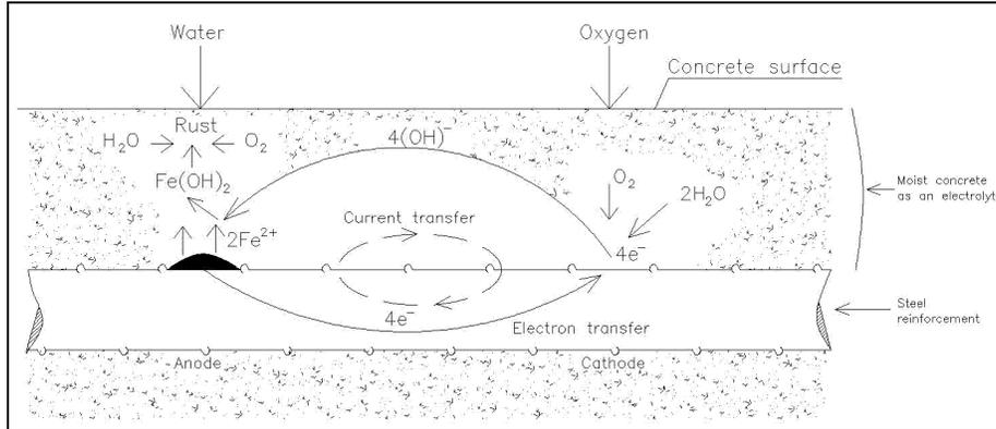
Figure 2.7 Simplified model of the corrosion process of reinforcement steel in concrete
