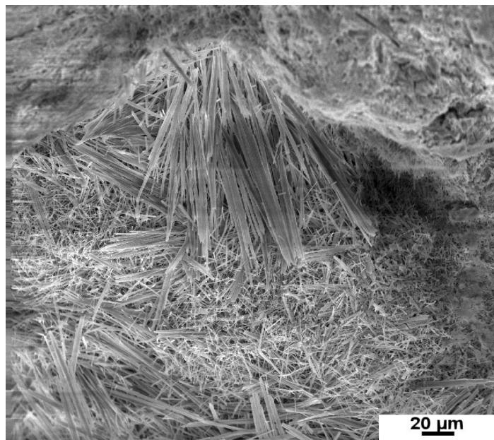
Figure 5.23 Concrete fracture surface taken in the depth of 40-50 mm of the hydroplane hangar shell
