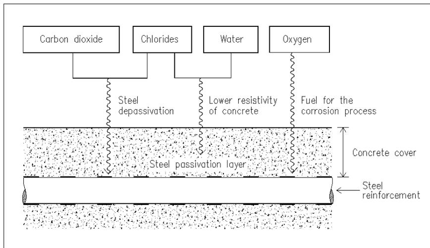
Figure 2.9 Critical environmental factors on corrosion of steel reinforcement
