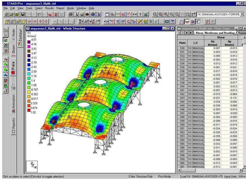
Figure 6.2 Calculation scheme of Tallinn hydroplane hangars in the Staad/Pro program
