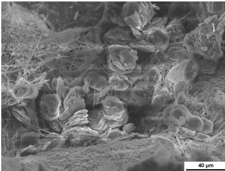
Figure 5.26 Concrete fracture surface taken in the depth of 20-40 mm (sample L2) of the hydroplane hangar reinforced concrete column
