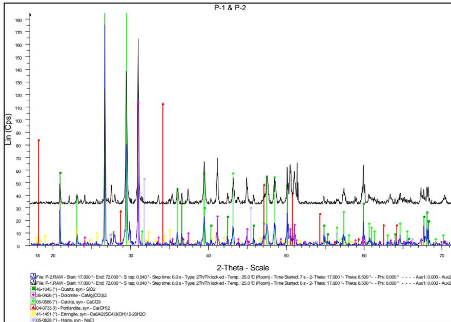
Figure 5.16 Powder diffractogram of X ray analysis of Papisaare hydroplane hangar column concrete, samples from the depth of 0–20 mm (sample P1) and 20–40 mm (sample P2) from the outer surface
