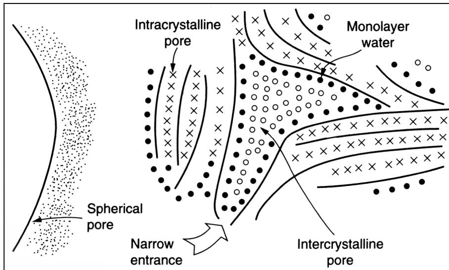
Figure 2.1 Diagrammatic representation of the pore system in hydrated cement paste based on Rahman's model [13]
