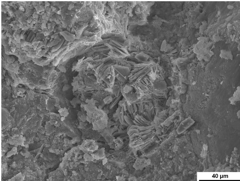
Figure 5.28 Concrete fracture surface taken in the depth of 80-100 mm (sample L5) of the hydroplane hangar reinforced concrete column
