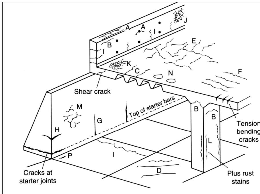
Figure 2.16 Schematic representation of the various types of cracking which can occur in concrete (see Table 2.8) [20]
