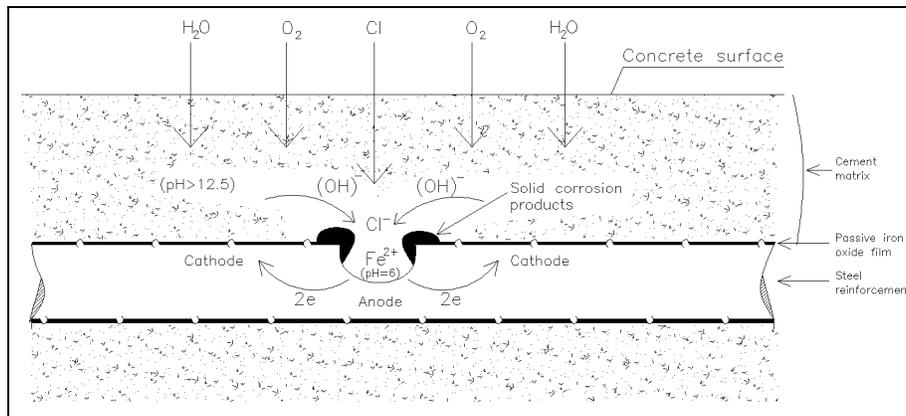
Figure 2.12 Pitting corrosion caused by chlorides
