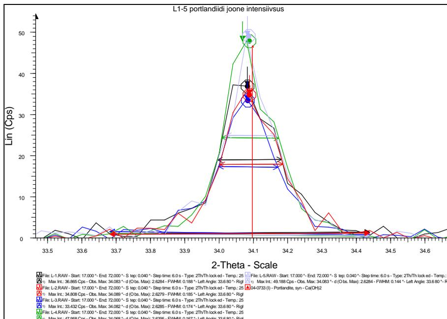
Figure 5.15 Powder diffractogram of X ray analysis of the Tallinn hydroplane hangar column concrete,  $\text{Ca(OH)}_2$  relative concentrations (intensities), samples from the depth of outer surface (sample L1) up to 100 mm of depth on the inner surface (sample L5)
