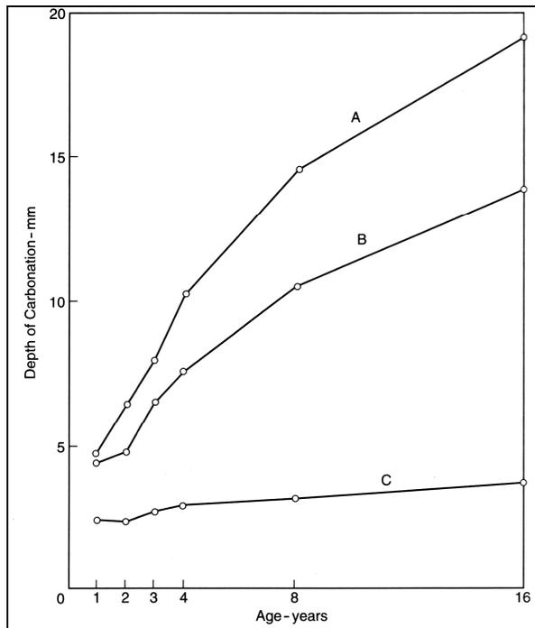
Figure 2.11 Progress of carbonation with time of exposure under different conditions: (A) 20 °C and 65% relative humidity; (B) outdoors, protected by a roof; (C) horizontal surface outdoors in Germany. The values are averages for concretes with water/cement ratios of 0.45, 0.60 and 0.80, wet-cured for 7 days (based on [19])
