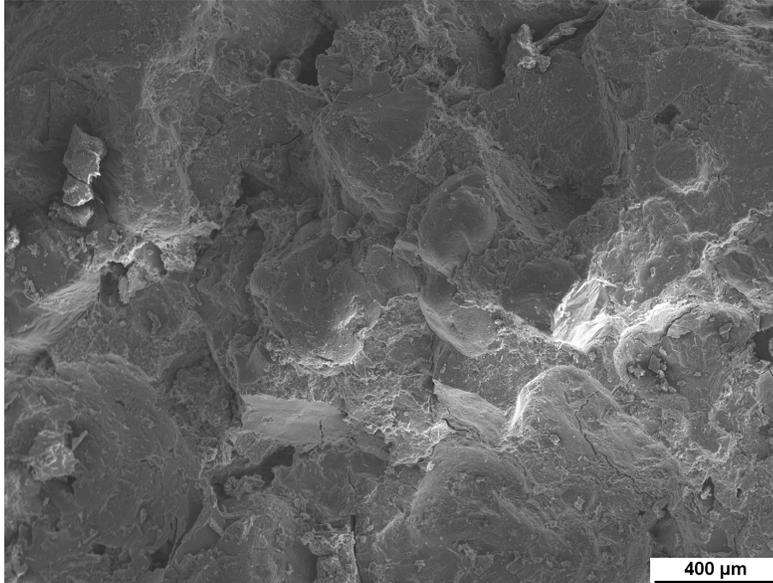
Figure 5.27 Concrete fracture surface taken in the depth of 80-100 mm (sample L5) of the hydroplane hangar reinforced column
