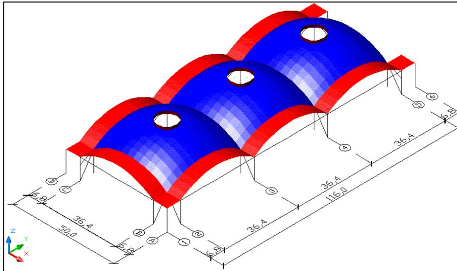
Figure 5.1 Dimensions of the hangar
