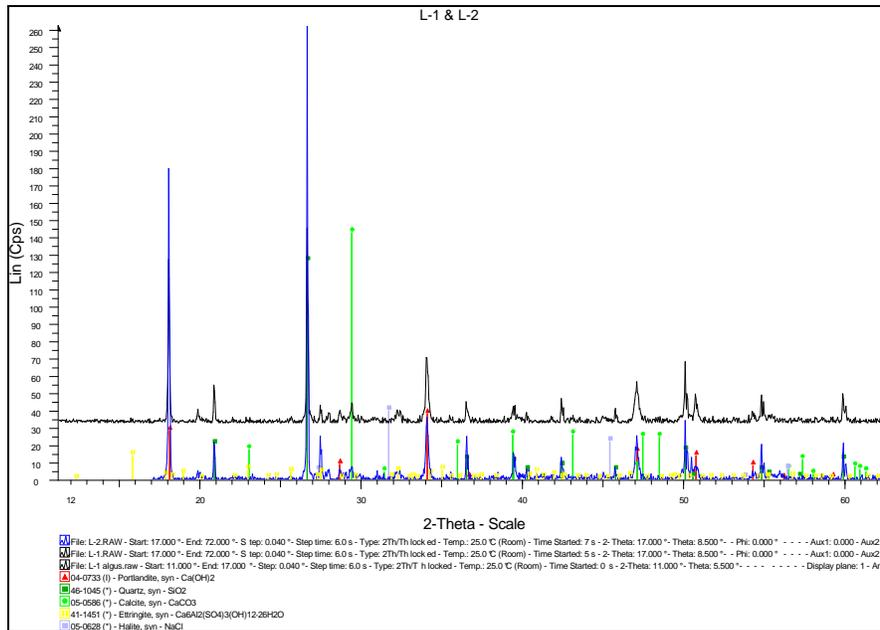
Figure 5.13 Powder diffractogram of X ray analysis of the Tallinn hydroplane hangar column, samples from the depth of 0 - 20mm (sample L1) and 20 – 40 mm (sample L2) from the outer surface
