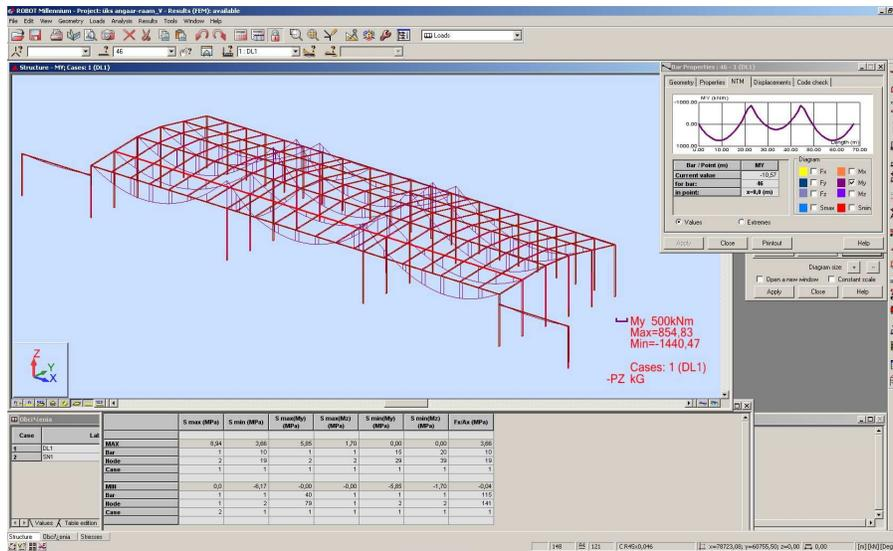
Figure 6.4 Calculation scheme of Papisaae hydroplane hangars in the Robot Millennium program
