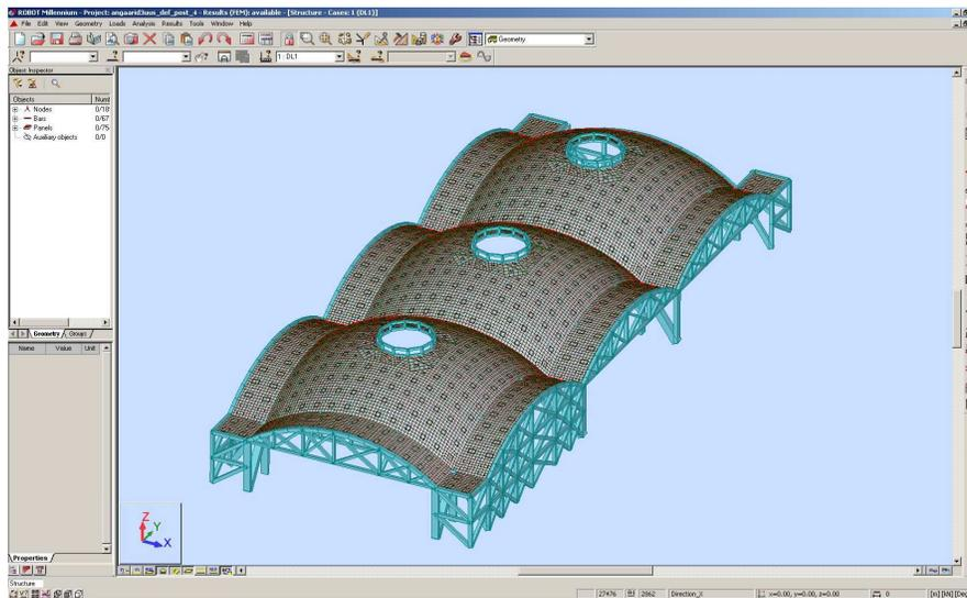
Figure 6.1 Calculation scheme of Tallinn hydroplane hangars in the Robot Millennium program
