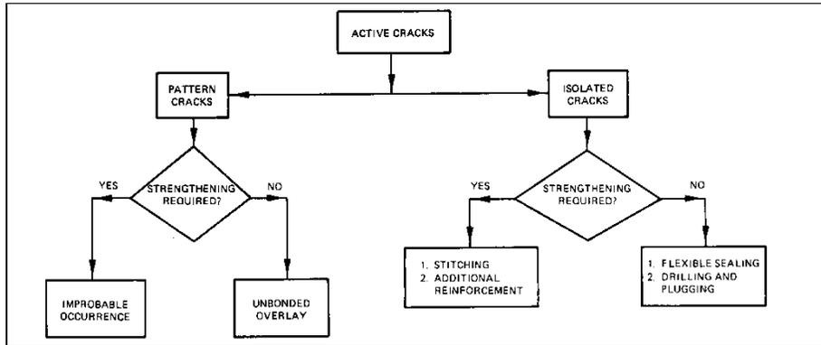
Figure 2.3.3 Selection of repair method for active cracks after Johnson [9]
