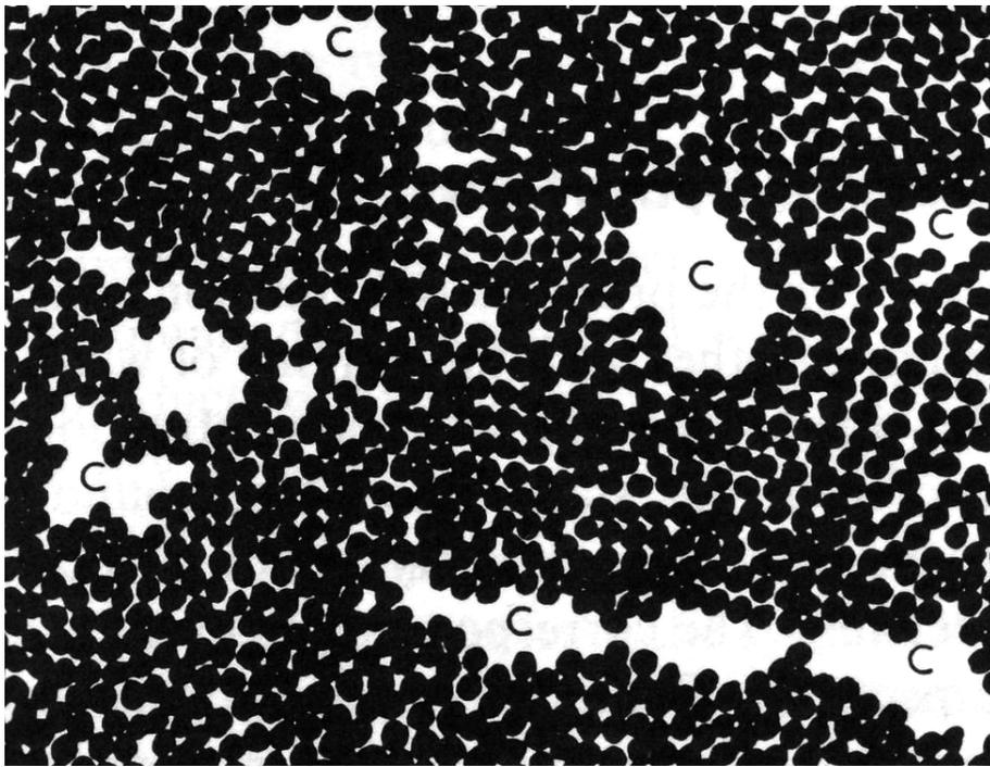
Figure 2.3 Simplified model of paste structure. Solid dots represent gel particles; interstitial spaces are gel pores; spaces such as those marked C are capillary pores. Size of a gel pore is exaggerated [1]
