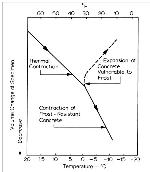
Figure 2.14 Change in volume of frost-resistant and vulnerable concretes in cooling [1]
