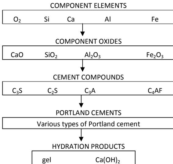
Figure 2.2 Schematic representation of the formation and hydration of Portland cement [1]
