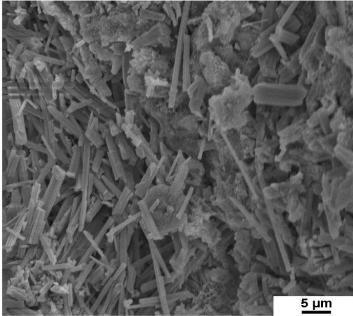
Figure 5.20 Concrete fracture surface taken in the depth of 40-50 mm of the hydroplane hangar shell
