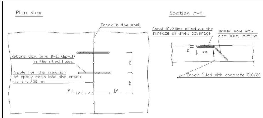
Figure 7.7 Reinforcement and injection of cracks
