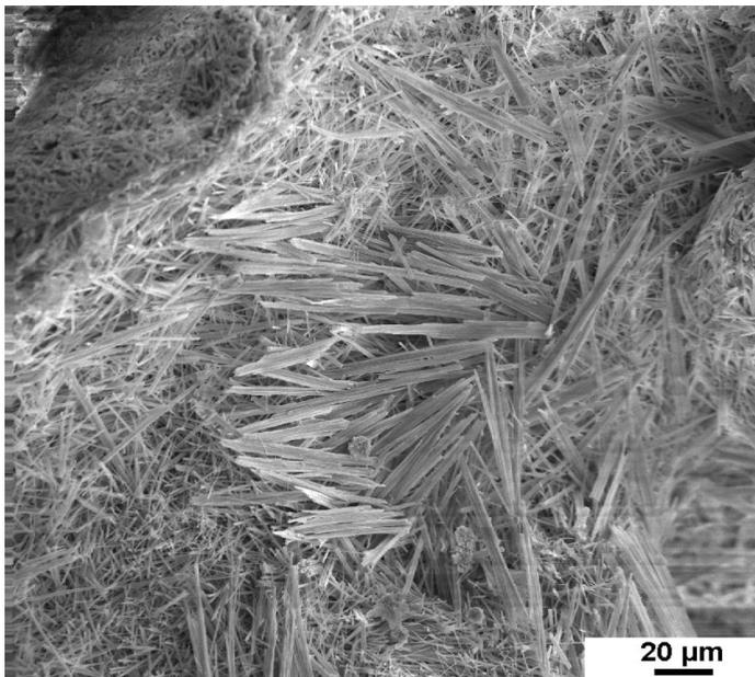
Figure 5.21 Concrete fracture surface taken in the depth of 40-50 mm of the hydroplane hangar shell
