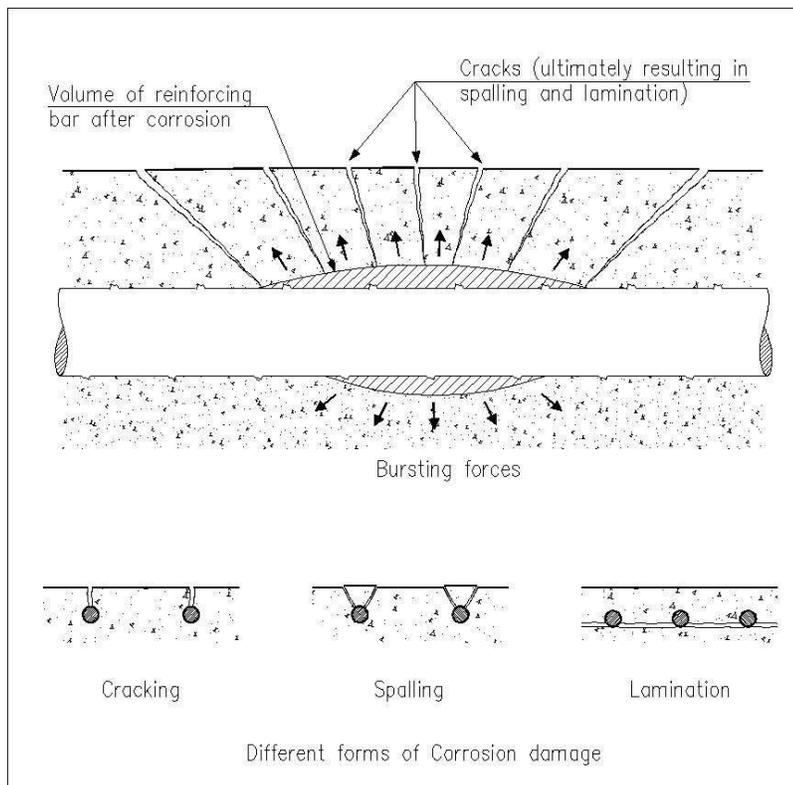
Figure 2.8 Cracking and spalling of concrete caused by corrosion of the reinforcement [3]
