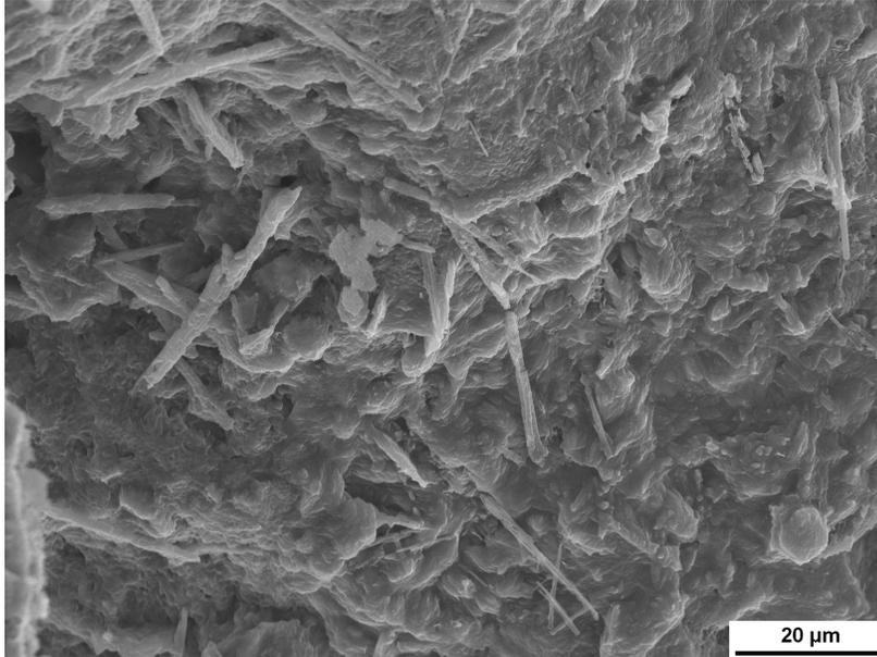
Figure 5.30 Concrete fracture surface taken in the depth of 20-40 mm (sample P2) of the Papisaare hydroplane hangar reinforced concrete column
