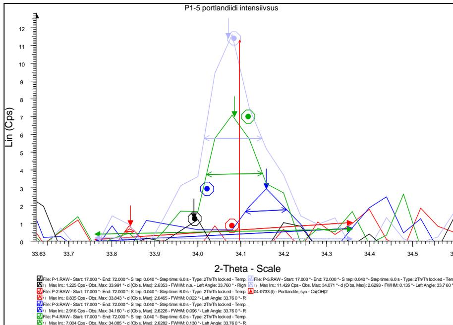
Figure 5.18 Powder diffractogram of X ray analysis of Papisaare hydroplane hangar column concrete, relative concentrations (intensities) of  $\text{Ca(OH)}_2$ , samples from the depth, outer surface, (P1) up to 100 mm of column depth, on the inner surface (P5)
