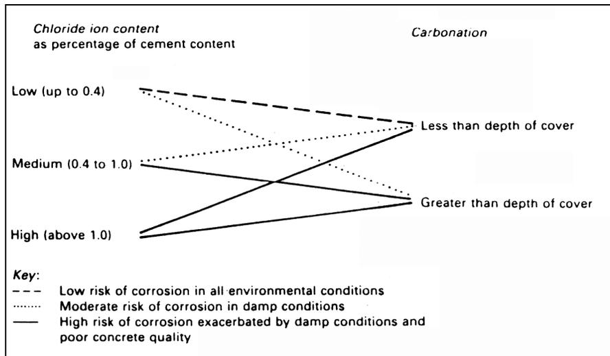
Figure 2.13 Risk of corrosion in relation to concrete analysis [3]
