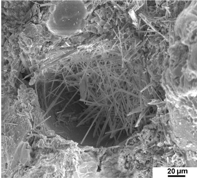
Figure 5.22 Concrete fracture surface taken in the depth of 40-50mm of the hydroplane hangar shell
