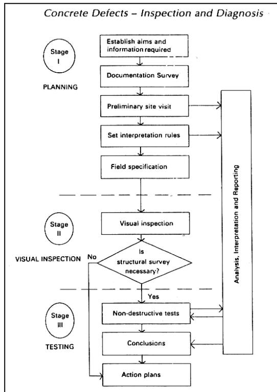
Figure 2.17 Flowchart to illustrate the inspection process [3]
