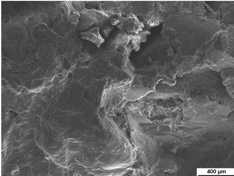
Figure 5.31 Concrete fracture surface taken in the depth of 80-100 mm (sample P5) of the Papisaare hydroplane hangar reinforced concrete column
