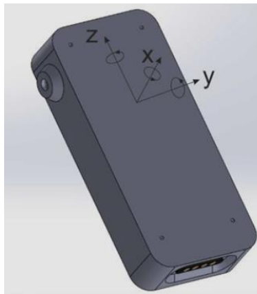
Figure 3.3: The global coordinate system of the IMU sensor.
