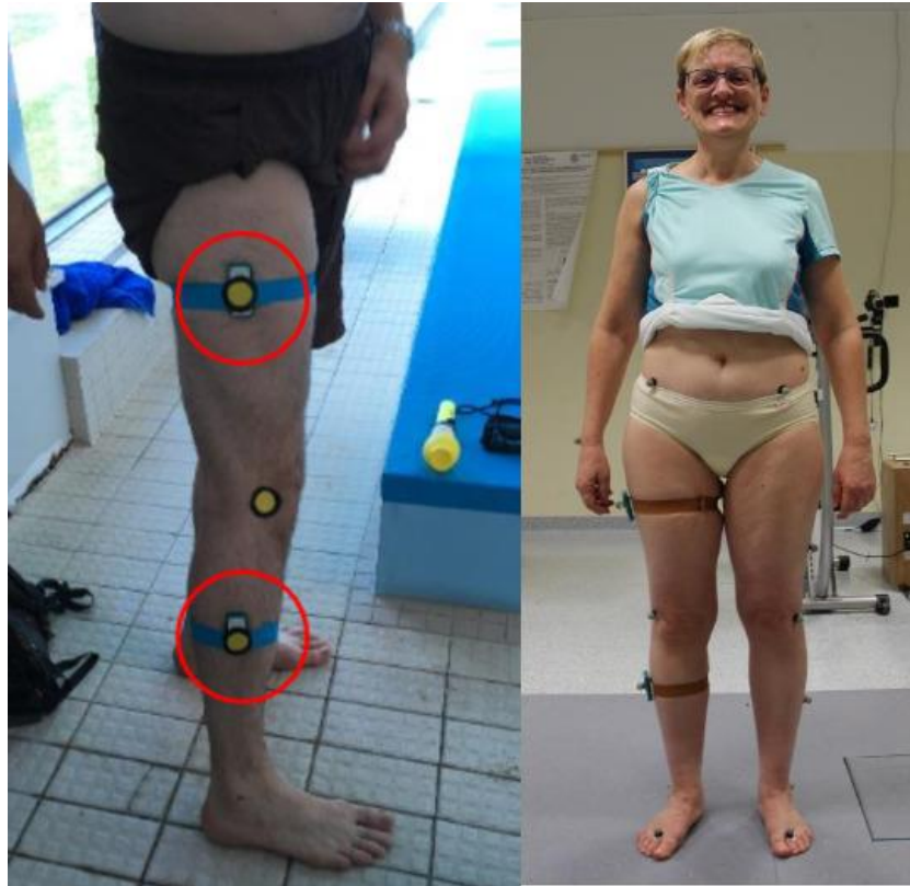
Figure 3.2: IMU sensors attachment to the Thigh and Shank of each subject.
