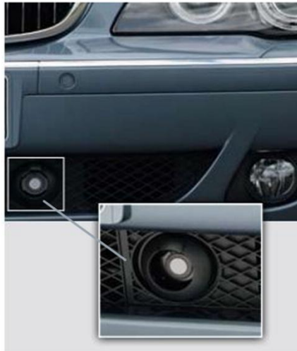
Fig 11. Camera installation inside the grille
