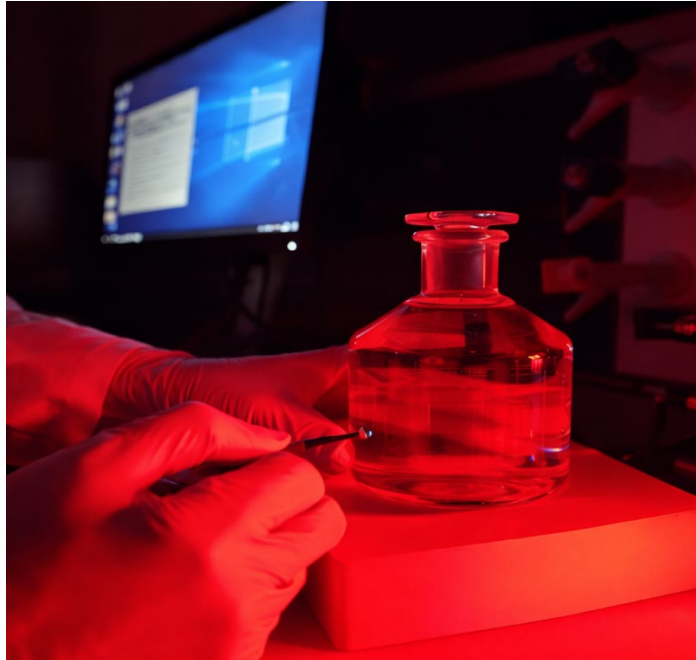
Figure 4. Modified oxygen measurement system used in the closed bottle test, employing a PreSens fiber-optic sensor integrated with OxyView software.
