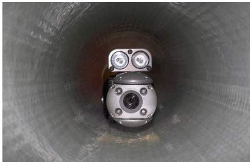
Figure 5: Pipeline Inspection Robot using Camera
