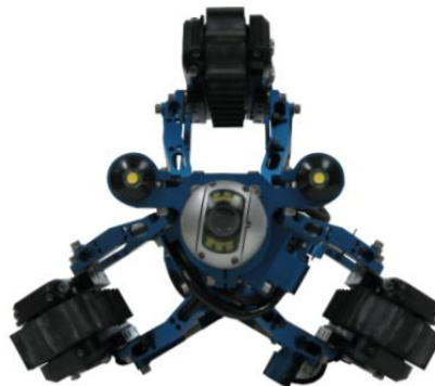
Figure 14: VT100 vertical crawler [29]
