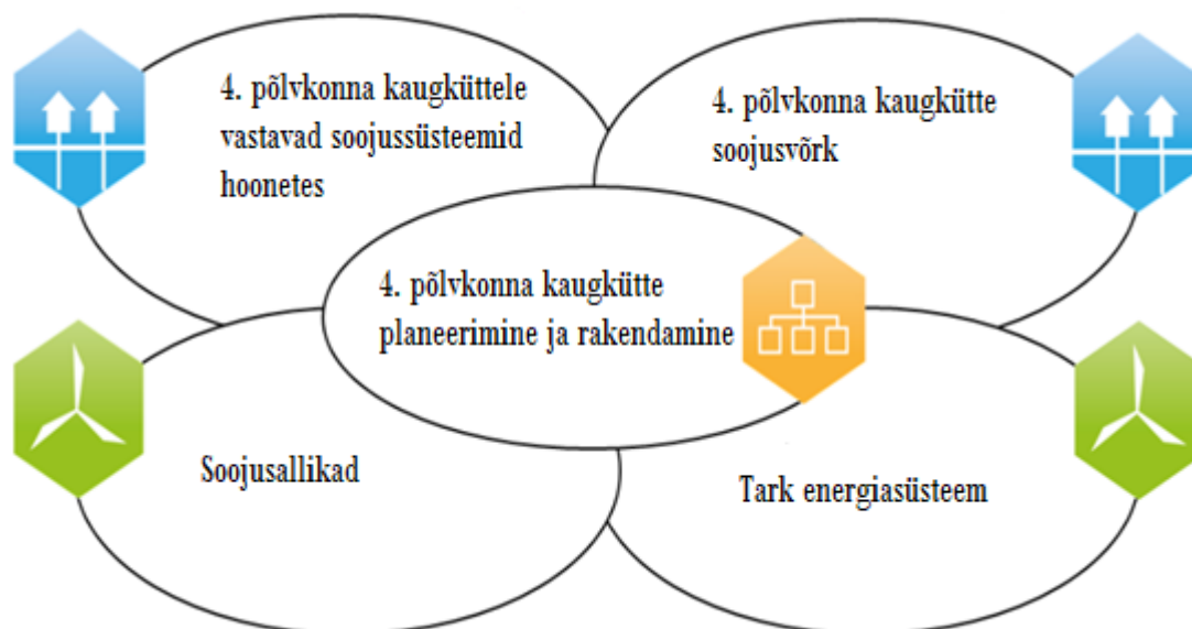
Joonis 2.5. Neljanda põlvkonna kaugkütte kontseptsioon (allikas: H. Lund et al., "4th Generation District Heating (4GDH): Integrating smart thermal grids into future sustainable energy systems" Energy , vol. 68, pp. 1–11, 2014)
