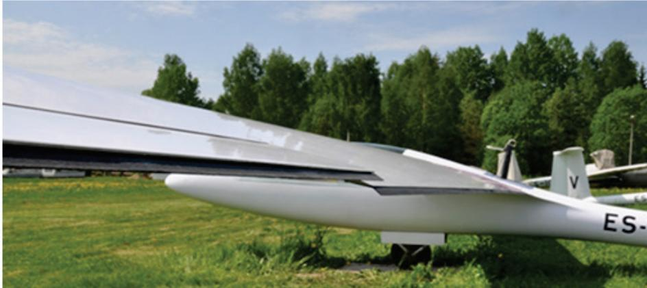
Figure 10. Fixed angle miniflaps on sailplane Jantar-Standard 3 wing.
