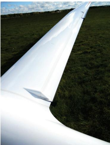
Figure 19. VGMF in extended position.
