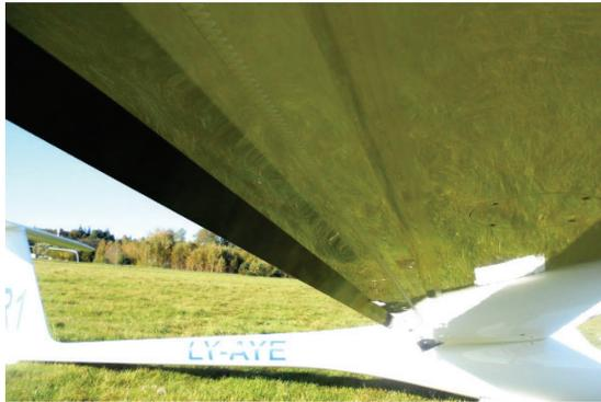
Figure 25. The miniflaps in extended position. The precurved mylar seal coated at the lower side of the flap's trailing edge.
