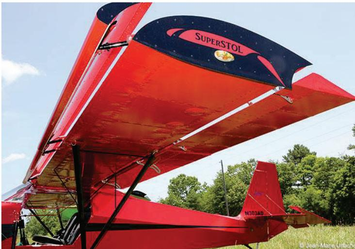
Figure 45. Just Superstol aircraft and its automatic slat mechanism (Cox, 2015).
