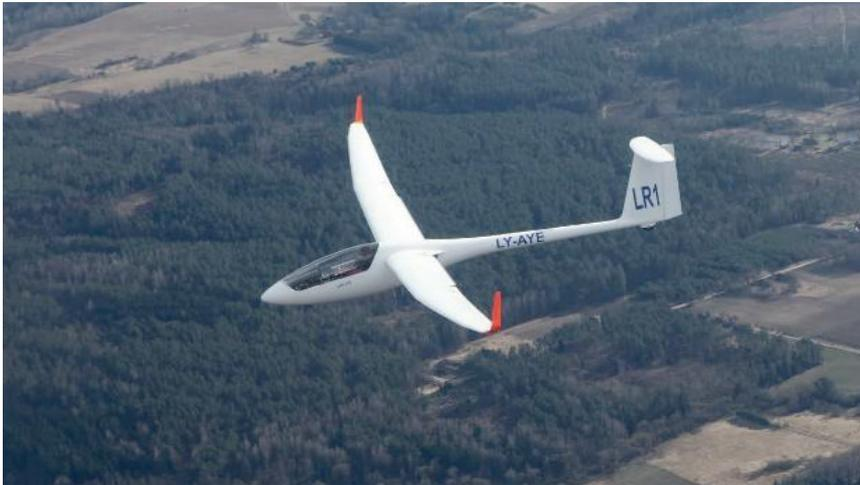
*Figure 21. LAK-17B with VGMF to make a test flight.*
