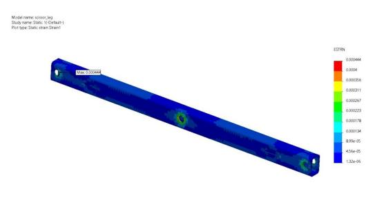
Figure 5.9.3 Strain of scissor link
