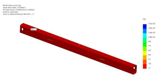
Figure 5.9.4 Factor of safety for scissor link
