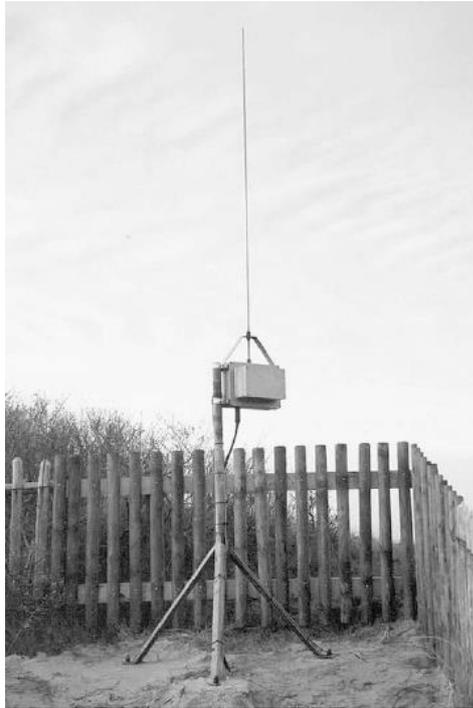
Figure 2.2 ATDnet sensor located in Norderney (Bennet *et al.* 2011).
