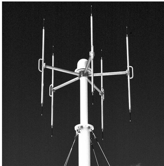
Figure 1.2. Example of a VHF interferometric sensor (Lojou *et al.* 2009).
