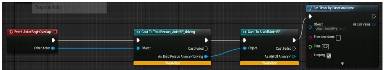
Figure 8. Trigger event followed by the blueprint function attached to it called in by the Cast to function.
