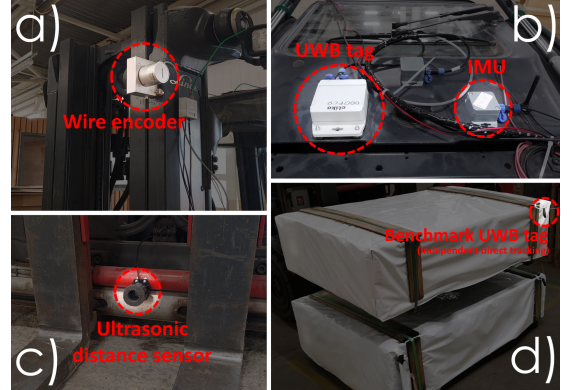
Fig. 4. Deployment of the sensors setup, used in the experimental testing of the proposed indirect tracking method: a) wire encoder sensor attached to the forklift mast; b) positioning unit (UWB tag) and IMU are deployed on top of the forklift; c) ultrasonic distance sensor deployed behind the fork area. d) Industrial products, tracked indirectly (using the proposed method) and directly (using the highlighted independent UWB tag) during the experimental campaign.
