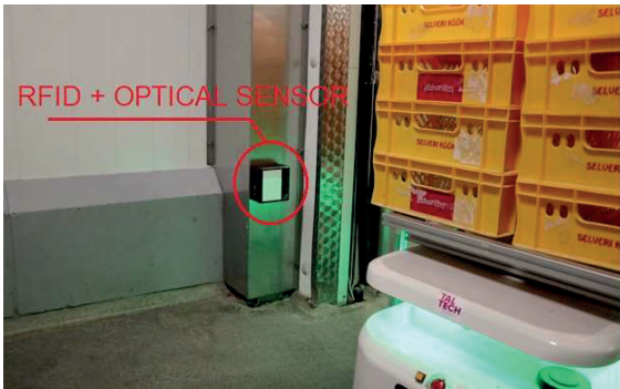
FIGURE 5: RFID AND OPTICAL SENSOR PLACEMENT IN PRODUCTION
