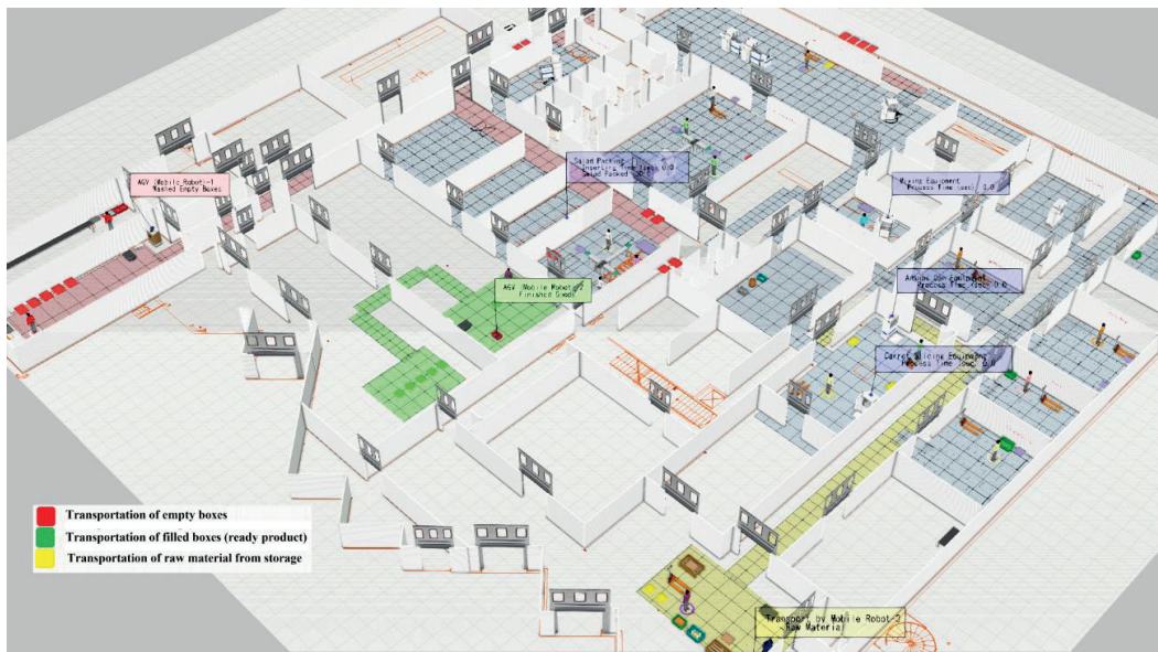
Fig. 4. 3D simulation model of production facility (virtual environment: a holistic view)
