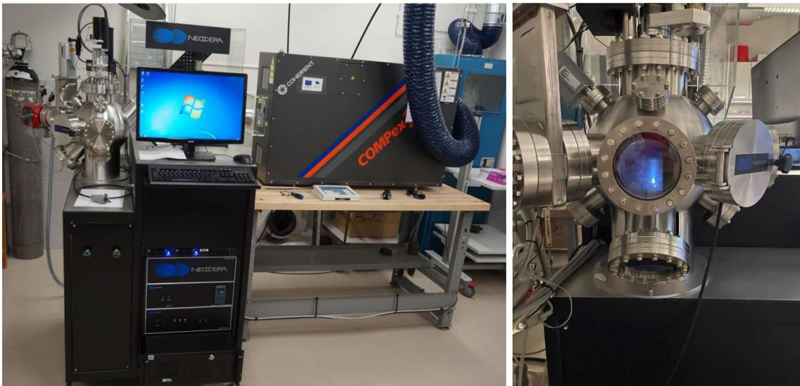
Figure 11 Pulsed laser deposition system Neocera Pioneer 120
