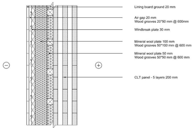
Figure 4.16. Details of layers of Cross-Laminated Timber Walls (V2)
