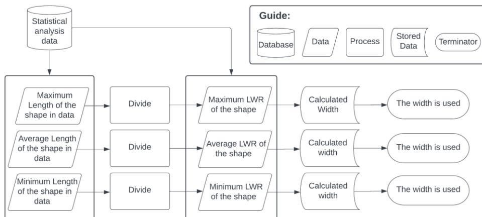
Figure 4.5. Flow chart of the selection of optimal options
