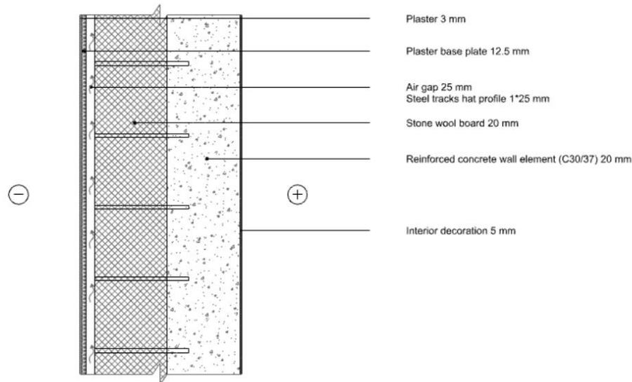
Figure 4.15. Details of layers of Reinforced Concrete Wall (V1)
