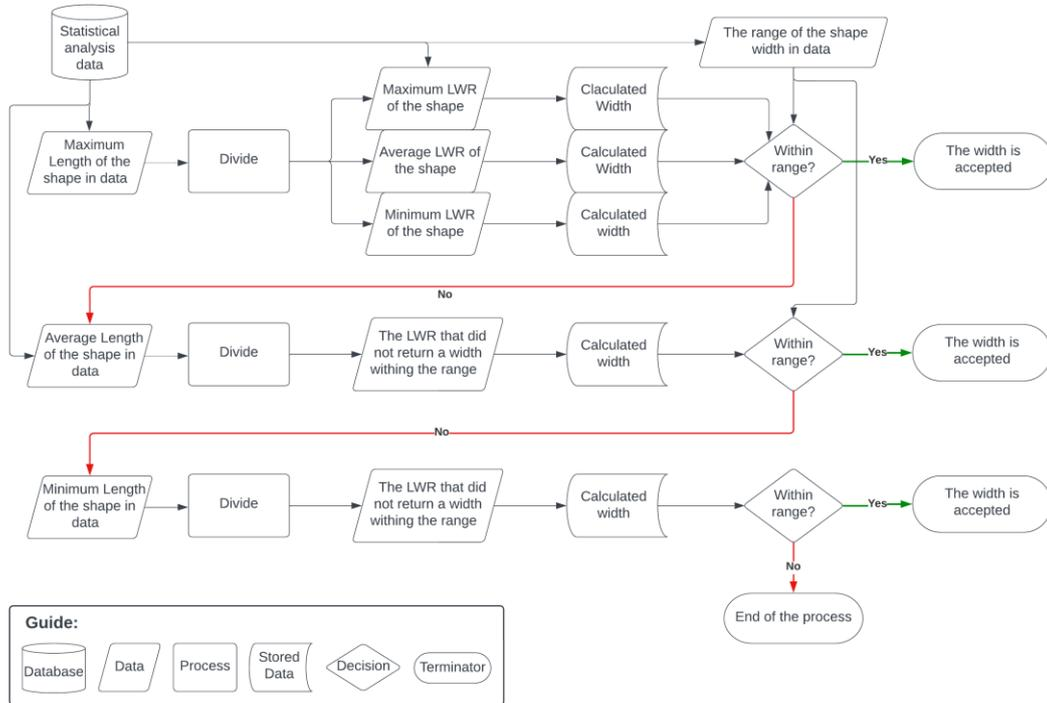
Figure 4.4. Flowchart of the logic of defining building variation dimensions
