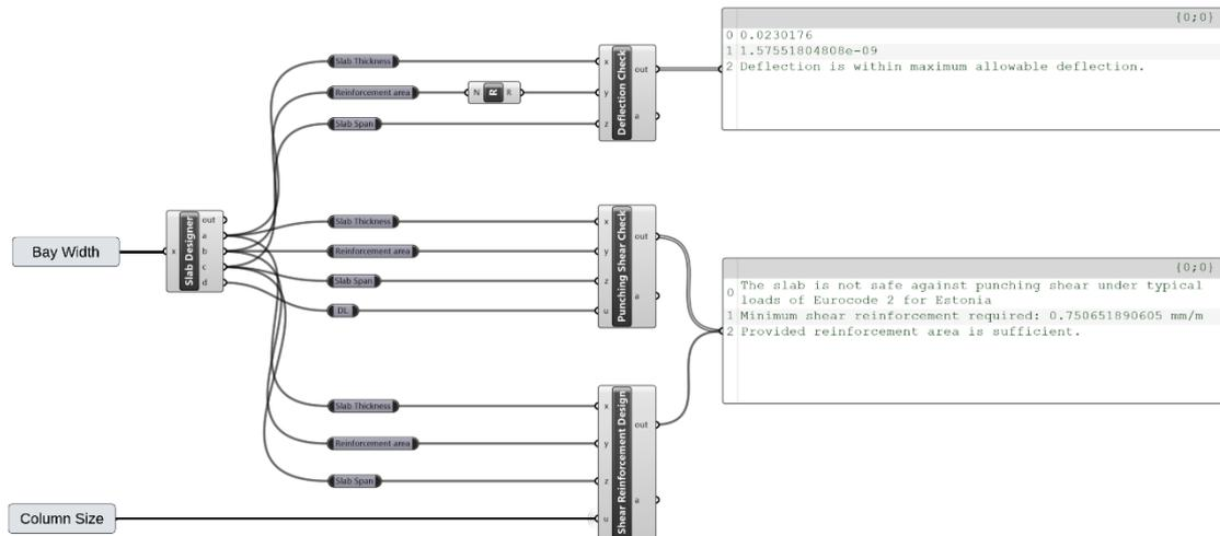
Figure 4.10. Slab design workflow inside Grasshopper
