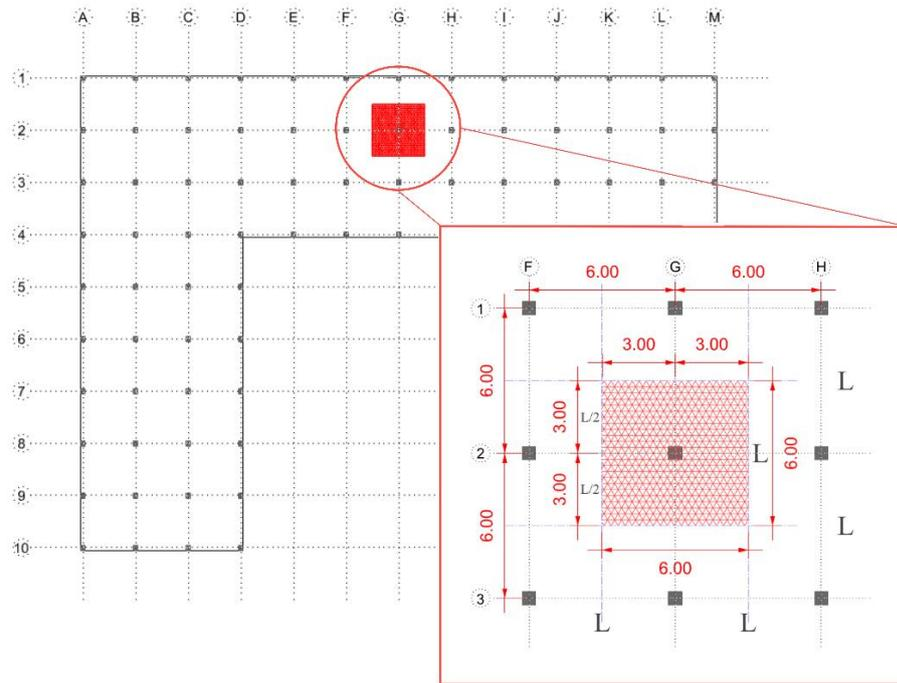
Figure 4.11. A sample column span for a 6-meter-wide bay width
