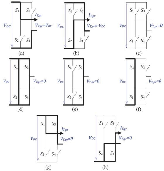
Fig. 2. Typical switching states of the single-phase inverter: (a) and (b) two active states, (c) one unstable state  $V_{T,pr} < V_{DC}$ , (d)–(f) three shoot-through states, and (g) and (h) two zero states.
