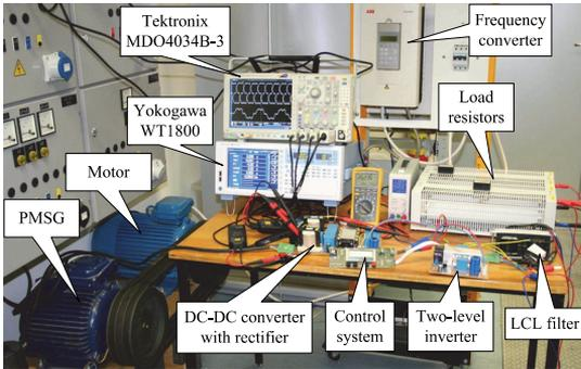
Fig. 10. Test-bench of a small wind energy conversion system.
