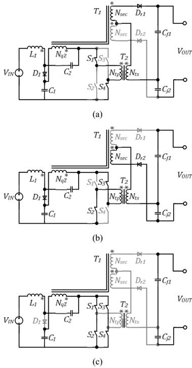
Fig. 7. Equivalent circuits of the proposed topology for: shoot-through states during  $[t_2;t_3]$  and  $[t_4;t_5]$  (a), and active state during  $[t_1;t_2]$  (b) and  $[t_3;t_4]$  (c).
