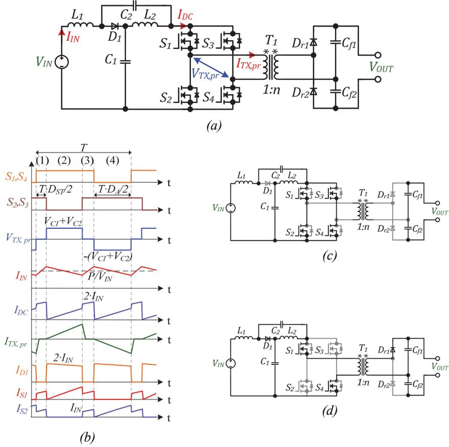
Figure 2.3 Transformer-based qZS GI single-phase full-bridge DC-DC converter [48]: topology (a), sketch of idealized operating waveforms (b), equivalent circuit for the shoot-through state (c), and for the one of active states (d).
