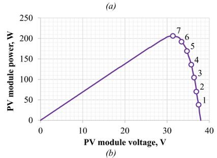
Fig. 3. Selected I-V (a) and P-V (b) characteristics of the PV module.
