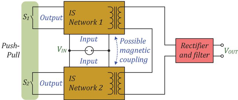
Figure 3.12 Generalized functional scheme of the coupled-inductor-based push-pull GI ISCs [PAPER-I].
