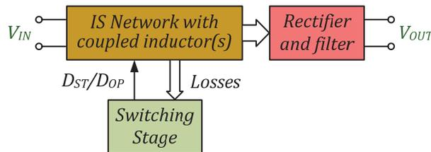
Figure 2.5 Generalized functional scheme of the coupled-inductor-based GI ISCs class.
