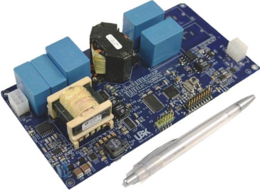
Fig. 4. The 200 W prototype of the PV MIC based on the SSqZSC topology.
