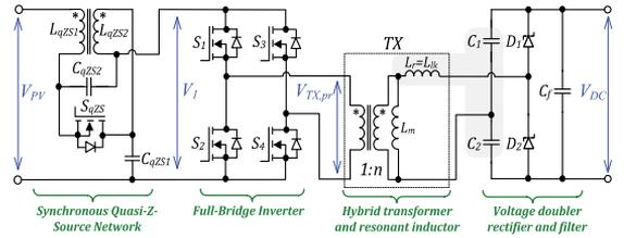
Fig. 3. Generalized topology of the galvanically isolated series resonant quasi-Z-source DC-DC converter (qZSSRC).
