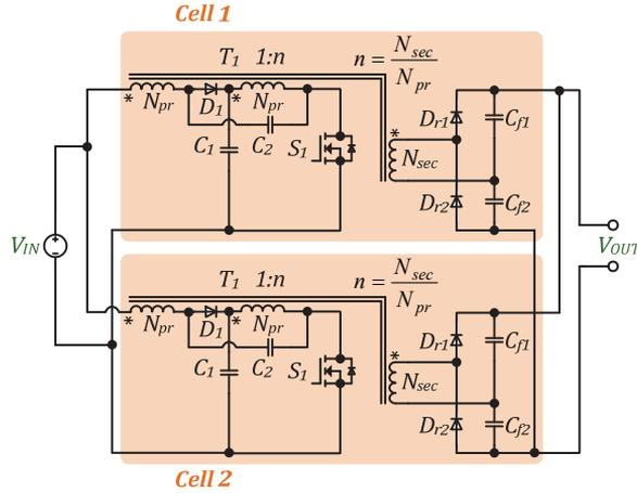
Figure 4.16 Topology of a GI coupled-inductor-based qZS DC-DC converter stage composed of two cells.
