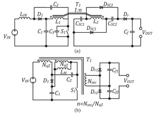
Fig. 25. qZS-based galvanically isolated coupled-inductor-based single-switch dc-dc converters: (a) with two inductors [67] and (b) with a single inductor [68].
