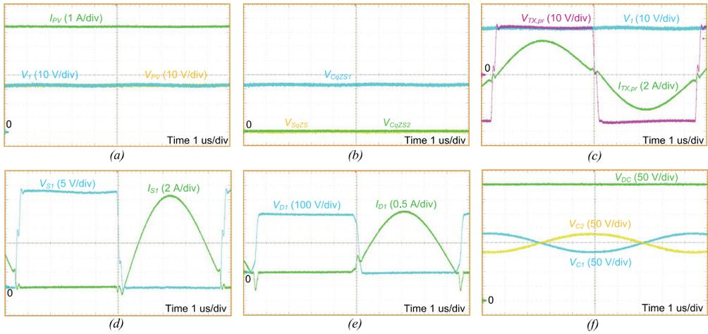
Fig. 23. Experimental waveforms of the qZSSRC in the normal mode at  $V_{PV} = 34$  V and  $P = 250$  W: input voltage, input current, and intermediate DC-link voltage (a), voltages of qZS capacitors and voltage of the switch  $S_{qZS}$  (b), intermediate DC-link voltage and isolation transformer primary winding voltage and current (c), voltage and current of switch  $S_1$  (d), voltage and current of diode  $D_1$  (e), voltages of VDR capacitors and output voltage of the converter (f).
