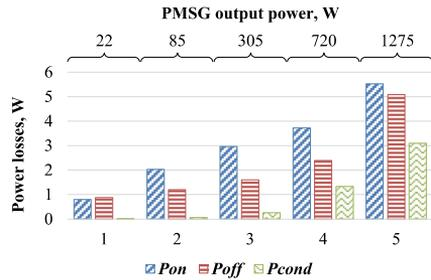
Fig. 15. Semiconductor power losses of a DC-DC converter switch: turn-on ( $P_{on}$ ), turn-off ( $P_{off}$ ), and conducting ( $P_{cond}$ ).
