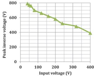
Fig. 9. Peak inverse voltage across diode  $Dr_1$  in the HWR topology versus the input voltage.
