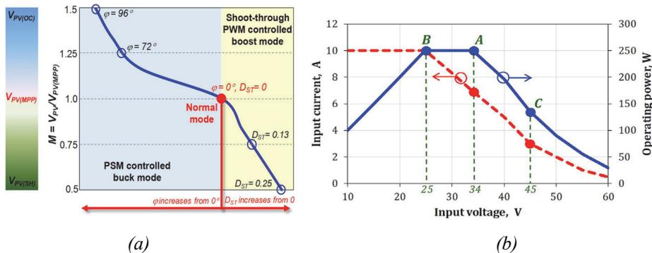
Figure 4.4 Operating modes with ideal control variables (a) and load profile of the qZSSRC (b) [PAPER-IX].
