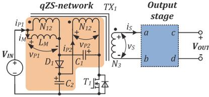
Fig. 2. General schematic of the isolated qZS DC-DC converter.
