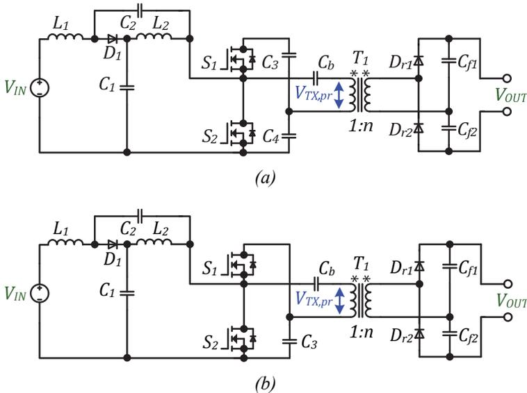
Figure 3.3 Transformer-based qZS GI asymmetrical half-bridge DC-DC converters: with two (a) and a single capacitor (b) in the switching stage [PAPER-II].
