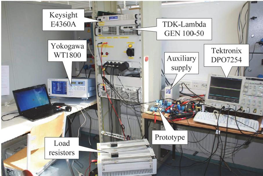
Figure 1.3 Photo of the test-bench used for the experimental study of PV module integrated converters.
