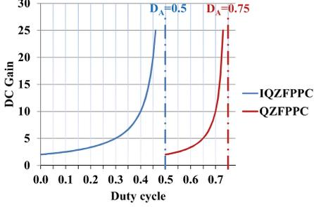
Fig. 6 – DC gain characteristics of the proposed converters.
