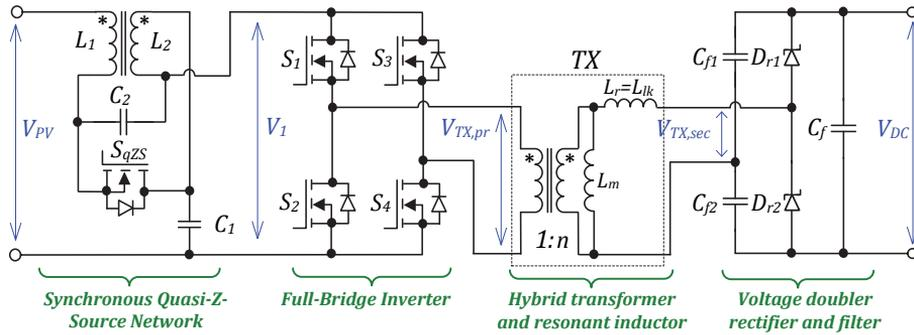
Figure 4.3 Galvanically isolated series resonant full-bridge quasi-Z-source DC-DC converter (qZSSRC) topology.
