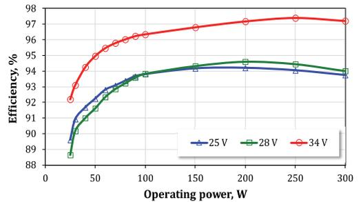
Fig. 22. Experimental efficiency of the proposed converter in the maximum power point range.
