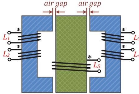
Figure 3.11 Five-winding coupled inductor for the coupled-inductor-based qZS GI push-pull DC-DC converter with a single coupled inductor.
