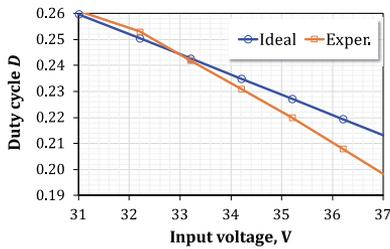
Fig. 6. Comparison of ideal and experimental regulation characteristics of the proposed converter.
