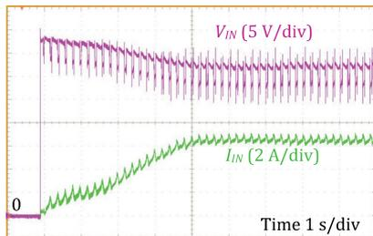
Fig. 7. Input voltage and current during startup and MPPT process.
