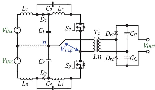
Figure 3.1 Transformer-based qZS GI symmetrical half-bridge DC-DC converter [PAPER-III].
