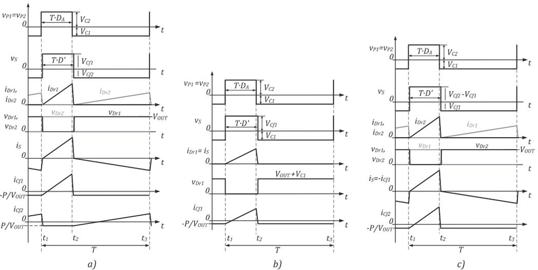
Fig. 5. Idealized waveforms of currents and voltages of the basic converter for the three selected rectifiers: a) VDR1, b) HWR, c) VDR2.
