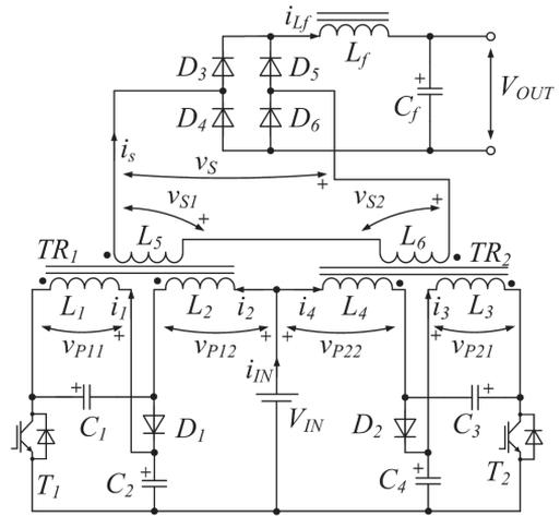
**Figure 1:** qZS-derived push-pull converter topology.
