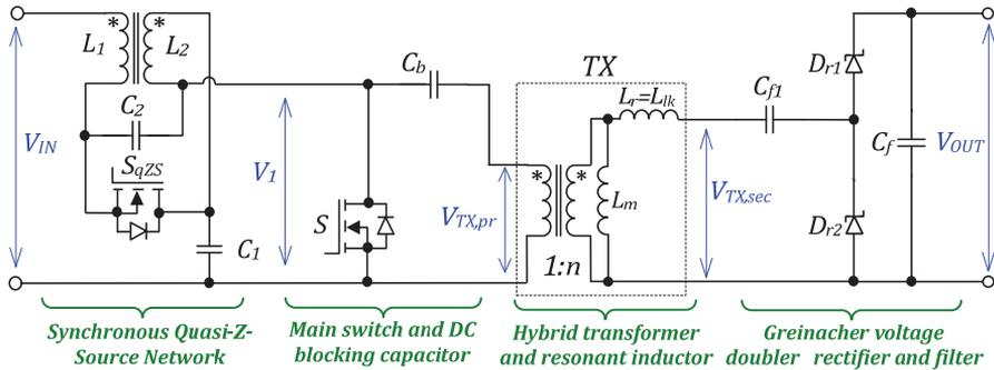
Figure 4.10 Galvanically isolated single-switch qZS MIC topology.
