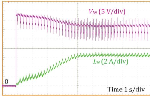
Figure 4.14 Input voltage and current during startup and the MPPT process.
