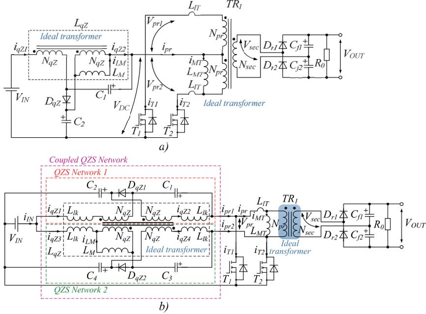
Fig. 2 – Topologies of the proposed quasi-Z-source-fed push-pull converter family: a) quasi-Z-source-fed push-pull converter and b) interleaved quasi-Z-source-fed push-pull converter.
