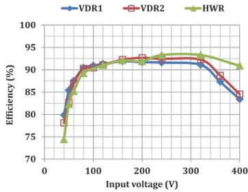
Fig. 8. Measured efficiency versus input voltage.
