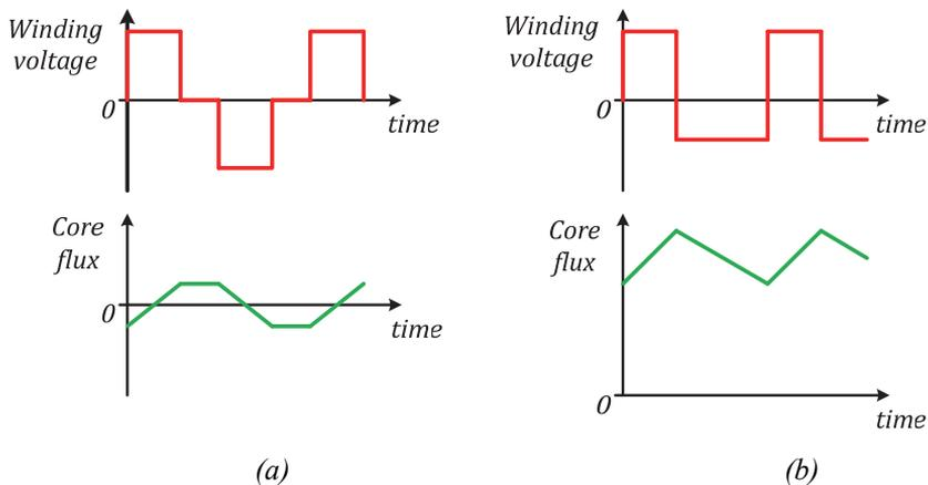
Figure 2.1 Sketches of typical waveshapes of the winding voltage and consequent core flux of: a transformer (a) and a coupled inductor (b) [PAPER-I].
