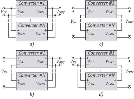
Fig. 1. Four architectures of the series-parallel conversion system: a) IPOP, b) ISOP, c) ISOS, and d) IPOS.
