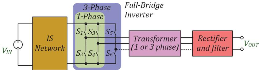
Figure 2.4 Generalized functional scheme of the transformer-based GI ISCs with the full-bridge switching stage [PAPER-I].
