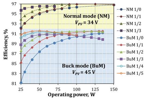
Fig. 26. Part- and light-load efficiency improvement of the proposed converter by the use of the cycle-skipping technique.
