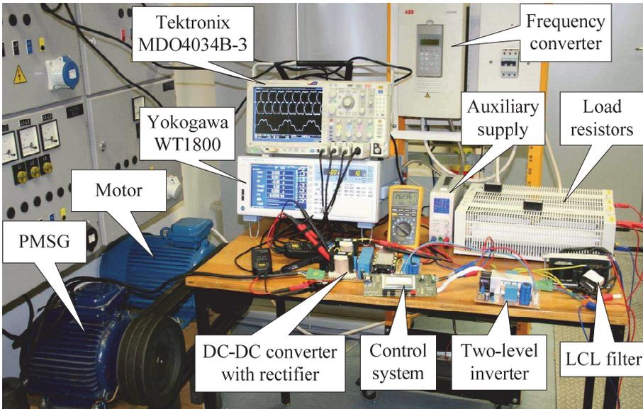
Figure 1.4 Photo of the test-bench used for the experimental study of the power conditioning unit intended for variable speed permanent magnet synchronous generator (PMSG) based micro wind turbines.
