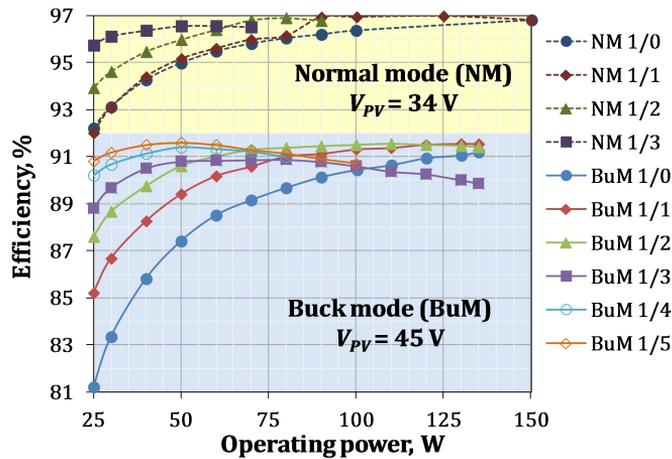
Figure 4.9 Light-load efficiency of the  $qZSSRC$  for different cycle-skipping modulation parameters (1/0 - no cycle skipping, 1/1 - one applied and one skipped, etc.) [PAPER-IX].
