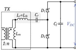
Fig. 4. Greinacher voltage doubler rectifier as an alternative option for the qZSSRC secondary side.
