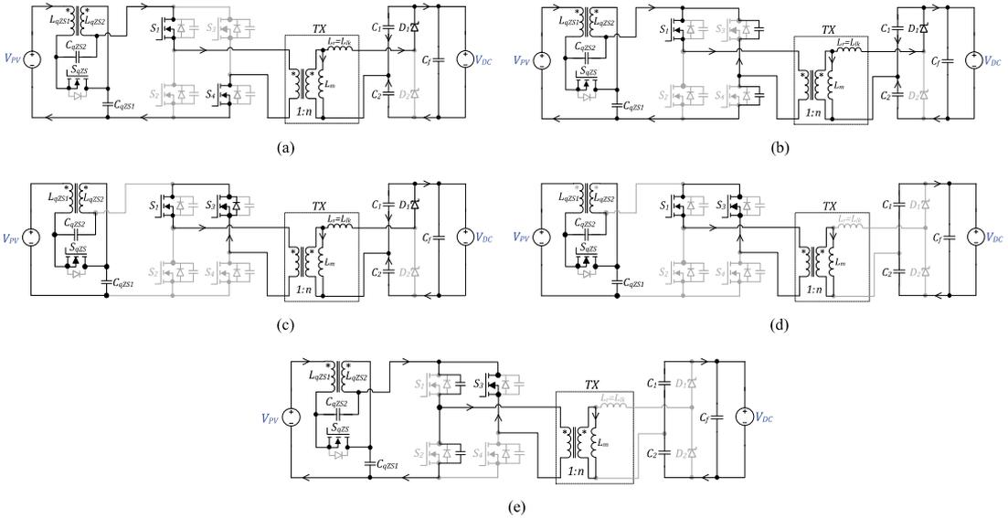
Fig. 9. Generalized equivalent circuits of the qZSSRC operating in the buck mode:  $t_0 < t < t_1$  (a),  $t_1 < t < t_2$  (b),  $t_2 < t < t_3$  (c),  $t_3 < t < t_4$  (d) and  $t_4 < t < t_5$  (e).
