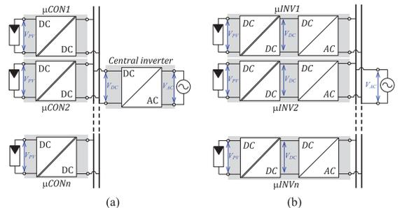
Fig. 1. Full-power converters for the parallel connection of PV modules: microconverters ( $\mu CON$ ) with common DC bus (a) and microinverters ( $\mu INV$ ) with grid side connection (b).
