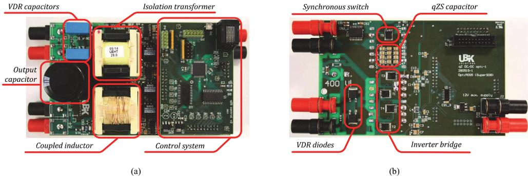
Fig. 18. Top (a) and bottom (b) views of the 300 W experimental prototype of the wide input voltage range PV microconverter based on the qZSSRC topology.
