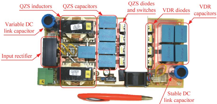
Figure 4.17 Prototype of the two-cell GI qZS DC-DC converter.
