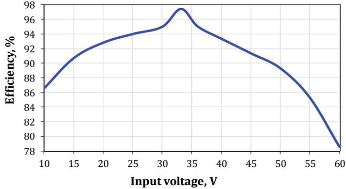
Figure 4.8 Experimental efficiency of the converter  $qZSSRC$  according to the power profile from Figure 4.4 [PAPER-IX].
