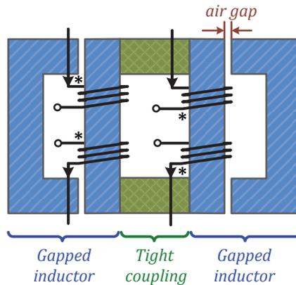
Figure 3.6 Four-winding coupled inductor for an interleaved qZS push-pull converter.
