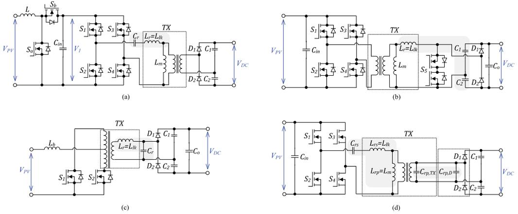
Fig. 2. State-of-the-art DC-DC converters for MLPE applications: double stage topology combined from a front-end synchronous boost converter and series resonant converter (a), double stage topology combined from a series resonant converter and a back-end boost converter based on the bi-directional AC switch (b), single stage approach based on the parallel resonant current-fed push-pull converter (c), and single-stage multiresonant converter (d).
