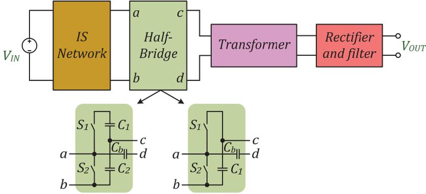
Figure 3.4 Generalized functional scheme of the transformer-based asymmetrical half-bridge GI ISCs [PAPER-I].
