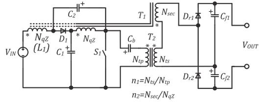
Fig. 5. Single-switch galvanically isolated qZS DC-DC converter with combined energy transfer
