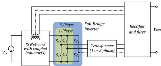
Fig. 1. Generalized functional scheme of the galvanically isolated full-bridge IS DC-DC converter with combined energy transfer.
