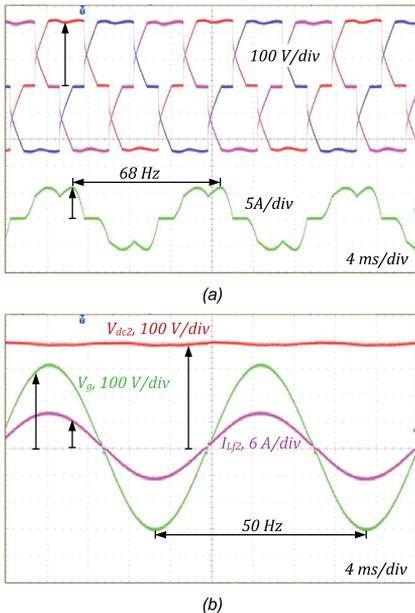
Fig. 13. Experimental voltage and current waveforms: generator output line-to-line voltages (top) and phase current (bottom) (a) and the stable DC link voltage (top) and inverter current and voltage (bottom) (b).
