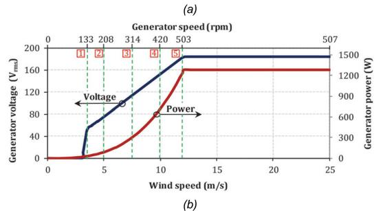
Fig. 11. Characteristics of the case study variable speed PMSG based WT: optimum torque curve (a) and dependence of the PMSG line-to-line voltage and output power on the wind speed.
