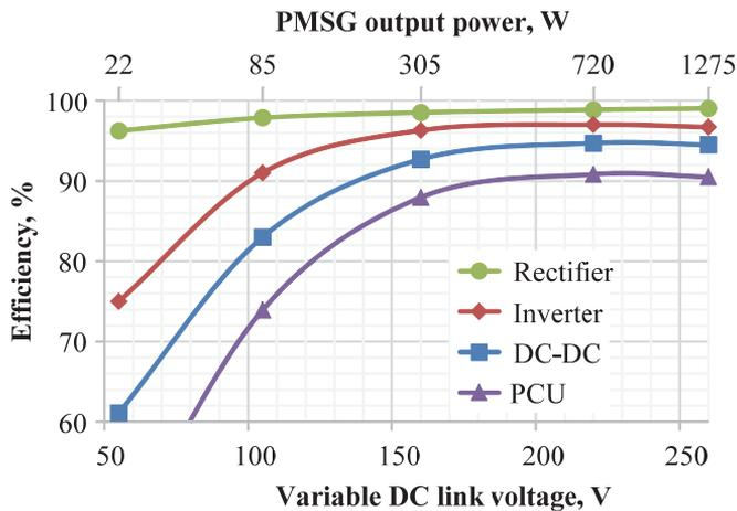
Figure 4.20 Efficiency measurement of the PCU and its parts.
