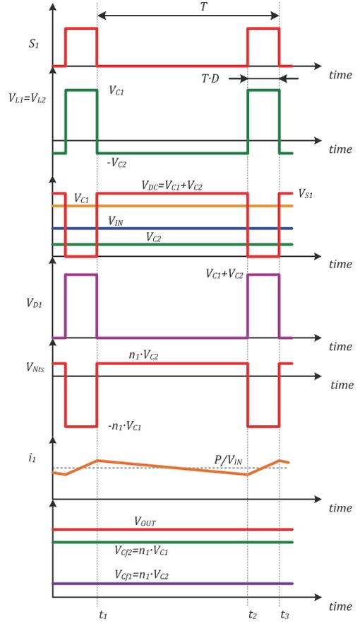
Fig. 4. Idealized current and voltage waveforms of the proposed converter
