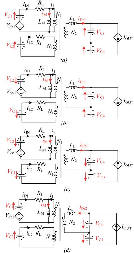
Fig. 4. Equivalent circuits of the single-switch qZS dc-dc converter.
