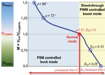
Fig. 5. An example of operating modes and idealized control variables of the multi-mode qZSSRC.
