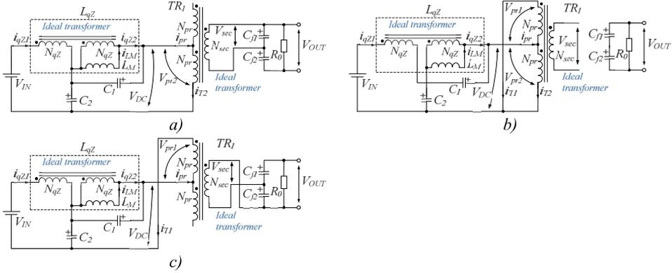
Fig. 4 – Equivalent circuits of the QZSFPPC for time intervals: a)  $[t_1; t_2]$ , b)  $[t_2; t_3]$  and  $[t_4; t_5]$ , c)  $[t_3; t_4]$ .
