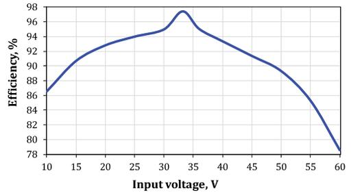
Fig. 21. Experimental efficiency of the proposed converter measured according to the power profile from Fig. 17.
