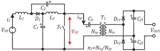
Fig. 3. Single-switch galvanically isolated qZS DC-DC converter
