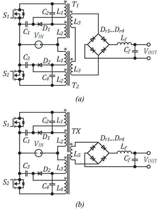
Figure 3.10 Coupled-inductor-based qZS GI push-pull DC-DC converters with an ISN that contains two (a) and one (b) coupled inductor [51].
