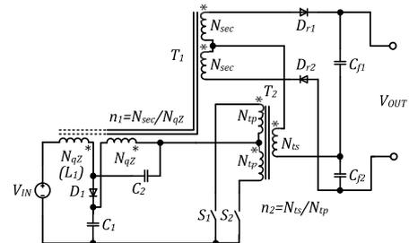
Fig. 4. qZS based galvanically isolated push-pull DC-DC converter with combined energy transfer.
