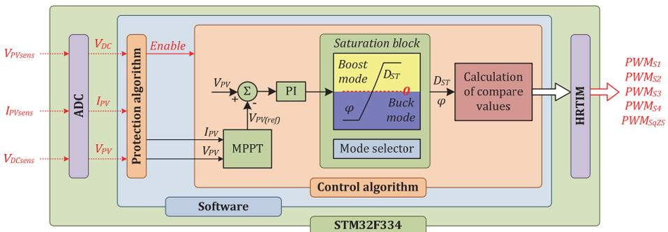
Figure 4.6 Block diagram of the control system developed for the qZSSRC converter [PAPER-IX].
