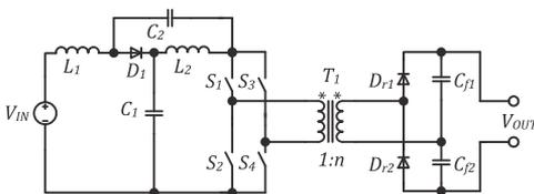
Fig. 1. qZS based galvanically isolated full-bridge DC-DC converter
