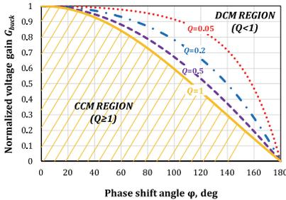
Fig. 11. Normalized voltage gain of the qZSSRC as a function of the phase shift angle  $\varphi$  for the different  $Q$ -factors of the resonant network.
