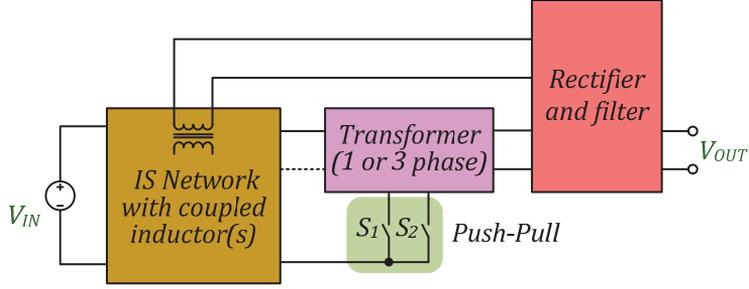
Figure 3.17 Generalized functional scheme of the push-pull GI ISCs with combined energy transfer [PAPER-I].
