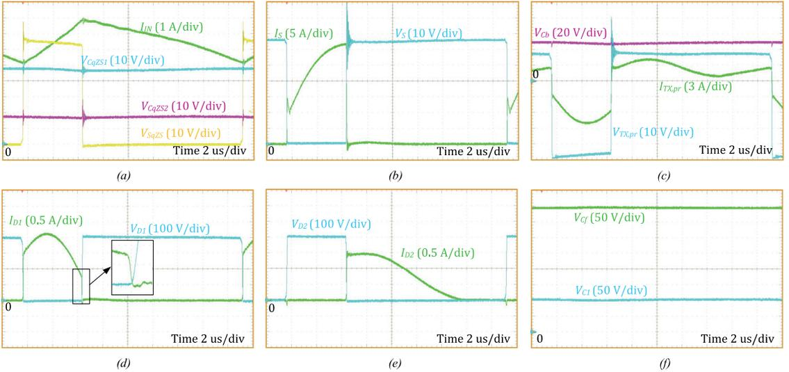
Fig. 5. Experimental waveforms of the proposed converter at  $V_{IN} = 31$  V,  $P = 200$  W,  $D = 0.26$  and  $V_{OUT} = 400$  V: input current, voltages of qZS capacitors and voltage of the switch  $S_{qZS}$  (a), voltage and current of main switch  $S$  (b), voltage of DC blocking capacitor and isolation transformer primary winding voltage and current (c), voltage and current of diode  $D_1$  (d), voltage and current of diode  $D_2$  (e), voltages of GVDR capacitors (g).
