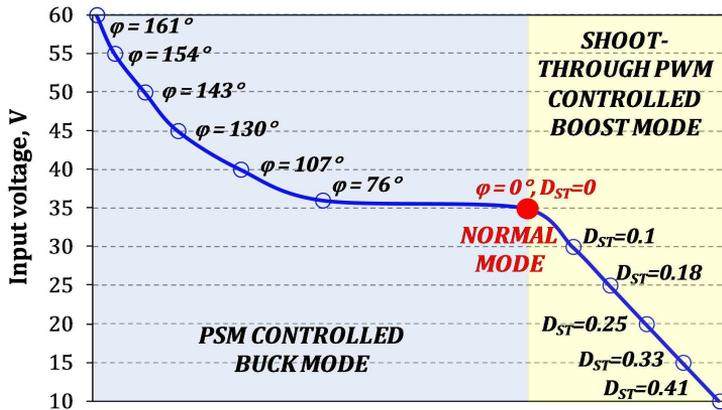
Figure 4.7 Experimental control variables of the qZSSRC converter [PAPER-IX].
