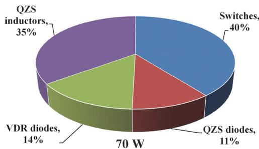
Figure 4.21 Power loss breakdown on the DC-DC converter at the maximum power (operating point 5).
