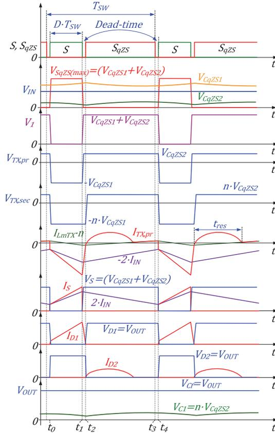
Figure 4.11 Sketch of the idealized current and voltage waveforms of the transformer-based single-switch qZS DC-DC converter [PAPER-X].
