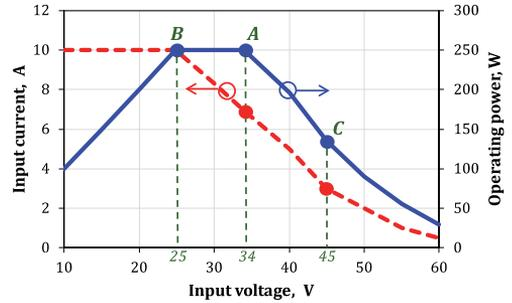
Fig. 17. Input current and operating power of the experimental prototype as functions of the input voltage.
