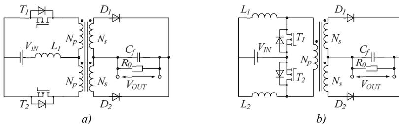
Fig. 1 – Isolated current-fed push-pull converter family: a) current-fed push-pull converter and b) two-inductor isolated boost converter.
