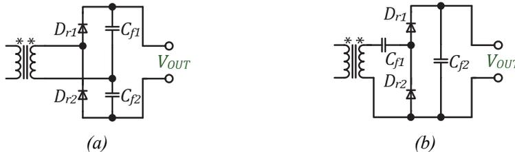
Figure 3.20 Voltage doubler rectifiers: bridge type (a) and Greinacher type (b) [5].
