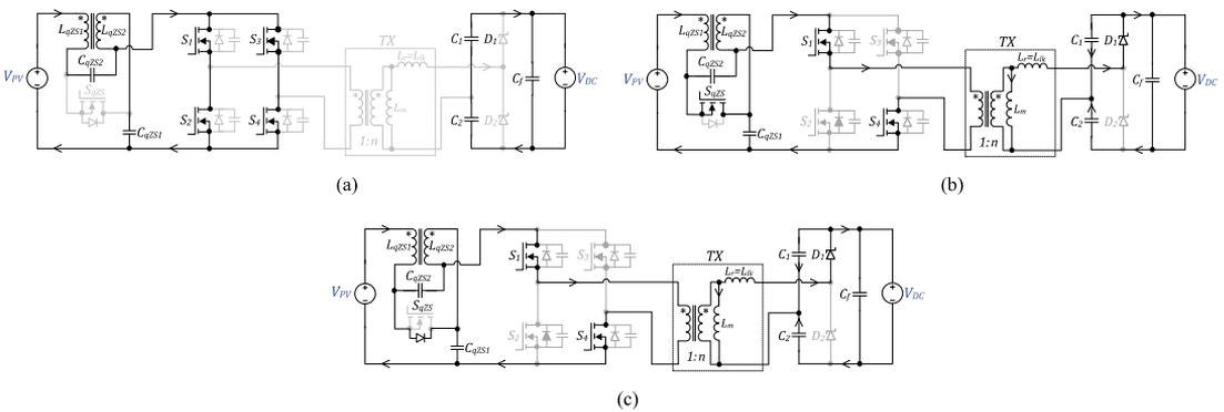
Fig. 10. Generalized equivalent circuits of the qZSSRC operating in the boost mode:  $t_0 < t < t_1$  (a),  $t_1 < t < t_2$  (b) and during the dead-time of the  $S_{qzS}$  (c).
