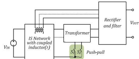
Fig. 3. Generalized functional schemes of the galvanically isolated IS push-pull DC-DC converter with combined energy transfer.
