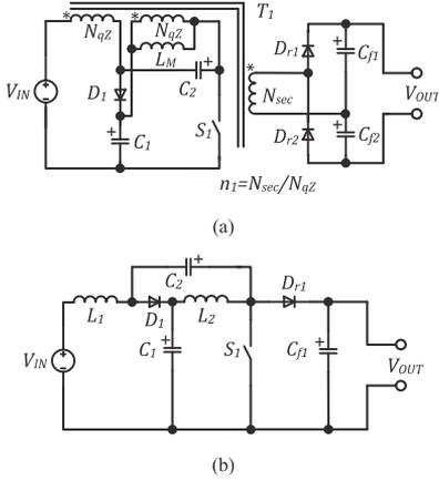
Fig. 2. qZS single-switch DC-DC converters: galvanically isolated coupled inductor based with a single inductor (a) and conventional nonisolated (b).
