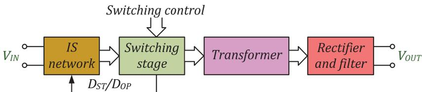
Figure 2.2 Generalized functional scheme of the transformer-based GI ISCs class.
