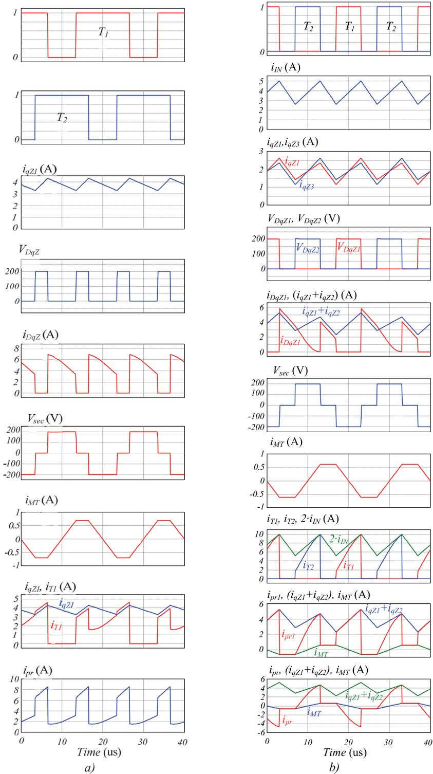
Fig. 7 – Simulation results of the proposed converters: a) QZSFPPC and b) IQZSFPPC.
