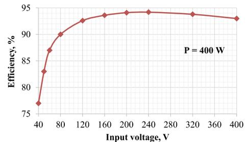
Fig. 7. Efficiency measured at the constant operating power.
