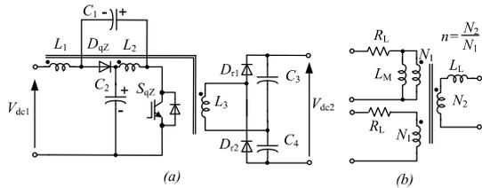
Fig. 2. Investigated topology of the single-switch isolated qZS based dc-dc converter (a) and equivalent circuit of coupled inductor (b).
