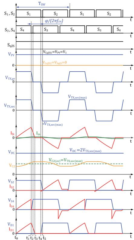
Fig. 7. Steady-state waveforms of the qZSSRC operating in the buck mode.
