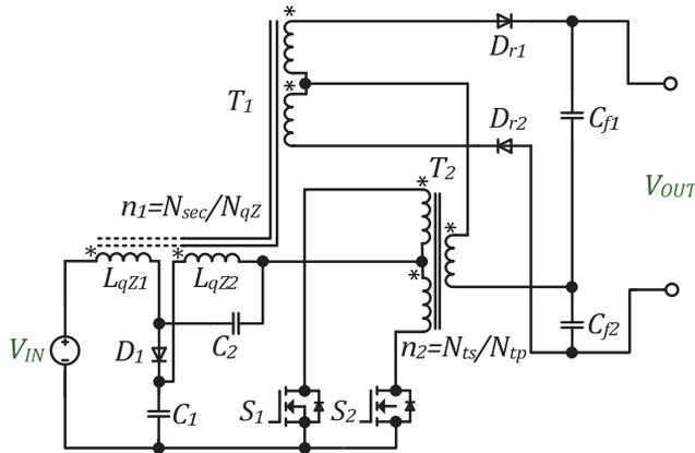
Figure 3.16 qZS GI push-pull DC-DC converters with combined energy transfer [PAPER-IV].
