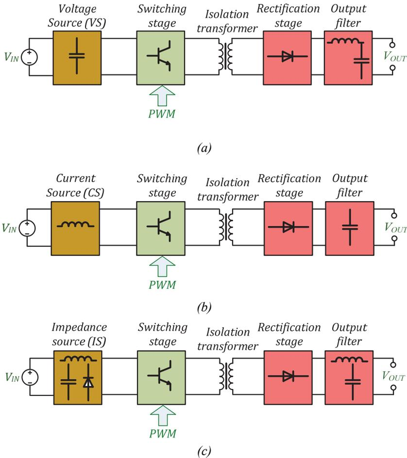
Figure 1.1 Generalized block diagrams of the VS (a), CS (b) and IS (c) GI DC-DC converters [PAPER-I].
