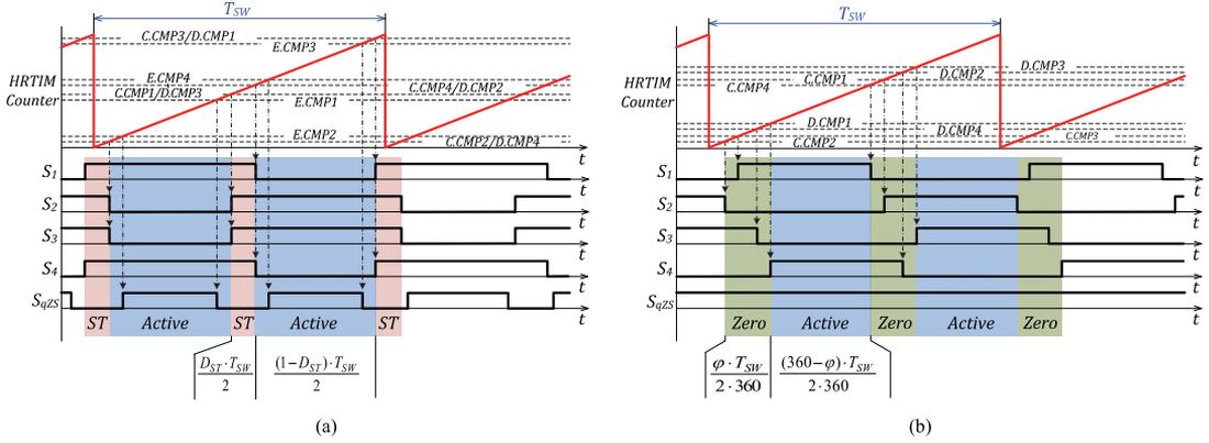
Fig. 16. Generalized principle of the control signal generation in the boost (a) and the buck (b) modes.
