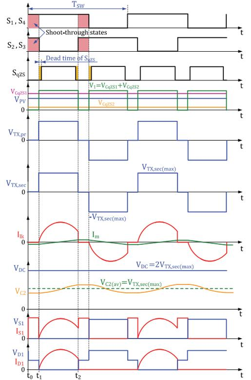
Fig. 12. Steady-state waveforms of the qZSSRC operating in the boost mode.
