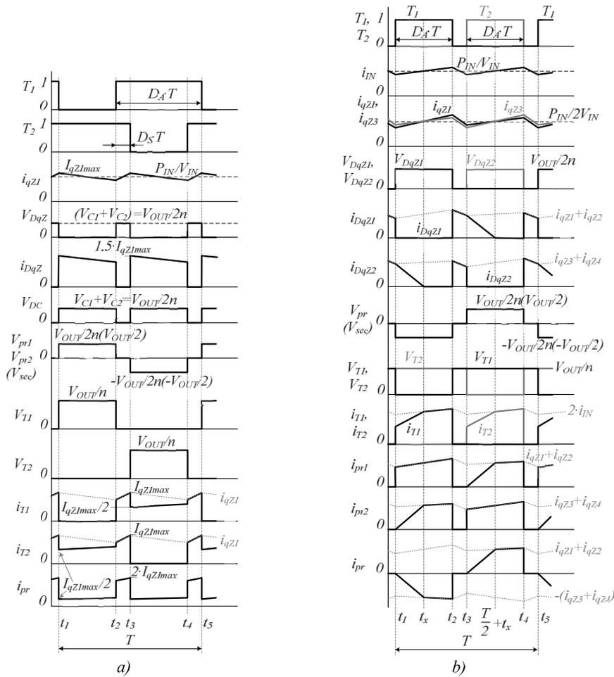
Fig. 3 – Current and voltage waveforms for the proposed converters: a) QZSFPPC and b) IQZSFPPC.
