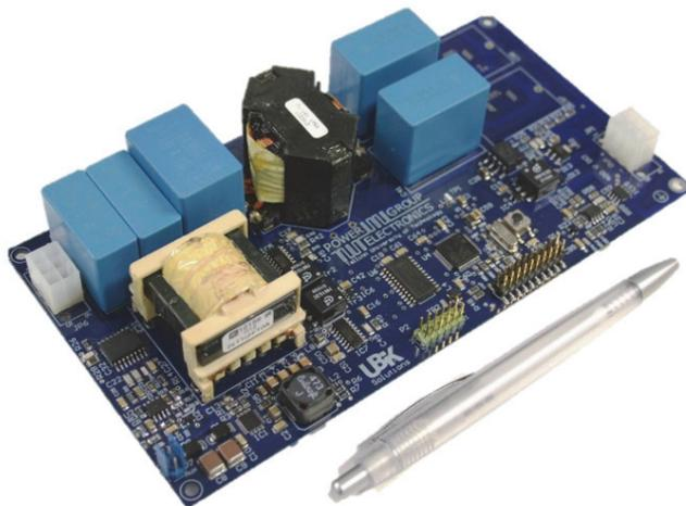
Figure 4.12 Developed 250 W prototype of the single-switch qZS MIC [PAPER-X].
