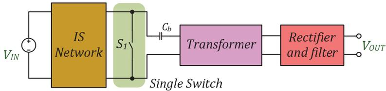
Figure 3.9 Generalized functional scheme of the transformer-based single-switch GISCs [PAPER-I].
