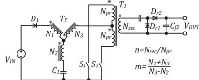
Fig. 19. YS-based galvanically isolated push-pull dc-dc converter [62].
