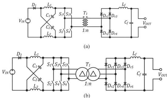
Fig. 5. State-of-the-art (a) ZSI-based single-phase and (b) three-phase galvanically isolated dc–dc converters [13], [21].
