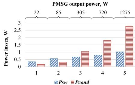
Fig. 16. Semiconductor power losses of a dc-dc converter qZS diode: switching ( $P_{sw}$ ) and conducting ( $P_{cond}$ ).
