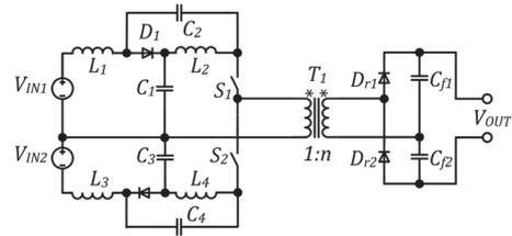
Fig. 14. qZS-based galvanically isolated symmetrical half-bridge dc–dc converter [58].
