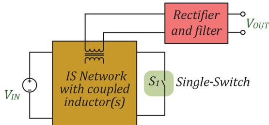
Figure 2.7 Generalized functional scheme of the coupled-inductor-based GI ISCs with a single switch [PAPER-I].
