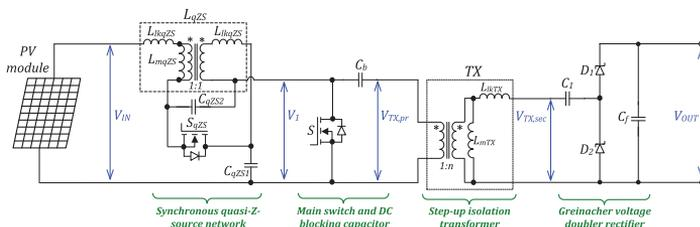
Fig. 1. Generalized circuit structure of the proposed single-switch galvanically isolated step-up DC-DC converter for photovoltaic applications.
