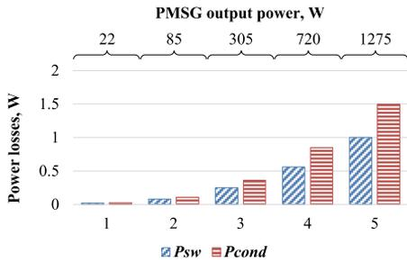
Fig. 17. Semiconductor power losses of a dc-dc converter VDR diode: switching ( $P_{sw}$ ) and conducting ( $P_{cond}$ ).
