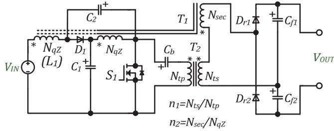
Figure 3.18 qZS GI single-switch DC-DC converters with combined energy transfer [PAPER-IV].
