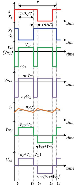
Fig. 6. Control principle and idealized operating waveforms of the proposed topology.
