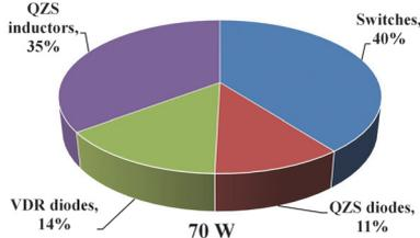
Fig. 18. Power loss breakdown on the dc-dc converter at maximum power (operating point 5).
