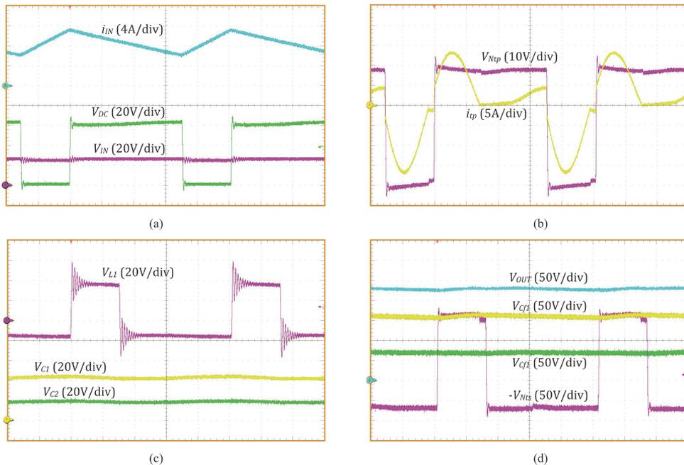
Fig. 7. Experimental waveforms of the proposed topology: input voltage, input current and intermediate DC-link voltage (a), voltage and current of the transformer primary winding (b), voltage of the qZS inductor, and qZS capacitors (c), and voltage of the transformer secondary winding, voltages of the VDR capacitors and output voltage of the converter (d) in time scale 2  $\mu$ s/div.
