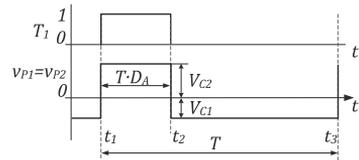
Fig. 4. Idealized waveforms of the primary windings voltage.
