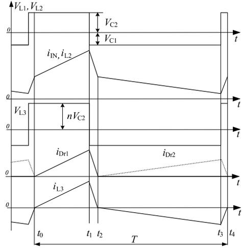
Fig. 3. Idealized waveforms of the proposed isolated single-switch dc-dc converter.
