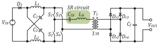
Fig. 9. ZS-based galvanically isolated SR full-bridge dc-dc converter [24].
