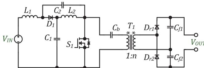
Figure 3.8 Transformer-based qZS GI single-switch DC-DC converter [PAPER-V].
