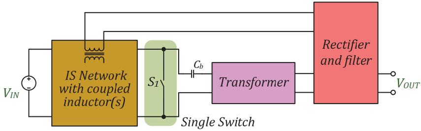
Figure 3.19 Generalized functional scheme of the single-switch GI ISCs with combined energy transfer [PAPER-I].
