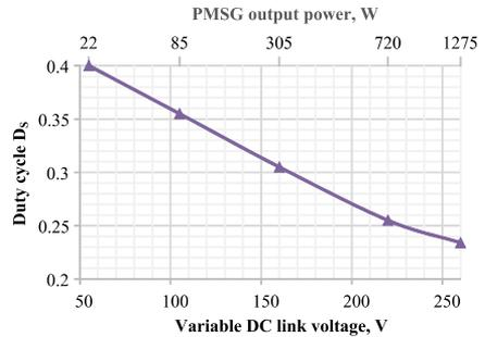
Fig. 14. Duty cycle of the DC-DC converter switches.
