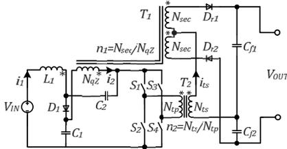
Fig. 5. Power circuit layout of the qZS galvanically isolated single-phase full-bridge ISC with combined energy transfer.
