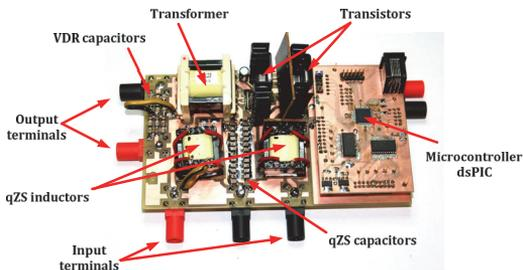
Fig. 5. Experimental prototype (165 mm x 90 mm).
