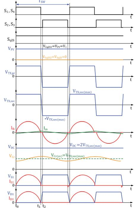
Fig. 6. Steady-state waveforms of the qZSSRC operating in the normal mode.
