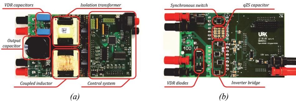
Figure 4.5 Top (a) and bottom (b) views of the 300 W MIC prototype of the qZSSRC [PAPER-IX].
