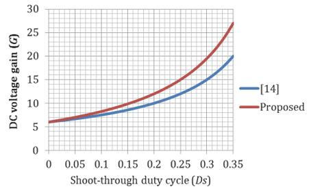
Fig. 8. Comparison of DC voltage gain for  $n_1 = 3$  and  $n_2 = 3$ .
