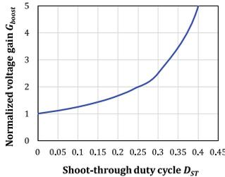
Fig. 13. Normalized voltage gain of the qZSSRC in a boost mode.
