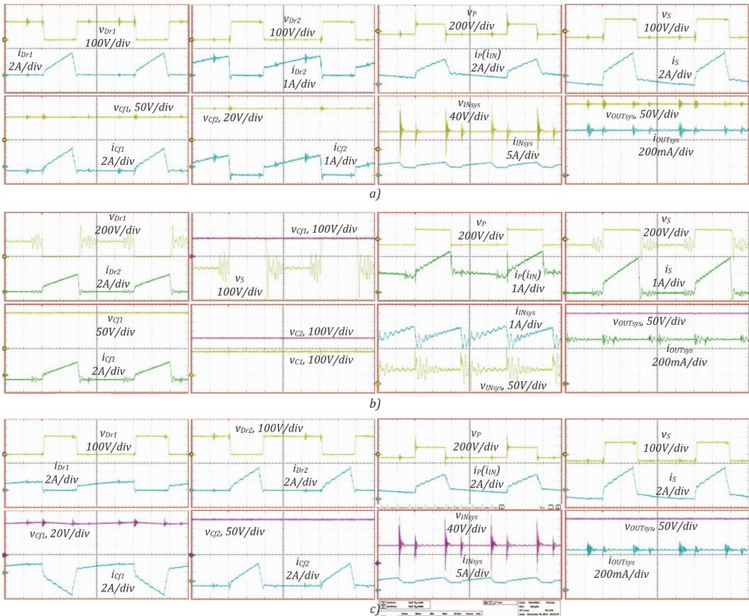
Fig. 10. Experimental waveforms of voltages and currents in the converter with: a) VDR1, b) HWR, and c) VDR2 rectifiers, in time scale  $2 \mu\text{s}/\text{div}$ .
