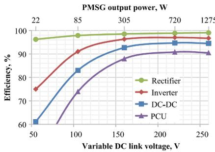
Fig. 12. Efficiency measurement of the PCU and its parts.
