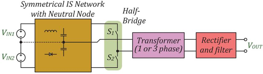
Figure 3.2 Generalized functional scheme of the transformer-based symmetrical half-bridge GI ISCs [PAPER-I].
