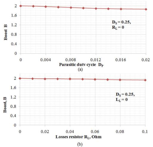
Fig. 5. The boost factor as a function of the  $D_P$  (a) and  $R_L$  (b).
