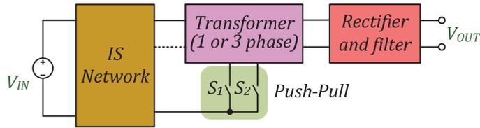
Figure 3.7 Generalized functional scheme of the transformer-based push-pull GI ISCs [PAPER-I].
