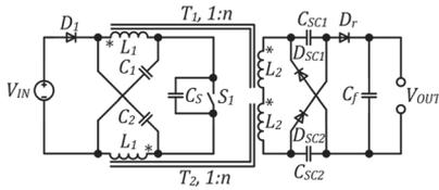
Fig. 26. ZS-based galvanically isolated single-switch dc–dc converter [69].
