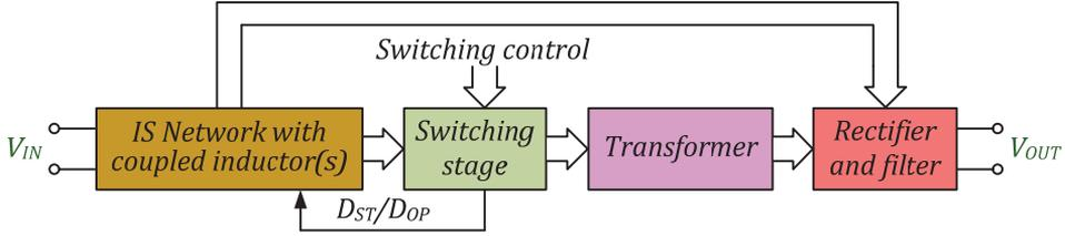
Figure 3.13 Generalized functional scheme of the class of GI ISCs with combined energy transfer.
