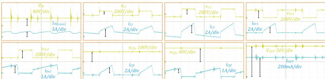
Fig. 9. Experimental voltage and current waveforms in time scale of 2  $\mu$ s/div.
