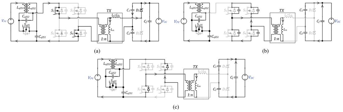
Fig. 8. Generalized equivalent circuits of the qZSSRC operating in the normal mode:  $t_0 < t < t_1$  (a),  $t_1 < t < t_2$  (b), and directly before the instant  $t_2$  (c).
