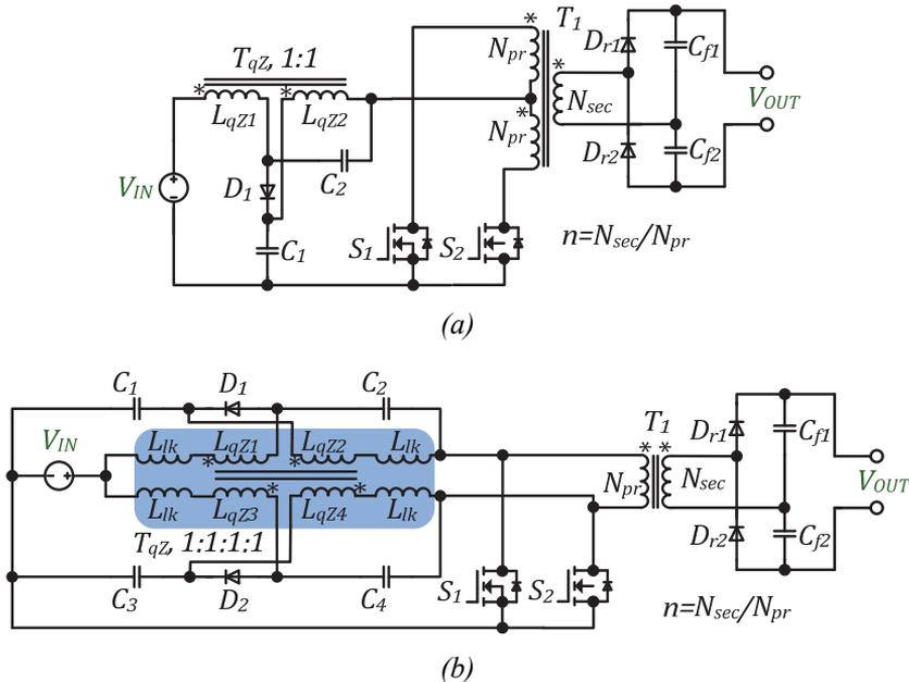
Figure 3.5 Transformer-based qZS GI push-pull DC-DC converters with: ISN that contains a coupled inductor (a) and interleaved with a coupled ISN (b) [PAPER-VII].
