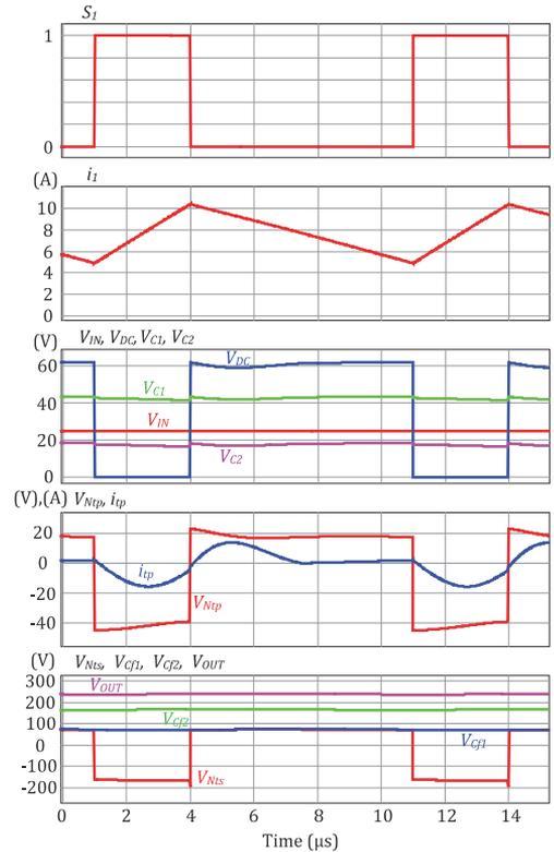
Fig. 6. Simulation results of the proposed topology
