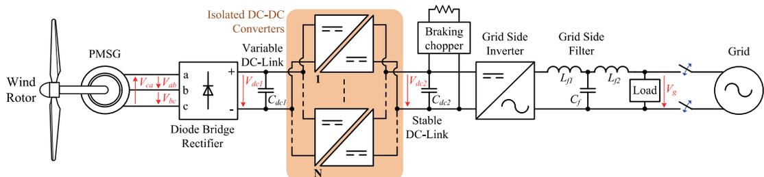
Fig. 1. Proposed variable speed PMSG based wind energy conversion system with three-stage PCU based on the isolated DC-DC converter(s).
