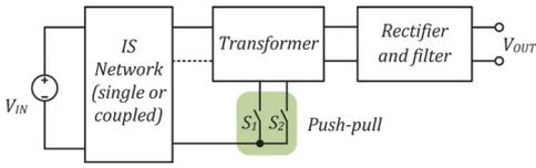
Fig. 16. Generalized functional scheme of the transformer-based IS galvanically isolated dc-dc converters with the push-pull switching stage.
