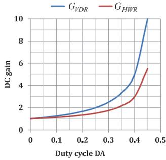
Fig. 6. Ideal DC gain factors of the converter.
