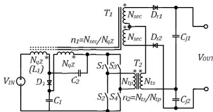
Fig. 2. qZS based galvanically isolated full-bridge DC-DC converter with combined energy transfer.
