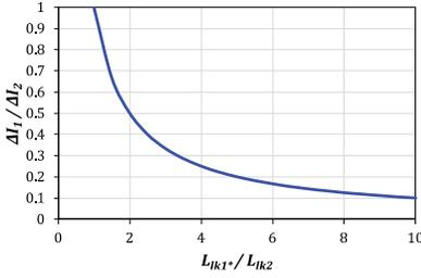
Fig. 15. Current ripple ratio as a function of the leakage inductance ratio.
