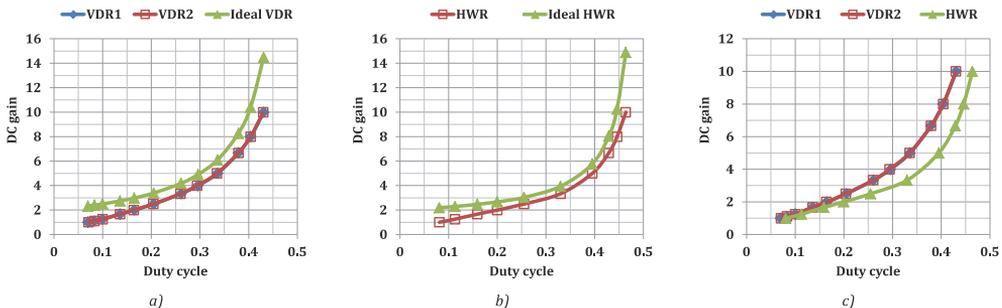
Fig. 7. DC gain characteristics: a) VDR1, VDR2 measured and ideal, b) HWR measured and ideal, c) measured for for all the three topologies.
