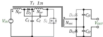
Figure 2.6 Coupled-inductor-based qZS GI single-switch DC-DC converter [PAPER-VIII]: topology (a), sketch of idealized operating waveforms (b), equivalent circuit for the shoot-through state (c), and for the active states (d).
