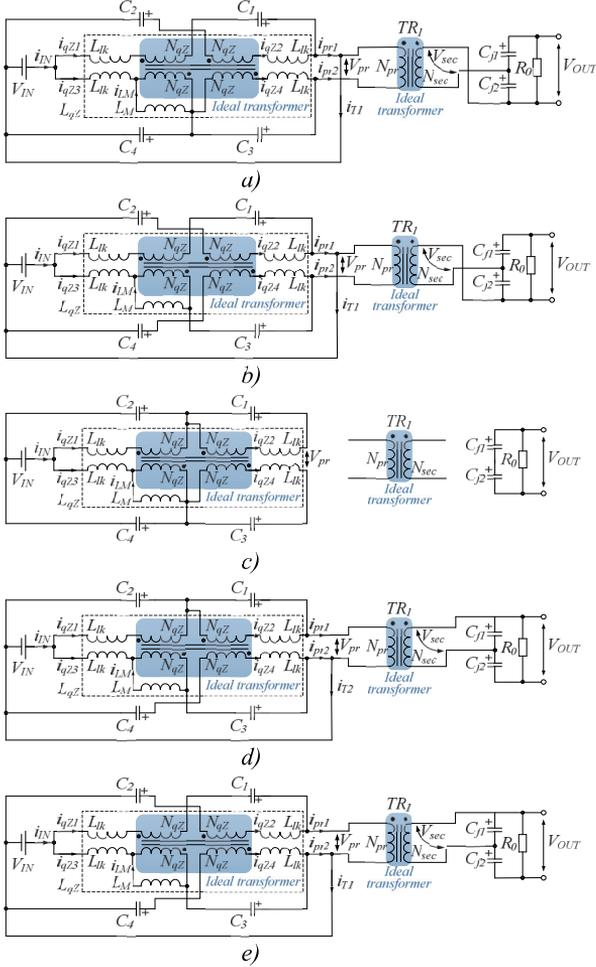
Fig. 5 – Equivalent circuits of the IQZSFPPC for time the intervals: a)  $[t_1; t_x]$ , b)  $[t_x; t_2]$ , c)  $[t_2; t_3]$  and  $[t_4; t_5]$ , c)  $[t_3; T/2 + t_x]$ , d)  $[T/2 + t_x; t_4]$ .
