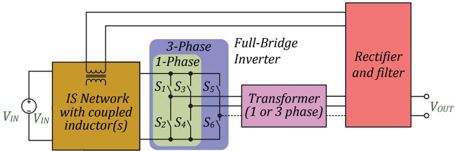
Figure 3.15 Generalized functional scheme of the full-bridge GI ISCs with combined energy transfer [PAPER-I].
