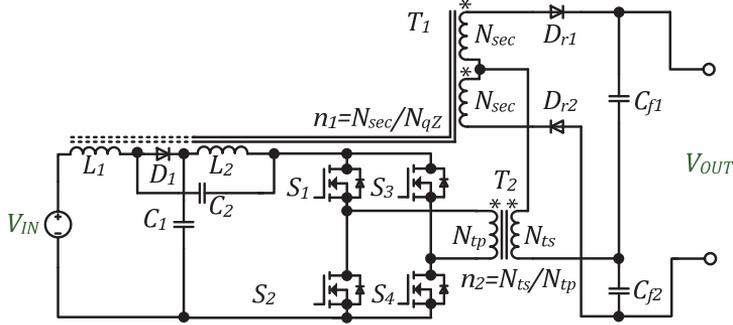
Figure 3.14 qZS GI full-bridge DC-DC converters with combined energy transfer [PAPER-IV].
