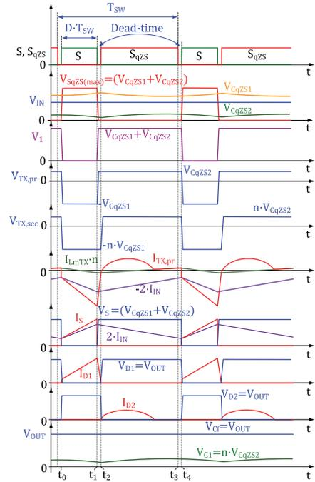
Fig. 2. Idealized steady-state current and voltage waveforms of the SSqZSC with synchronous qZS-network.
