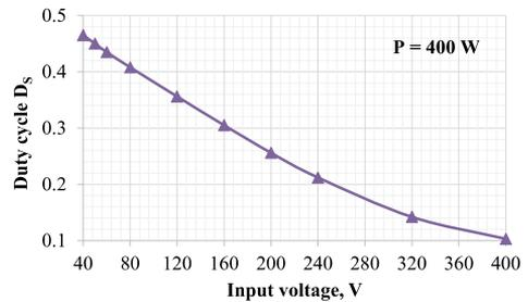
Fig. 8. Duty cycle of the switches at the constant operating power.
