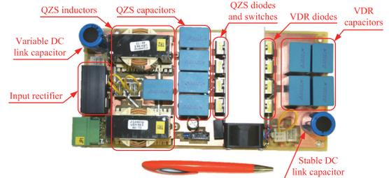
Fig. 6. Developed 1.3 kW prototype composed of two qZS converters.
