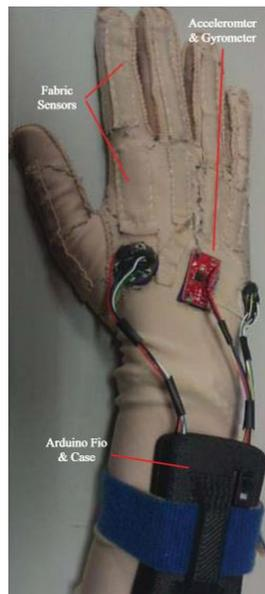
Figure 11. Prototype of Glove made by Research Centre Dublin.
