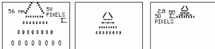
Fig. 15. CCD camera resolution with varying focal length
