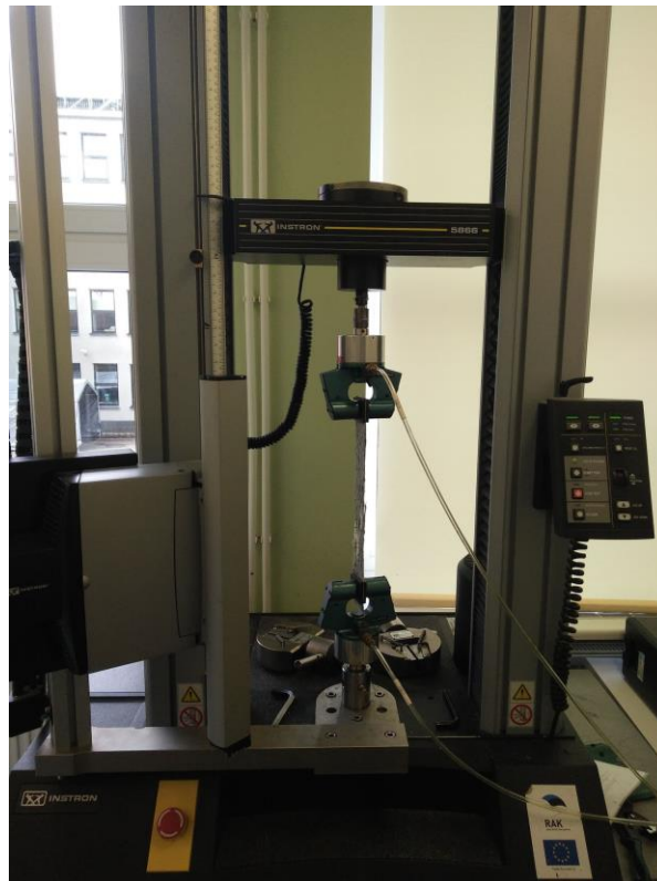
Figure 6.16 Instron 5866 tensile testing machine.
