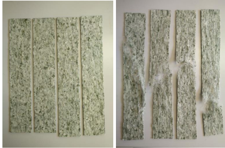
Figure 6.17 Test specimen before and after tensile testing.
