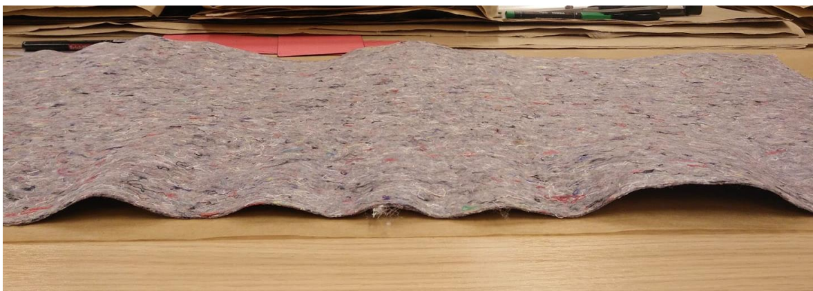
Figure 7.13 Ripple effect on nonwoven material.
