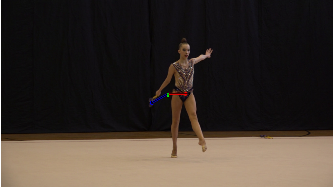
Figure 28. Visualization of the values predicted by the neural network. Red arrow: predicted pan value, blue arrow: predicted zoom value, green arrow: predicted tilt value, black arrows: smoothed values.
