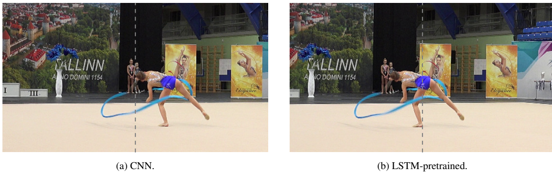
Figure 27. Same frame taken from CNN and LSTM-pretrained simulations. The gymnast is moving from left to right. LSTM manages to keep the gymnast centered even though the gymnast is moving fast and the system has latency. CNN noticeably lags behind and the video looks less eye pleasing because of negative lead room. The gray line is added for illustration purposes and indicates the center of the image.
