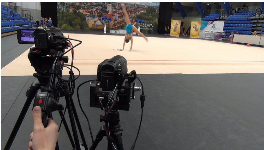
Figure 20. A manually operated camera (left) and a PTZ system operated by CNNs (right).
