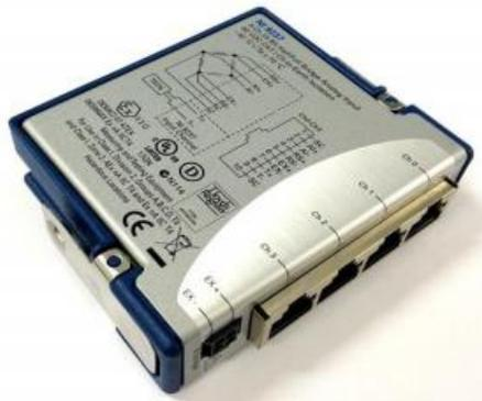
Figure 6.9 NI 9237 DAQ Board [34]
