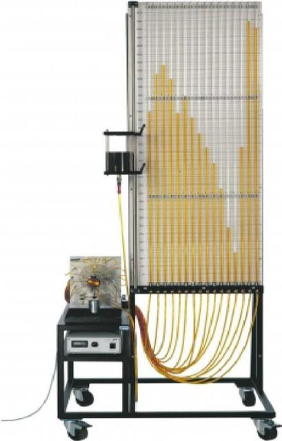
Figure 4.1 Journal bearing apparatus, Gunt Hamburg [9]
