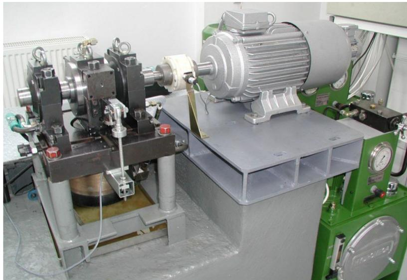
Figure 4.2 PG-2 1Ł - test rig for journal bearings [10]
