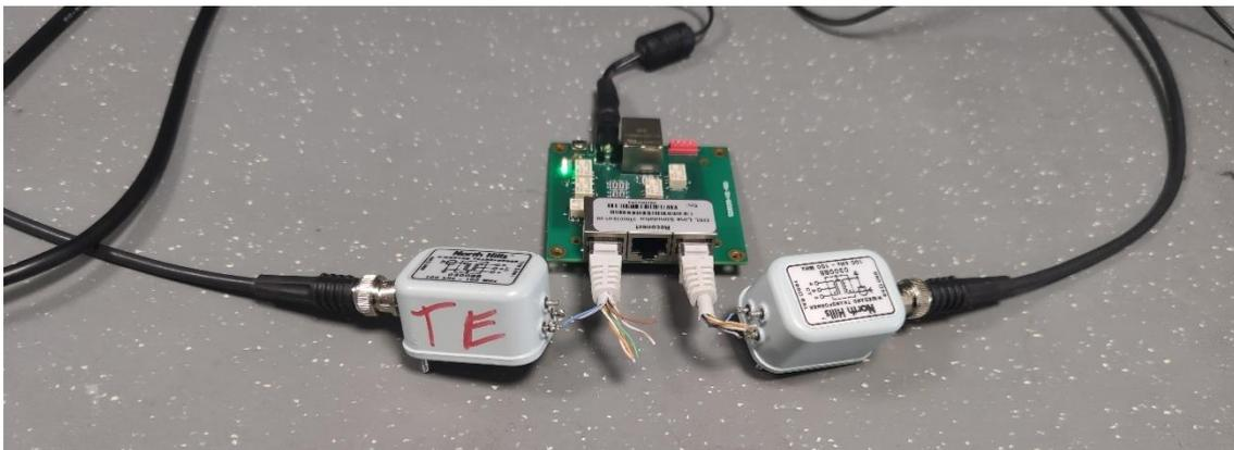
Figure 31 Measurement setup for DSL simulator
