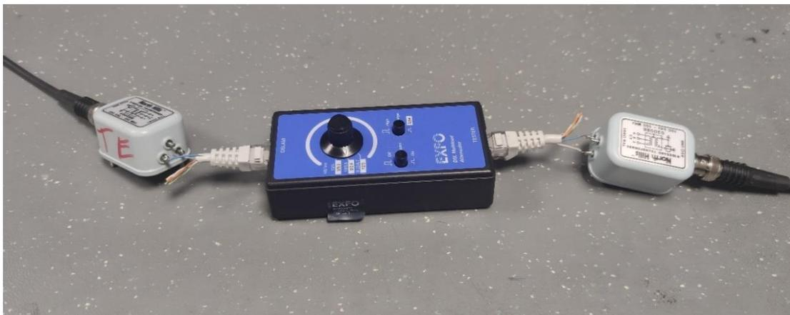
Figure 12 Measurement setup for EXFO device
