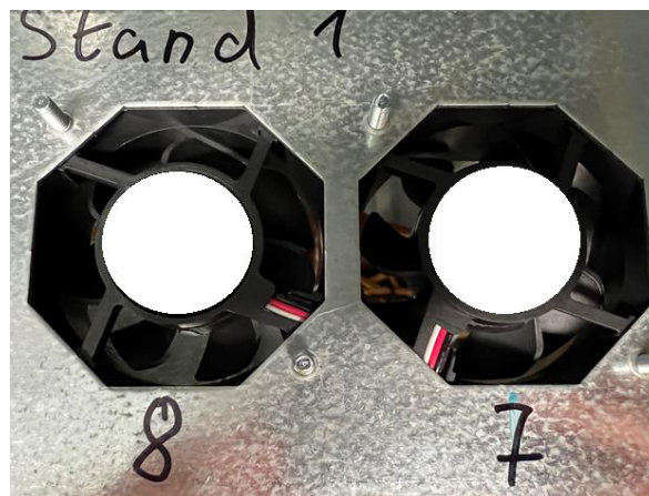
Figure 14. Fans installed on the test jig.
