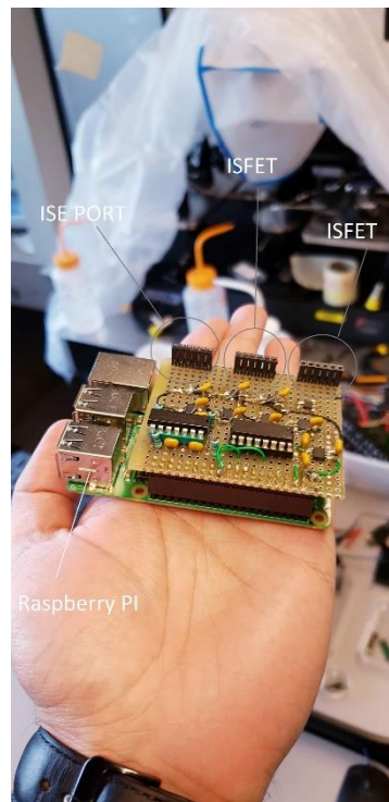
Figure 3: Raspberry Pi with the Developed Circuit
