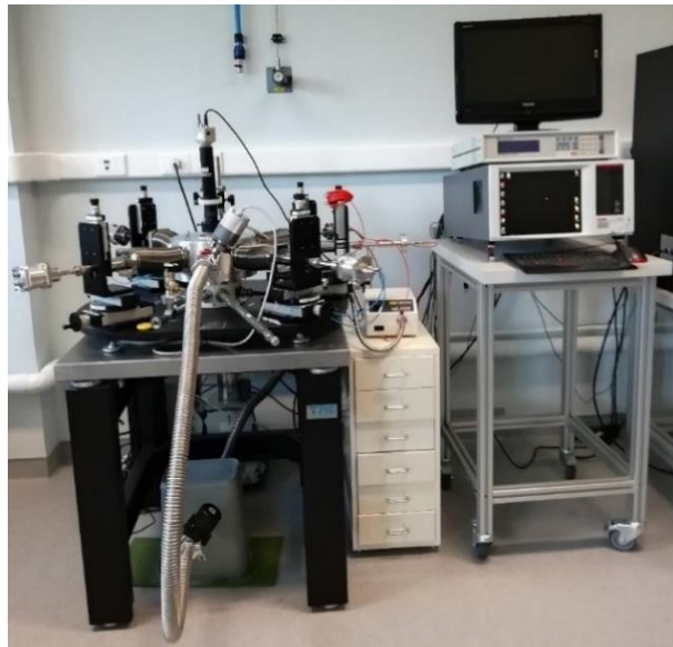
Figure 2. A probe measurement setup including Keithley 4200 SCS semiconductor parameter analyzer and a Janis ST-500 cryogenic probe station [4].
