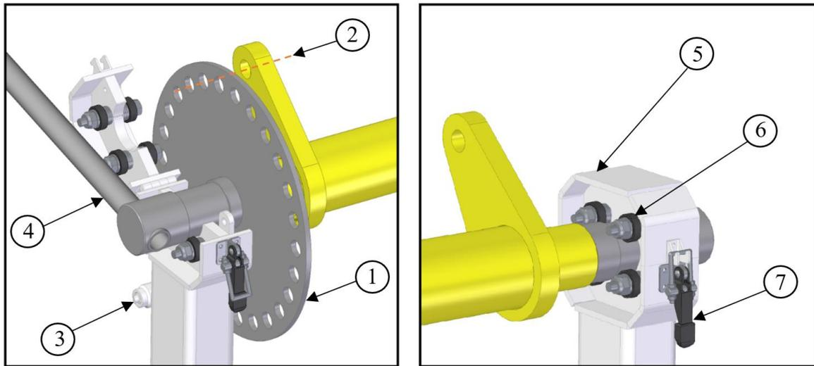
Figure 5.10 Main elements of the assembly jig
