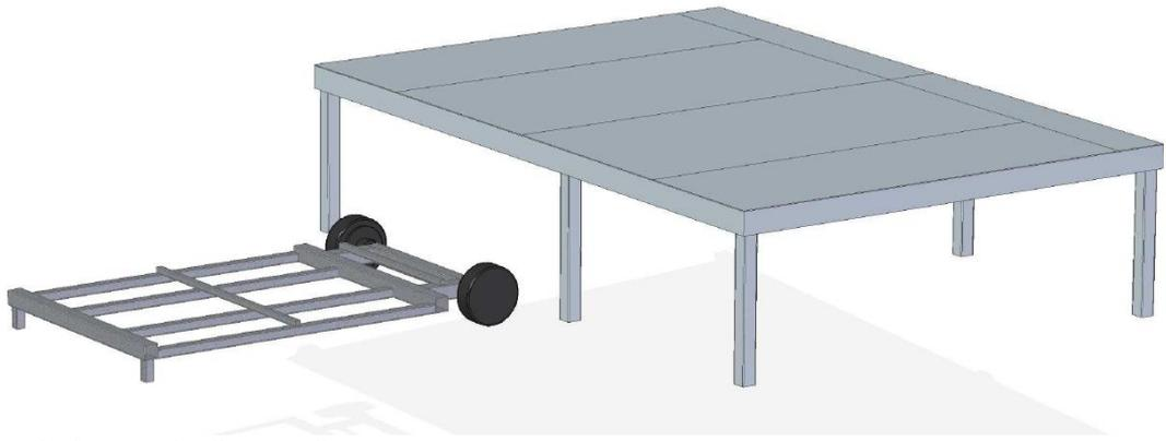
Figure 5.8 Platform and roll out trolley
