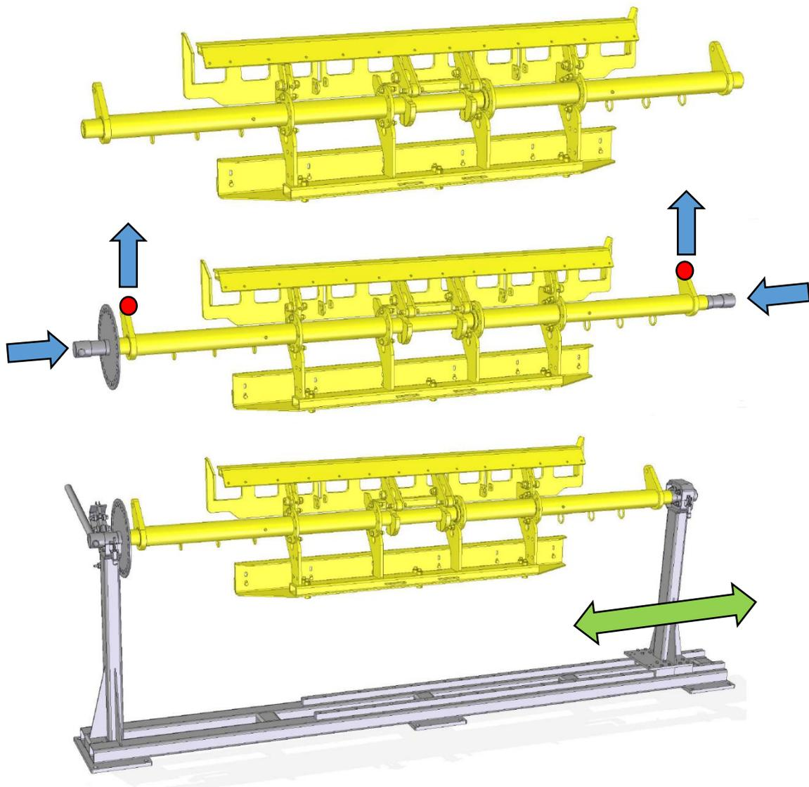
Figure 5.9 Installing of the Kärlyft product into a swiveling assembly jig
