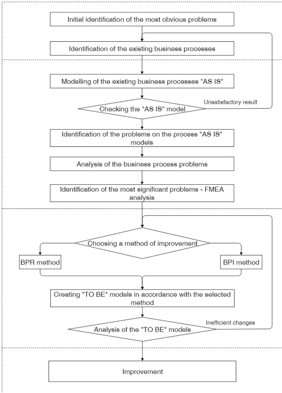
Figure 1.10 Process improvement algorithm
