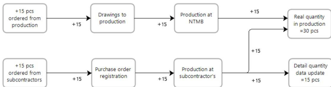
Figure 2.11 Identification of the mistake in production documentation (part 2)
