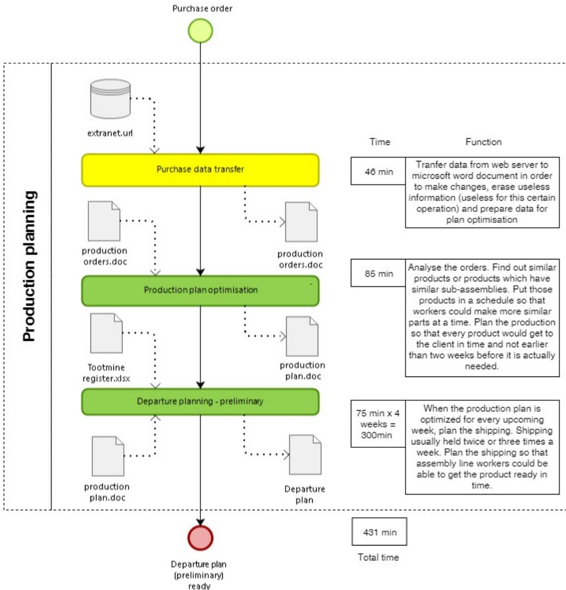
Figure 2.8 “Production planning” subprocess model
