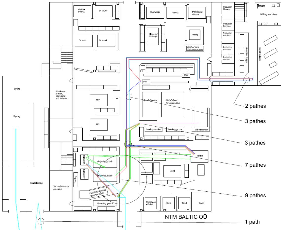
Figure 3.2 Transfer of blanks and finished products of model Standard Kärillyft 1000276053 [APX6]
