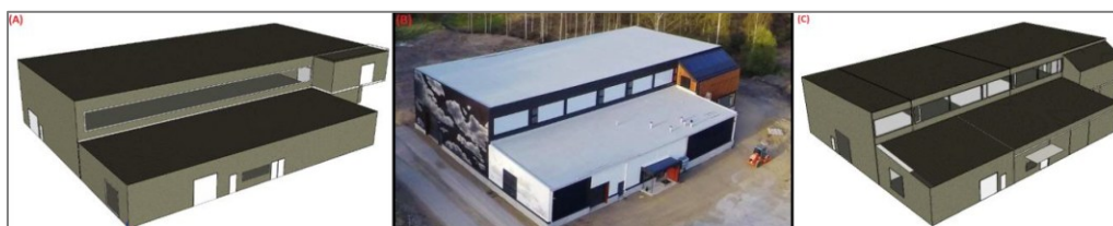
Figure 22. (a) Initial design model in IDA ICE. (b) OLK NZEB in Hämeenlinna. (c) Building calibration model in IDA ICE (Publication 4).
