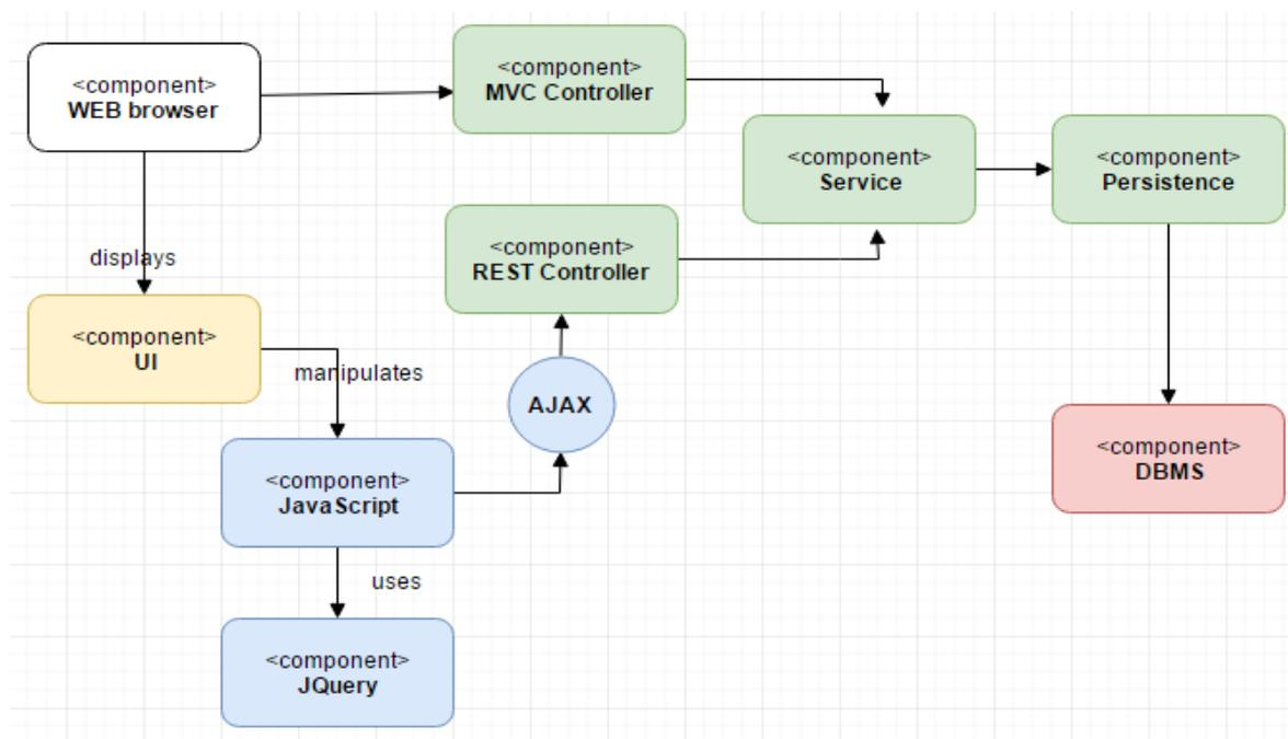
Figure 26 Application Components and their interactions.
