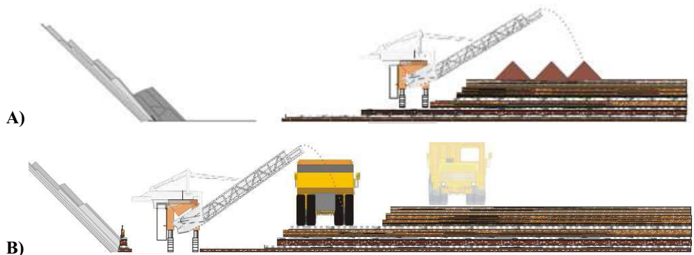
Figure 2. Surface miner loading technologies: windrowing (A) and direct truck loading (B)
