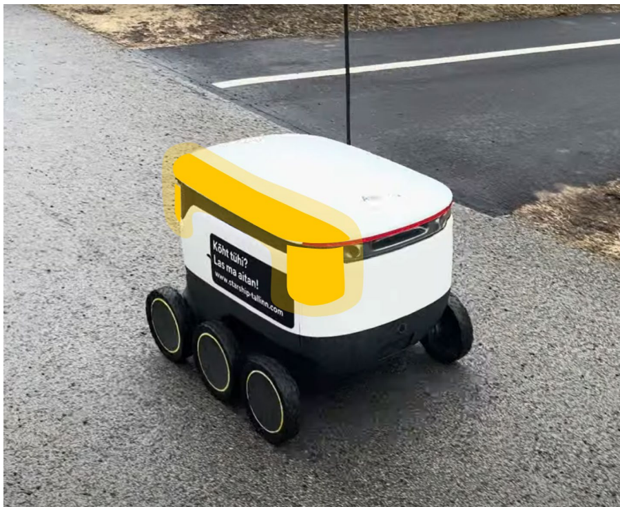
Figure 13 Proposed placement of turning lights (source: author)
