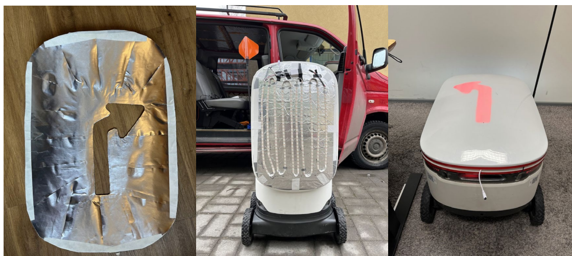
Figure 9 Components of the prototype. From left to right: (1) the underside of a stencil; (2) the light module attached to the robot's lid; (3) the light module and stencil covered with the top cover. (source: author)
