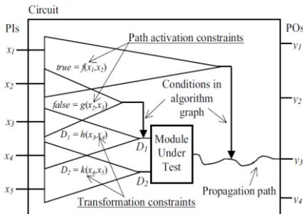
Fig. 2. Hierarchical test generation constraints
