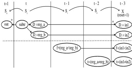
Figure 5. RT-level architecture of the GCD circuit.
