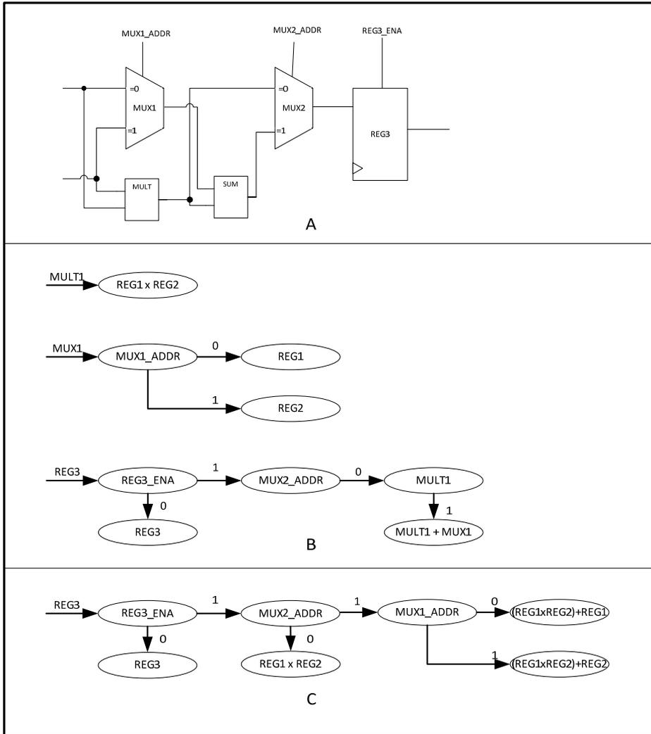
Figure 12. Datapath representing in HLDD and partitioning types
