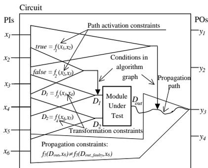
Figure 1. An example of test generation constraints
