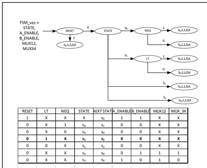
Figure 13. Converting FSM state table into HLDD
