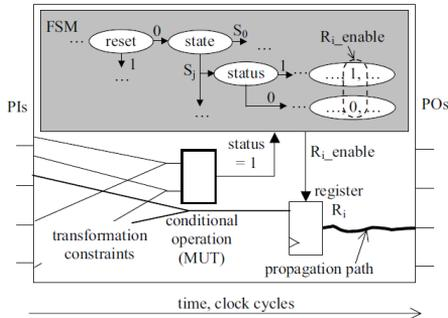
Fig. 4. FSM test covering conditional operations
