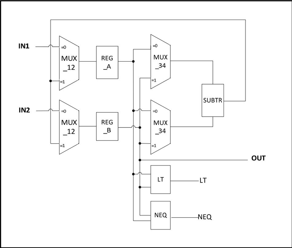
Figure 26. RT-level architecture of the GCD circuit
