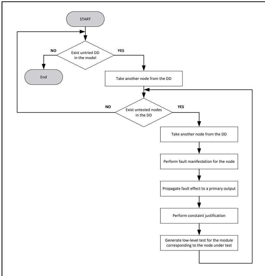
Figure 18. The general flow of the hierarchical test generation
