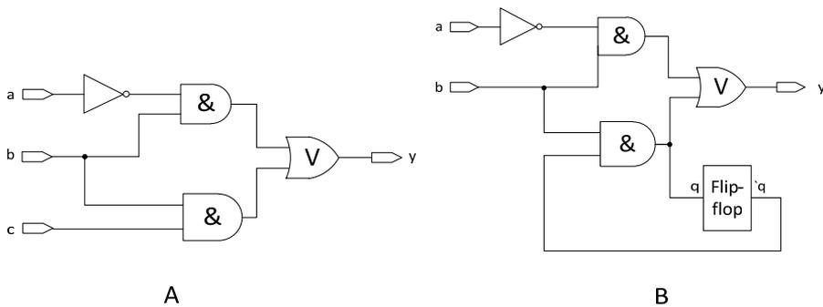
Figure 1. Combinational (A) and sequential (B) circuit example.
