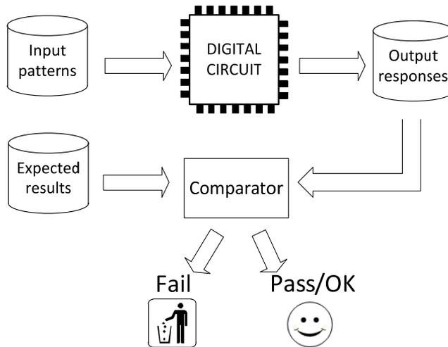
Figure 2. Digital circuits test process flow
