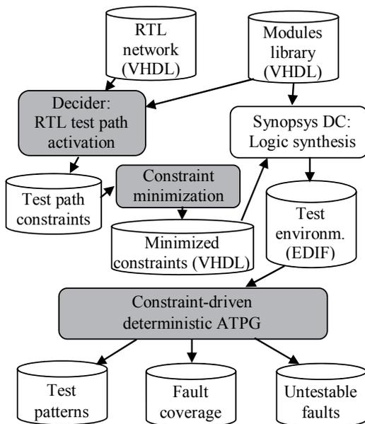
Figure 33. Constraint-based untestability proof flow
