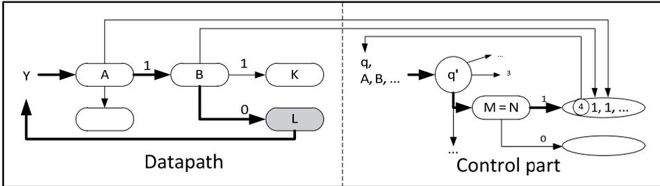
Figure 22. Fault effect propagation
