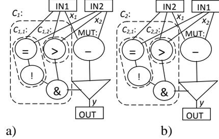
Figure 5. Full set of test path constraints for MUT
