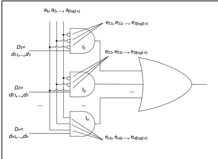
Figure 29. An  $n$ -input  $m$ -bit AND/OR multiplexer
