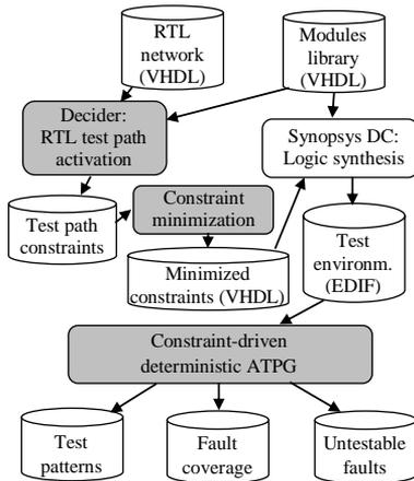
Figure 4. Constraint-based untestability proof flow
