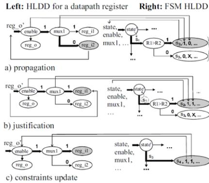
Fig. 3. RTL path activation on HLDDs
