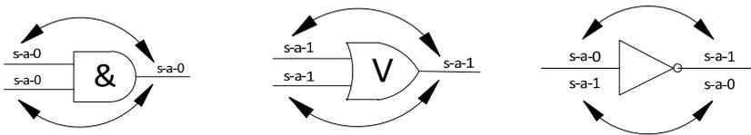
A. Equivalence relationships of stuck-at faults for basic logic gates
