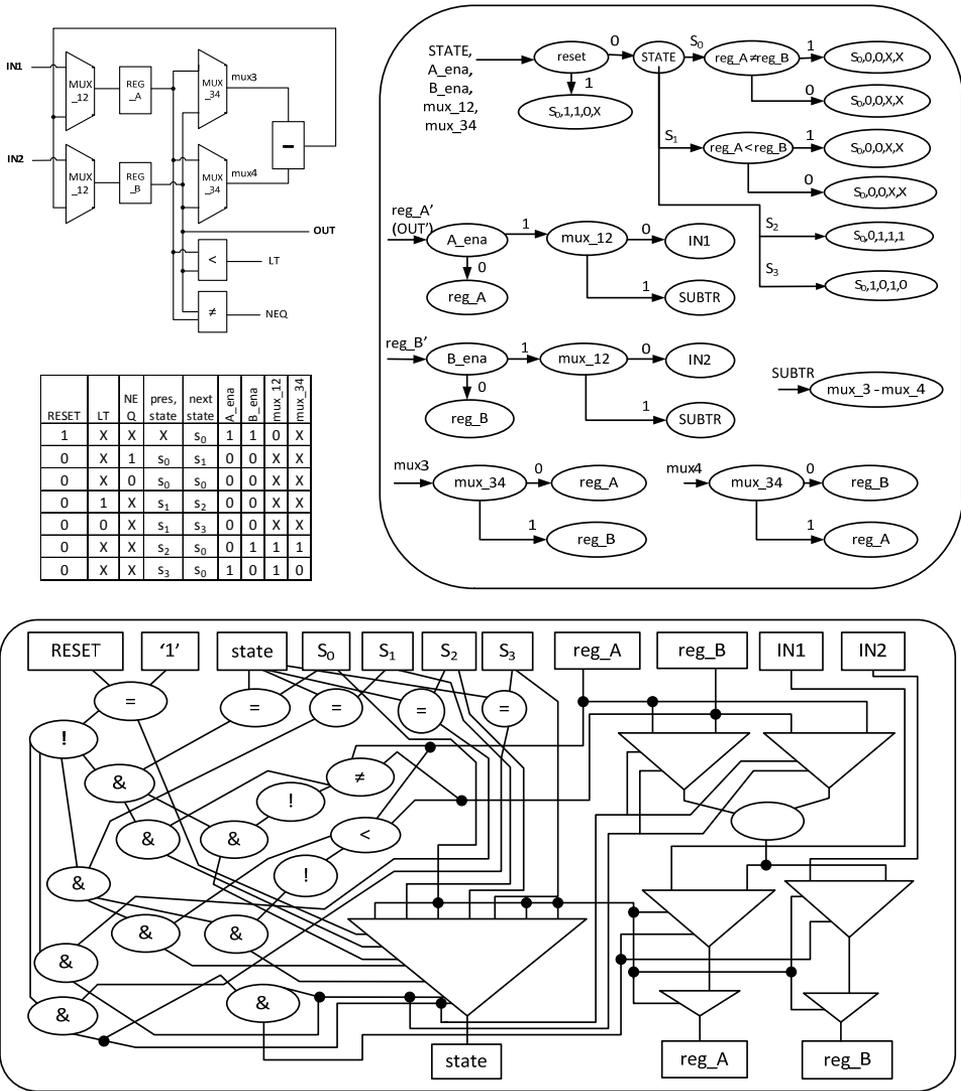
Figure 17. RTL circuit (top left), its HLDD (top right) and ADD (bottom).
