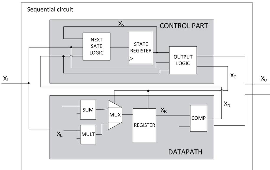
Figure 10. RTL view of a digital circuit
