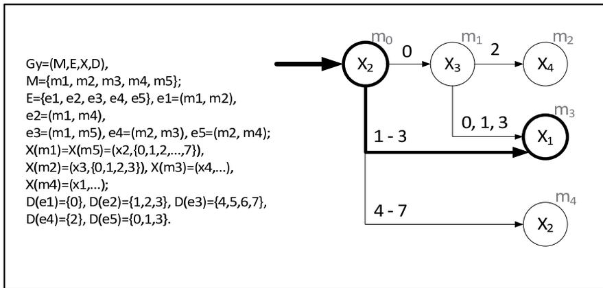
Figure 11. HLDD example for representing function  $y=f(x_1, x_2, x_3, x_4)$
