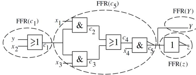
Figure 8. Partition of the combinational logic of a sequential circuit [16]
