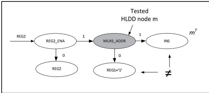
Figure 30. Functional fault model using HLDD node distinguishing
