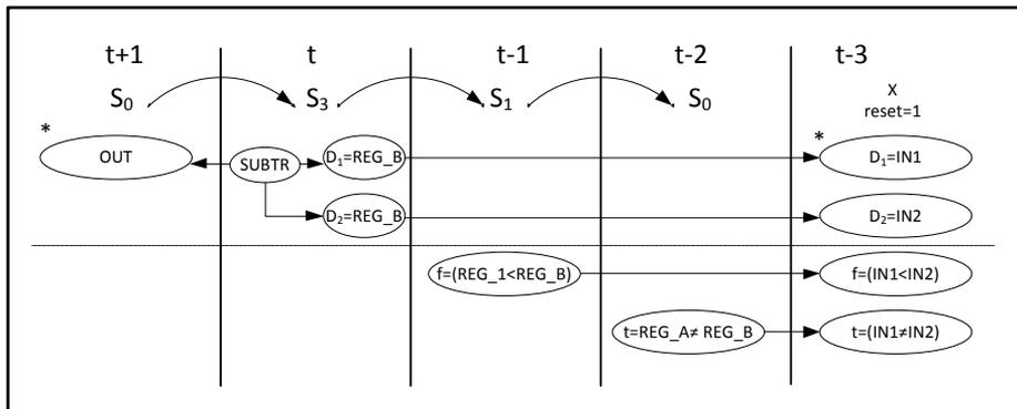
Figure 27. Constraint satisfaction process for GCD circuit
