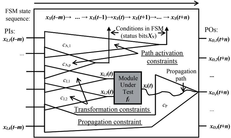
Figure 19. An unrolled RTL circuit with test generation constraints for a test path for a MUT
