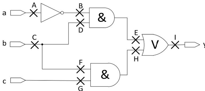
Figure 5. Potential stuck-at fault locations
