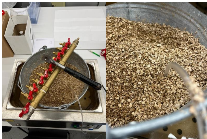
Figure 3.1 A picture containing vermiculite undergoing activation in the incubation unit
