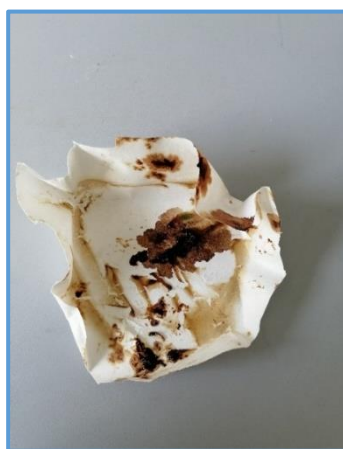
Figure 29. Degradation of CL 3:1 prepared by using craft paper cellulose by the presence of moisture.
