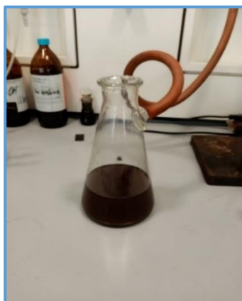
Figure 28. Degraded CL(VL) 2:1, due to high temperature and time
