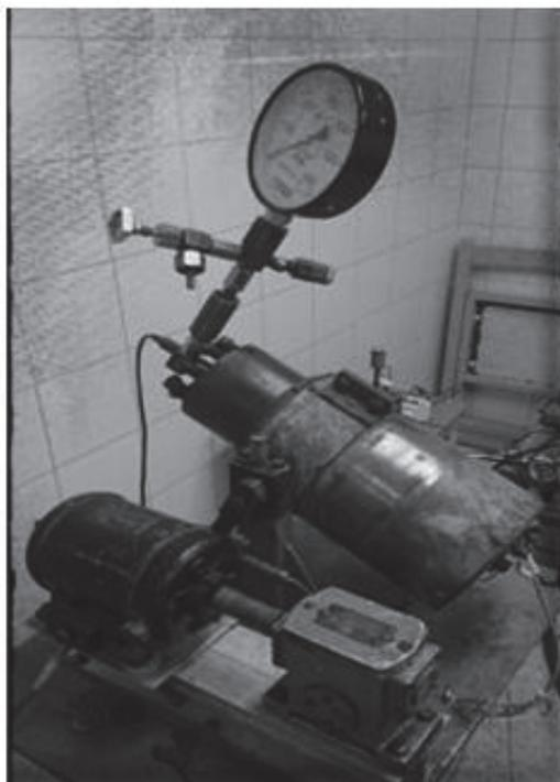
Figure 1. Batch rocking autoclave
