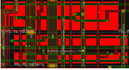
Fig. 2. Example of exposed area (highlighted in red) for cell assets (adopted from [31]).
