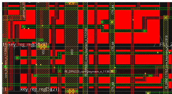
Figure 27: Example of exposed area (highlighted in red) for cell assets (from [71]).
