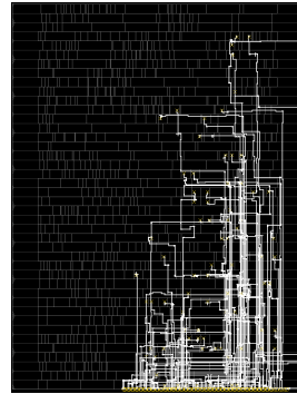
Fig. 10. A design ( PRESENT ) with most of the IO pins on the bottom side and the net assets (highlighted in white) connected to their relative IO pin.
