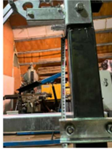
Figure 5. Spacing between lower actuator frame and pipe cycle
