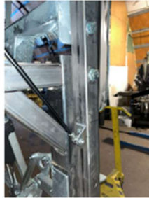
Figure 11. Mounting of the lower gas strut mount
