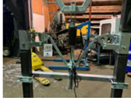
Figure 6. Assembled lower actuator mount with linkages
