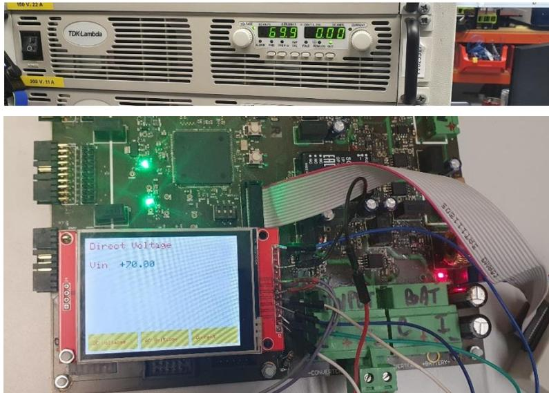
Figure 4.2 Direct Voltage Measurement
