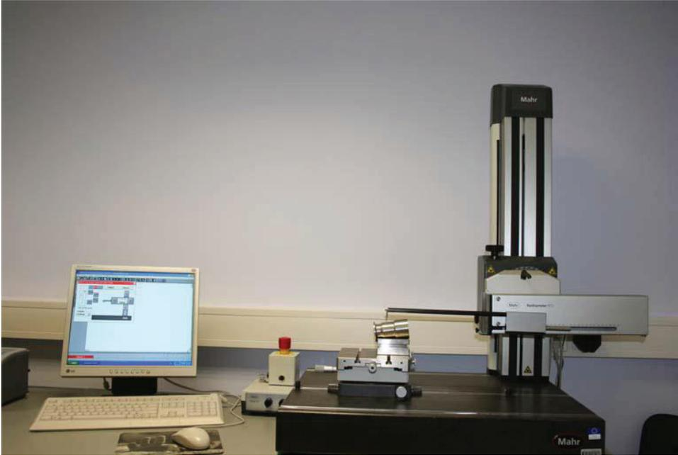
Figure 2.1 Surface profile measurement system Perthometer Concept
