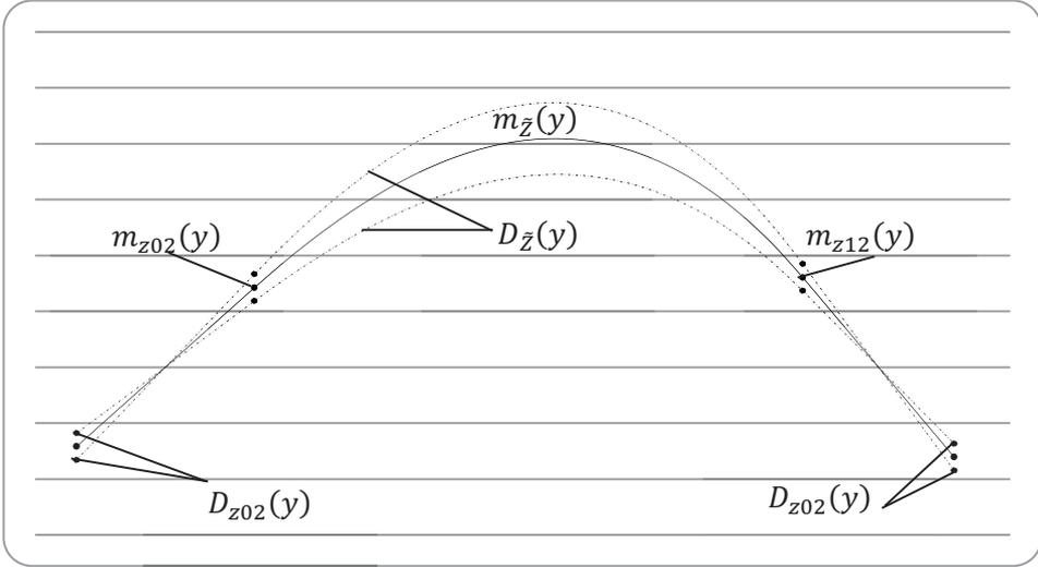
Figure 3.7 Dispersions and mean values of random functions of surface profiles [77]
