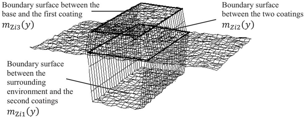
Figure 4.11 Boundary surfaces of thickness standard with two coatings
