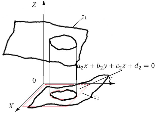
Figure 1.4 The coating thickness from the mean surface:  $z_1$  – surface between the coating and exterior environment,  $z_2$  – surface between the coating and the base
