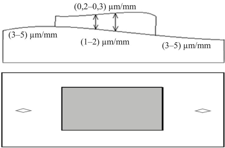
Figure 4.13 Flatness deviation of the base surface and change of coating thickness in the centre of standard [78]
