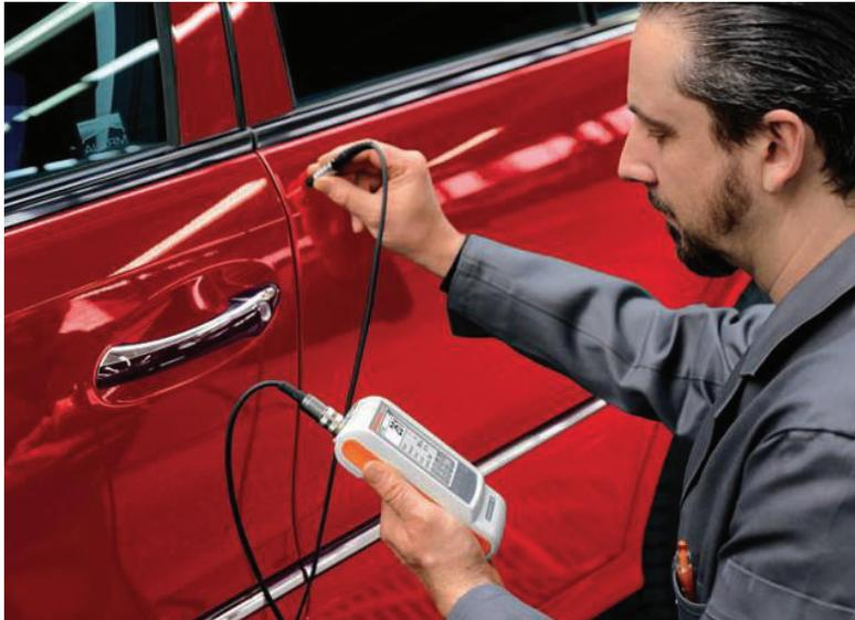
Figure 4.8 Measuring the thickness of zinc and paint in VW factory [24]
