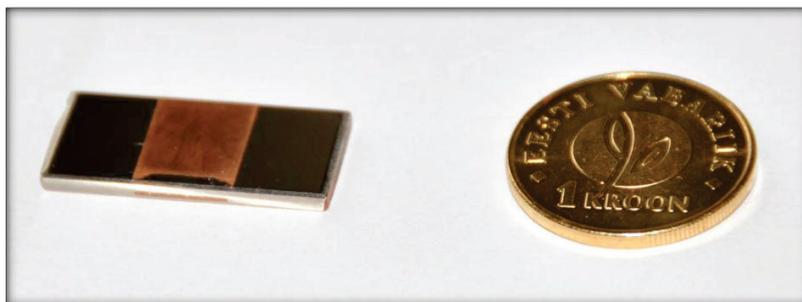
Figure 4.12 Manually made coating thickness standard (Ni-Cu)
