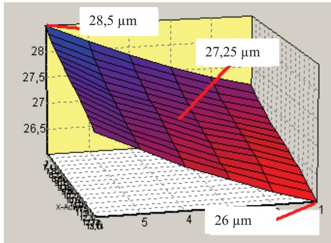
Figure 3.18 Uneven division of coating of coating thickness standards Nickel-Steel No 1001 in the middle of the measuring area
