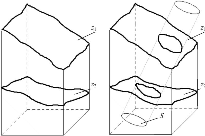
Figure 1.3 The illustration of a coated element:  $z_1$  – surface between the coating and exterior environment,  $z_2$  – surface between the coating and the base
