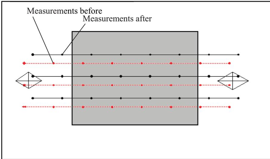
Figure 4.5 Positioning related drift towards the X and Y axis [78]
