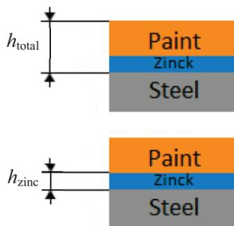
Figure 4.9 Coating thicknesses  $h_{total}$  measured with magnetic induction and  $h_{zinc}$  measured with phase-sensitive Eddy-Current method [24]
