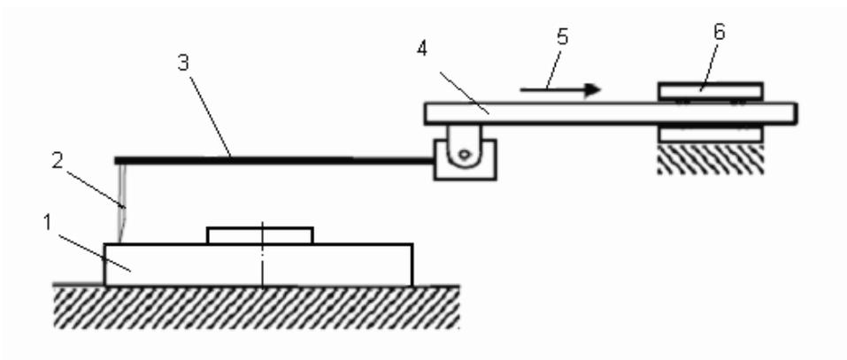
Figure 2.2 Schematic lay-out of the measurement principle: 1 – test object; 2 – stylus; 3 – tracing arm; 4 – drive unit; 5 – measuring direction; 6 – calibrated support [3]
