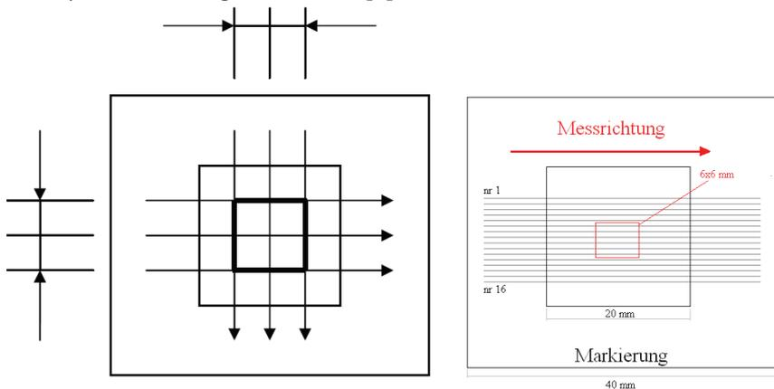
Figure 3.17 Measurement scheme of thickness standard used in TUT (1997, 2005), PTB (1999) on the left and PTB (2009) on the right
