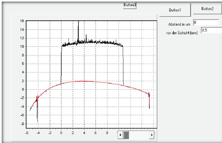
Figure 4.16 Measuring and calculating program for measuring covering thickness
