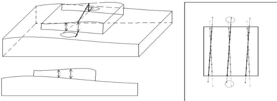
Figure 4.6 The effect of positioning on the results of coating thickness measurement [78]
