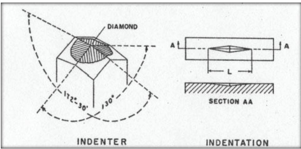
Figure 4.14 The indenter of the Knoop microhardness tester and the image of indentation [66]
