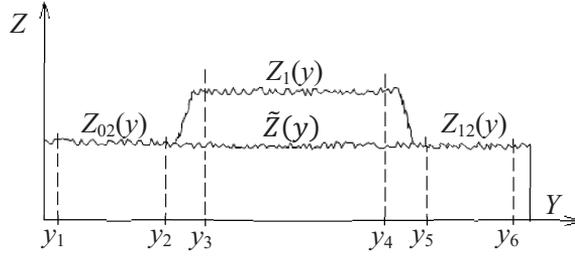
Figure 3.4 Random functions characterizing the top surface [96]
