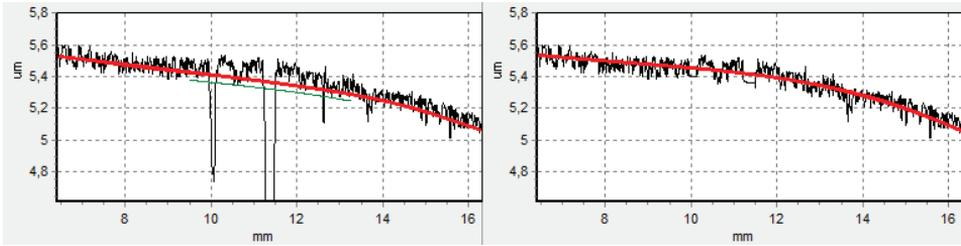
Figure 3.11 Unfiltered profile (on the left) and filtered profile (on the right)
