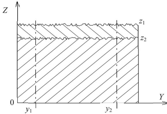
Figure 3.2 Element of the object:  $z_1$  – surface between the coating and exterior environment,  $z_2$  – surface between the coating and the base [1]
