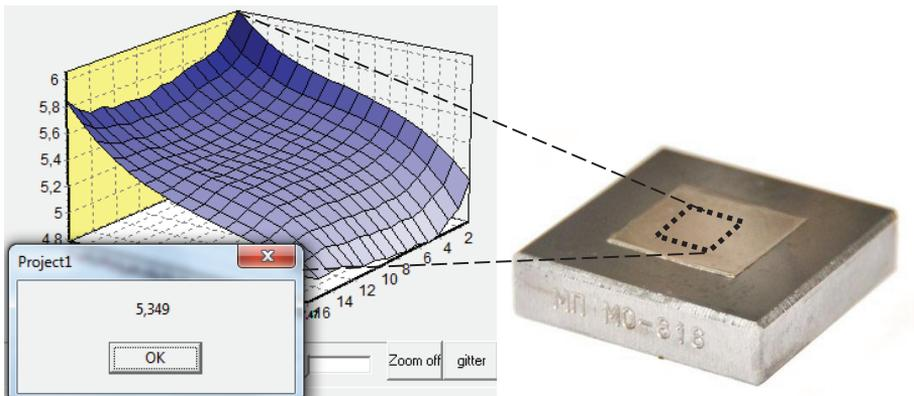
Figure 3.12 Graphic depiction of the coating thickness of the coating thickness standard
