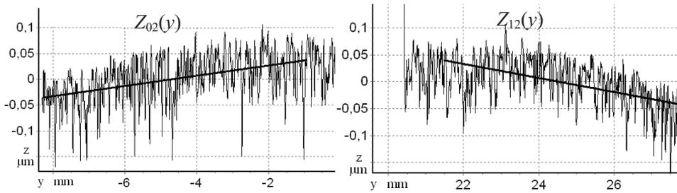
Figure 3.14 True profile of the base surface and  $m_{z_{02}}(y)$  (left)  $m_{z_{12}}(y)$  (right) - mean value of function  $Z_{02}(y)$  and  $Z_{12}(y)$  [77]
