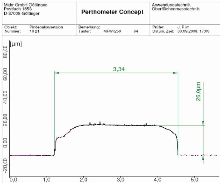
Figure 2.3 The coating thickness standards contour measured with Perthometer Concept [2]
