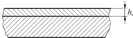
Figure 1.1 Theoretical coating thickness
