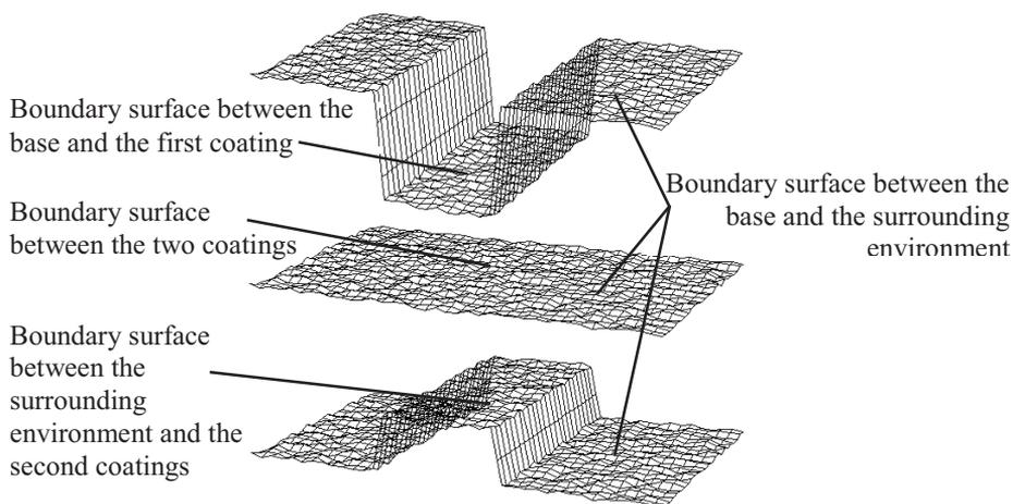
Figure 4.10 Three different profiles measured [40, 41]
