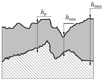
Figure 1.2 Various coating thicknesses
