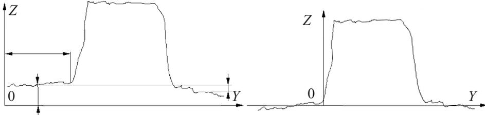
Figure 3.9 Initial measurement data (on the left) and adjusted measurement data (on the right)
