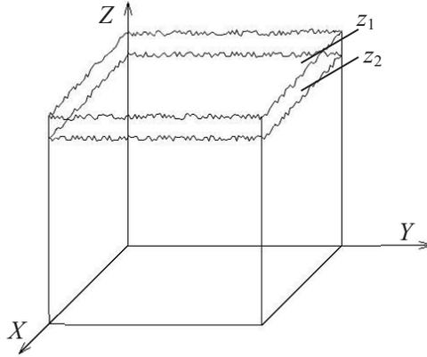
Figure 3.1 The coated object:  $z_1$  – surface between the coating and exterior environment,  $z_2$  – surface between the coating and the base [1]
