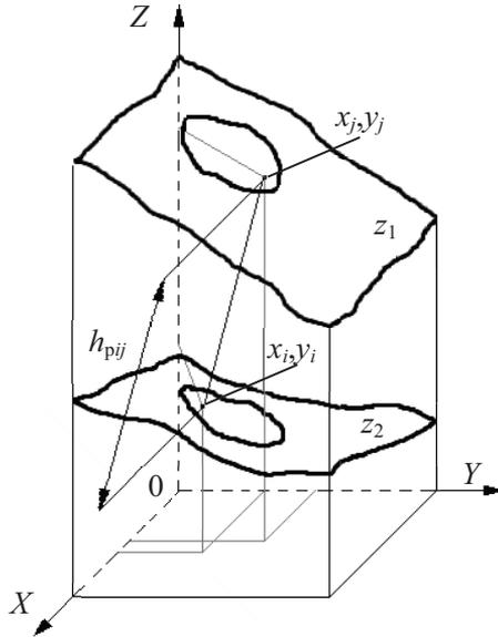
Figure 1.5 The coating thickness located in between two boundary surfaces  $z_1$  and  $z_2$
