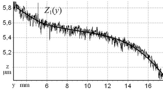
Figure 3.15 Measured profile of the coating surface and  $m_{z_1}(y)$  - mean value of function  $Z_1(y)$  [77]
