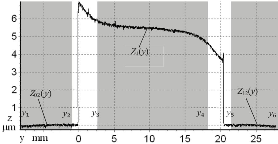
Figure 3.13 Profile of the base (of coating thickness standard No 1055) and functions  $Z_{02}$ ,  $Z_{12}$  and  $Z_1$  [77]
