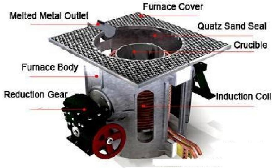
**Figure 3. Induction furnace** ( Weifang Jinhuaixin Electric Furnace Manufacturing )
