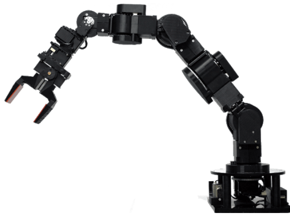
Figure 8. Picture of Cyton Gamma 1500 robot arm [24]
