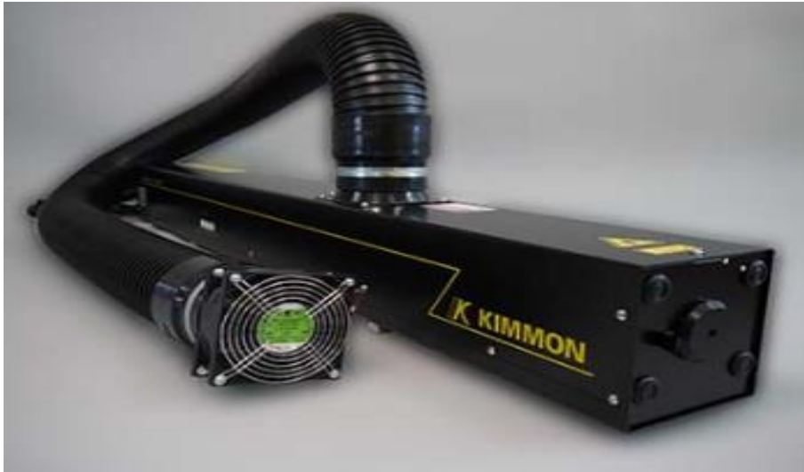
Figure 1:11: KIMMON IK series He-Cd laser with the wavelength of 325 nm
