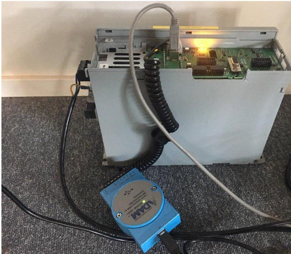
Figure 22. An example of a P400 drive that can be upgraded over APST.
