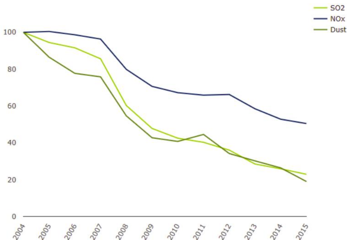
Chart – Indexed SO 2 , NO x and dust emissions from large combustion plants in the European Union
