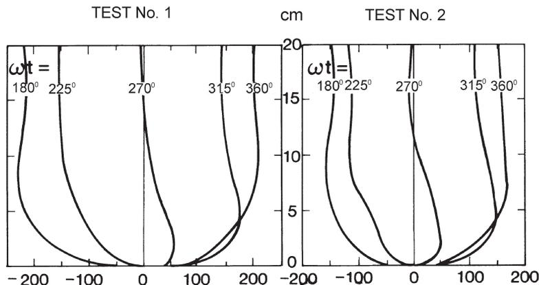
**Fig. 2.** Instantaneous velocities  $u(z, t)$  plotted against elevation from top of the roughness elements. Numbers on the curves refer to the phase  $\omega t$  of the free stream velocity  $A\omega \sin \omega t$  [1].
