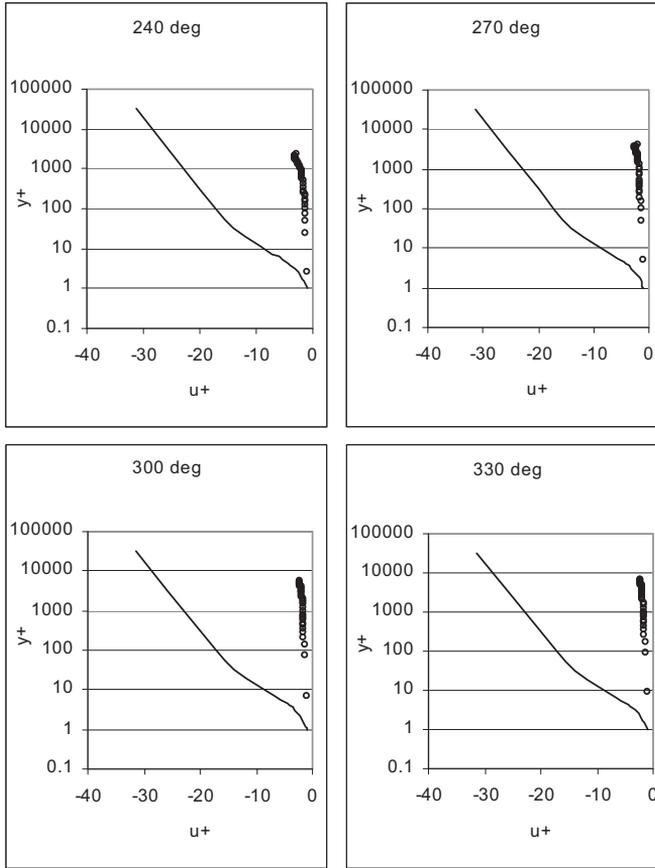
Figure 18 Dimensionless velocity profiles of  $u^+$  at different phases of the wave breaking: section  $(x - x_b) / h_b = 0.09$
