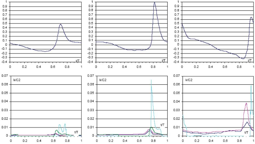
Figure 22 Surface elevation and turbulent kinetic energy in cross-sections  $x - x_b/h_b = -2.36$  (left column),  $x - x_b/h_b = 0.09$  (centre column) and  $x - x_b/h_b = 2.17$  (right column). at heights  $(y - \bar{\eta})/h = -0.99$ , (—)  $(y - \bar{\eta})/h = -0.89$ , (—)  $(y - \bar{\eta})/h = -0.54$ , (—)  $(y - \bar{\eta})/h = -0.17$ , (—)  $(y - \bar{\eta})/h = 0.18$
