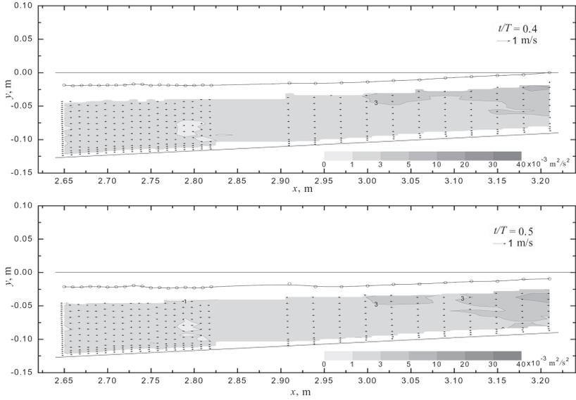
**Fig. 10.** Turbulent kinetic energy and velocity field at  $t/T = 0.4$  and  $0.5$ .
