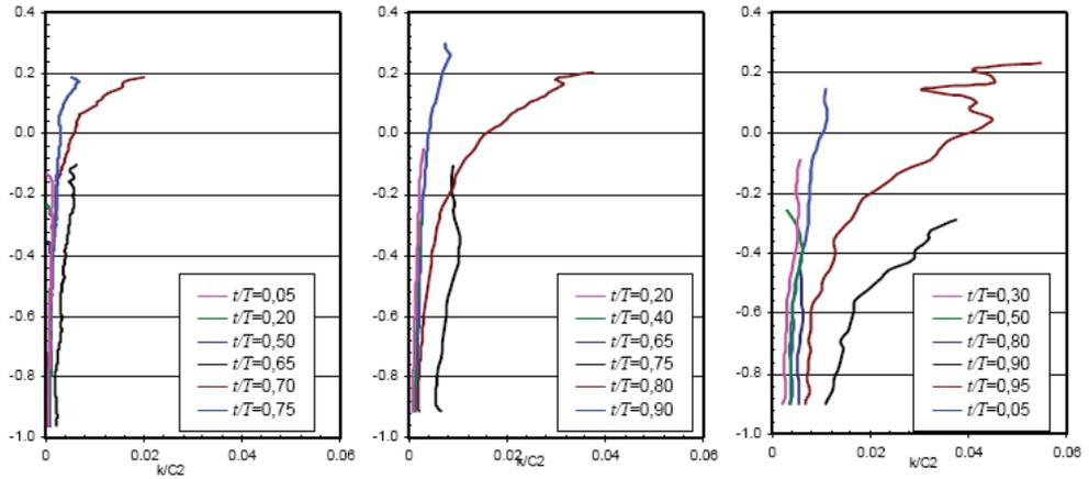
Figure 23 Ensemble-averaged turbulent kinetic energy profiles. Left column  $x - x_b / h_b = -2.36$ , middle column  $x - x_b / h_b = 0.09$  and right column  $x - x_b / h_b = 2.17$
