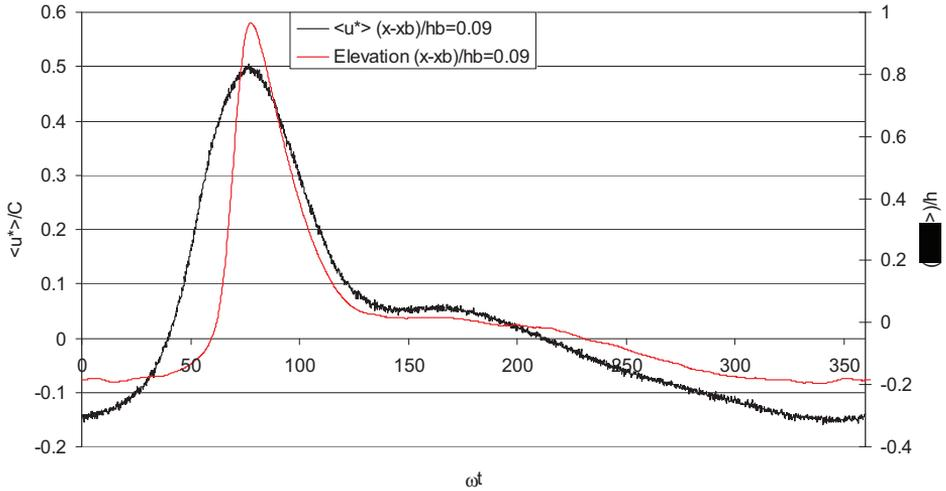
Figure 13 Ensemble averaged variation of non-dimensional shear velocity and the surface elevation at  $(x - x_b) / h_b = 0.09$
