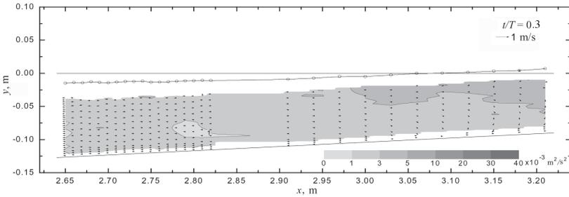
**Fig. 9.** Turbulent kinetic energy and velocity field at  $t/T = 0.2$  and  $0.3$ .
