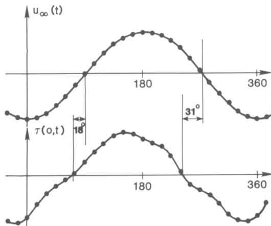
*Figure 1 Time variations of the bed shear stress  $\tau(0,t)$  for a rough turbulent flow over relatively small roughness elements Svendsen (1976).*
