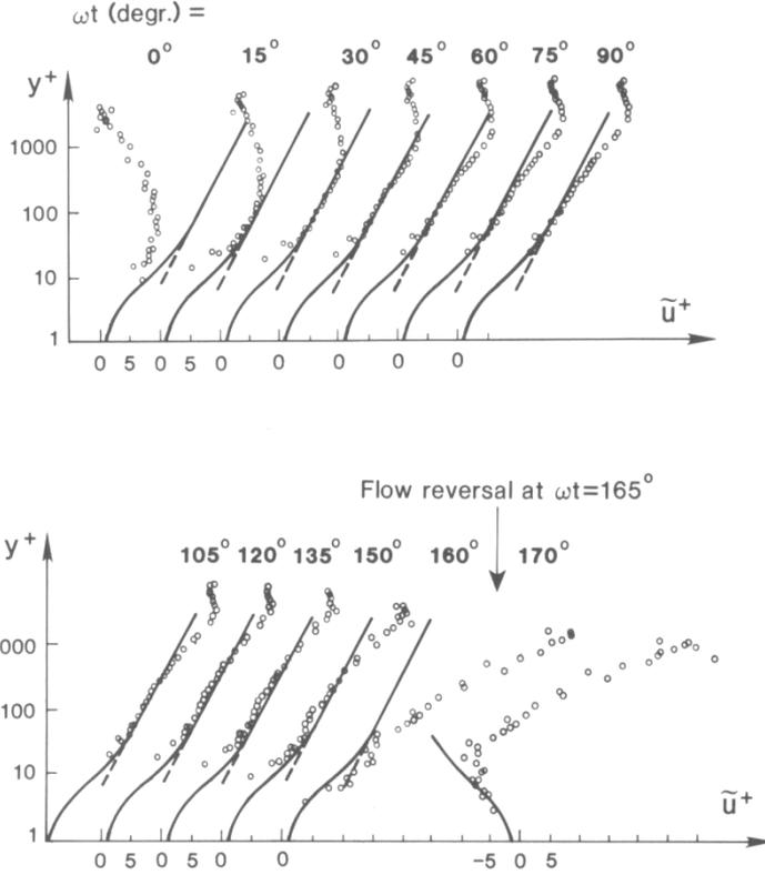
Figure 3 Dimensionless velocity profiles for smooth turbulent oscillatory flows at different phases of the free stream velocity  $A\omega\sin\omega t$  Jensen (1989)
