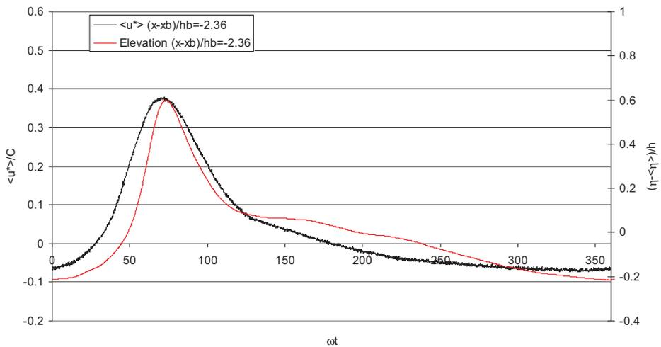
Figure 12 Ensemble-averaged variation of non-dimensional shear velocity and the surface elevation at  $(x - x_b)/h_b = -2.36$
