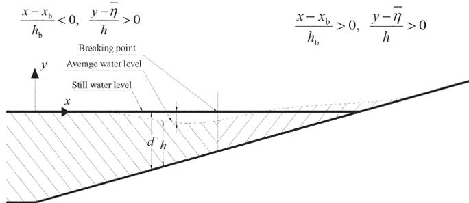
Fig. 4. Definition of flow parameters.
