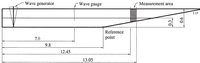
Fig. 1. Wave flume, dimensions in m.
