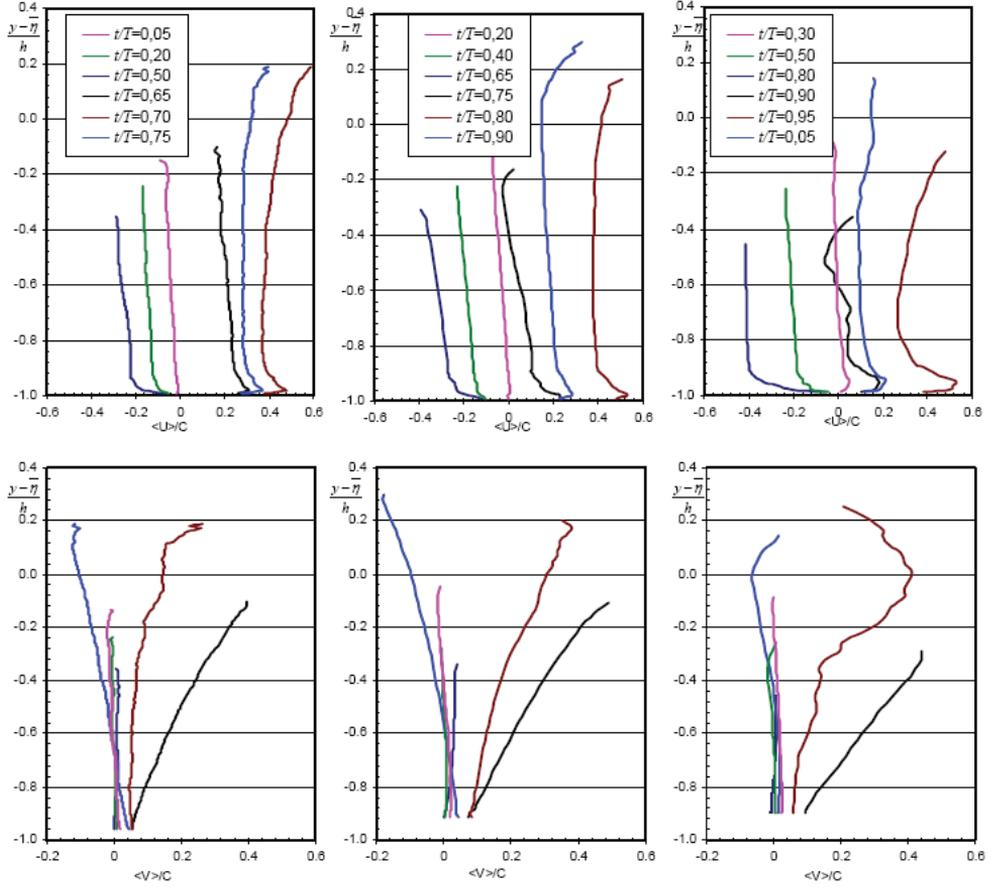
Figure 10 Ensemble-averaged horizontal and vertical velocity profiles. Left column  $x - x_b / h_b = -2.36$ , middle column  $x - x_b / h_b = 0.09$  and right column  $x - x_b / h_b = 2.17$
