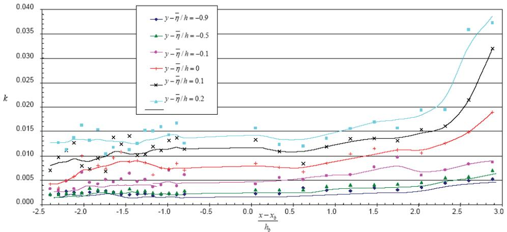
Figure 24 Time-averaged variation of turbulent kinetic energy perpendicular to the coastline at different heights above the bottom
