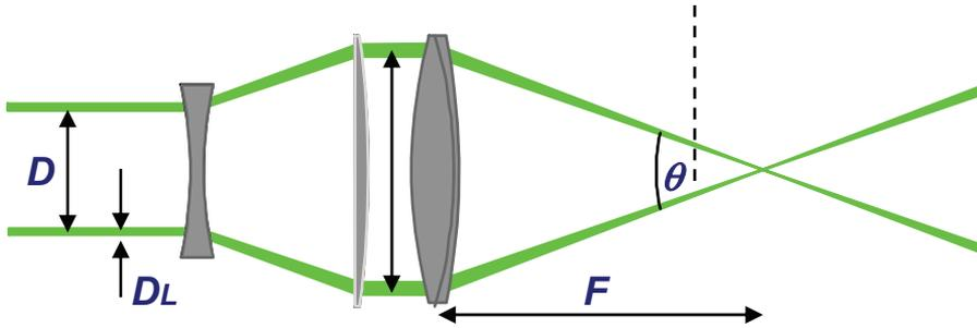
Figure 5 Explanation to Equation (11).  $D$  is the distance between the laser beams,  $D_L$  is the diameter of the laser beam,  $F$  is the focal distance of the frontal lens and  $\theta$  is the angle between the laser beams
