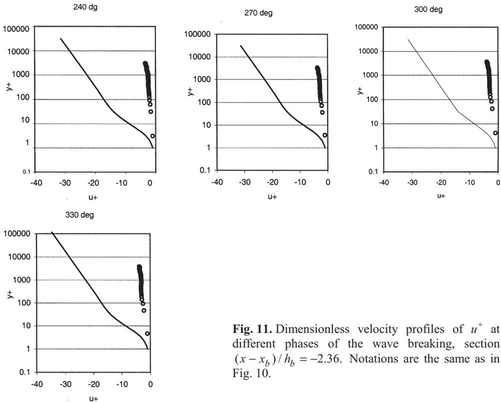
**Fig. 11.** Dimensionless velocity profiles of  $u^+$  at different phases of the wave breaking, section  $(x - x_b)/h_b = -2.36$ . Notations are the same as in Fig. 10.
