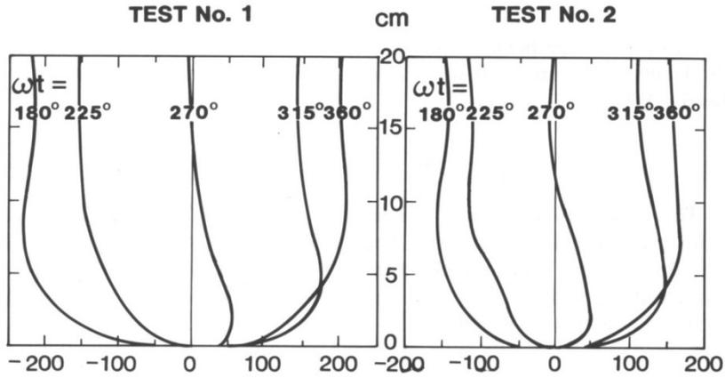
Figure 2 Instantaneous velocities  $u(z,t)$  plotted against elevation from the top of the roughness elements. Numbers on the curves refer to the phase of the free stream velocity  $A\omega \sin \omega t$  Jonsson (1966)
