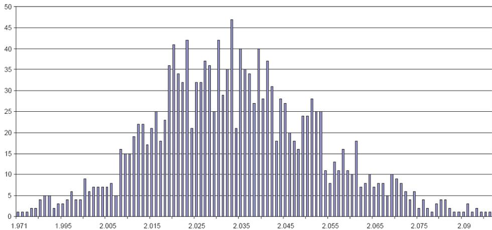
Figure 7 Spectra of wave periods for 12 consequent experimental runs  $N$  corresponds to the number of occurrences of the wave period
