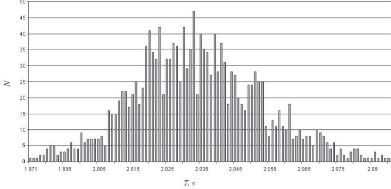
**Fig. 3.** Spectrum of wave periods for 12 consequent experimental runs.
