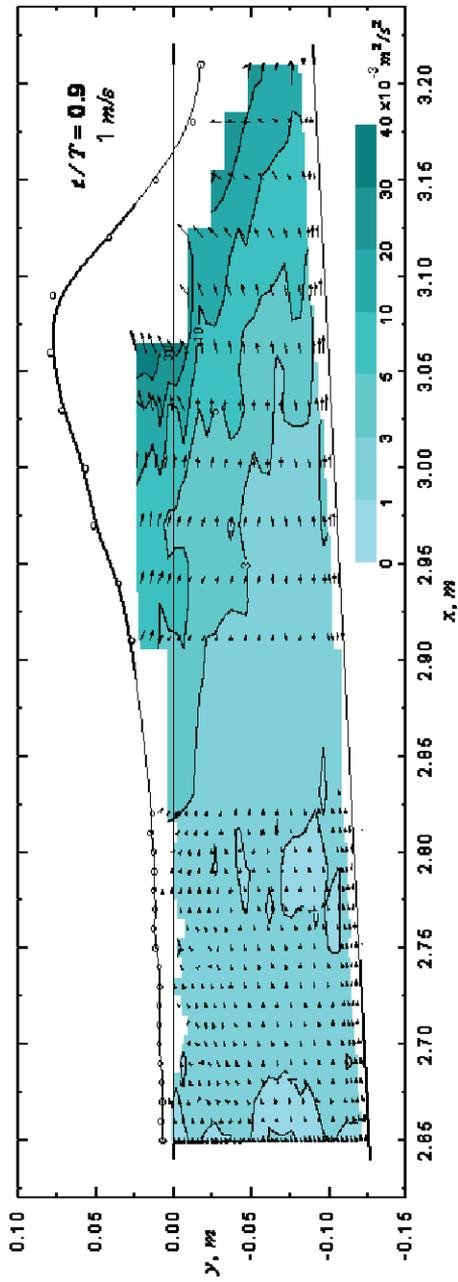
Figure 30 Turbulent kinetic energy and velocity field at  $t/T=0.9$
