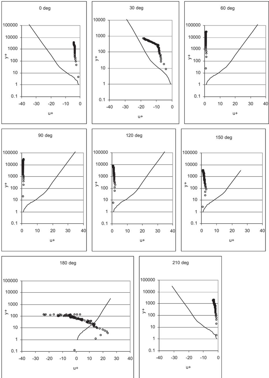
Figure 15 Dimensionless velocity profiles of  $u^+$  at different phases of the wave breaking: section  $(x - x_b)/h_b = -2.36$
