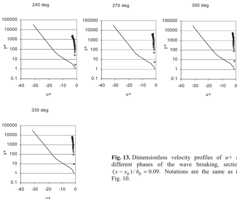
**Fig. 13.** Dimensionless velocity profiles of  $u^+$  at different phases of the wave breaking, section  $(x - x_b)/h_b = 0.09$ . Notations are the same as in Fig. 10.
