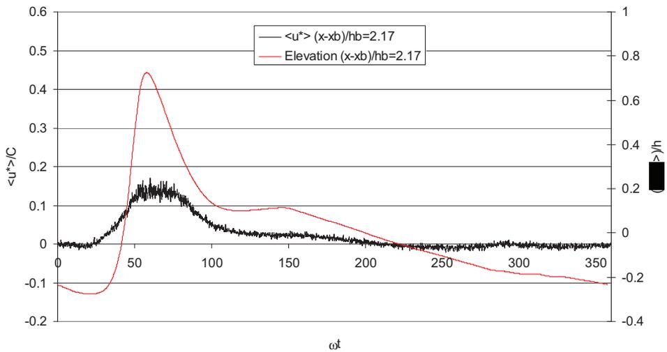
Figure 14 Ensemble averaged variation of non-dimensional shear velocity and the surface elevation at  $(x - x_b) / h_b = 2.17$
