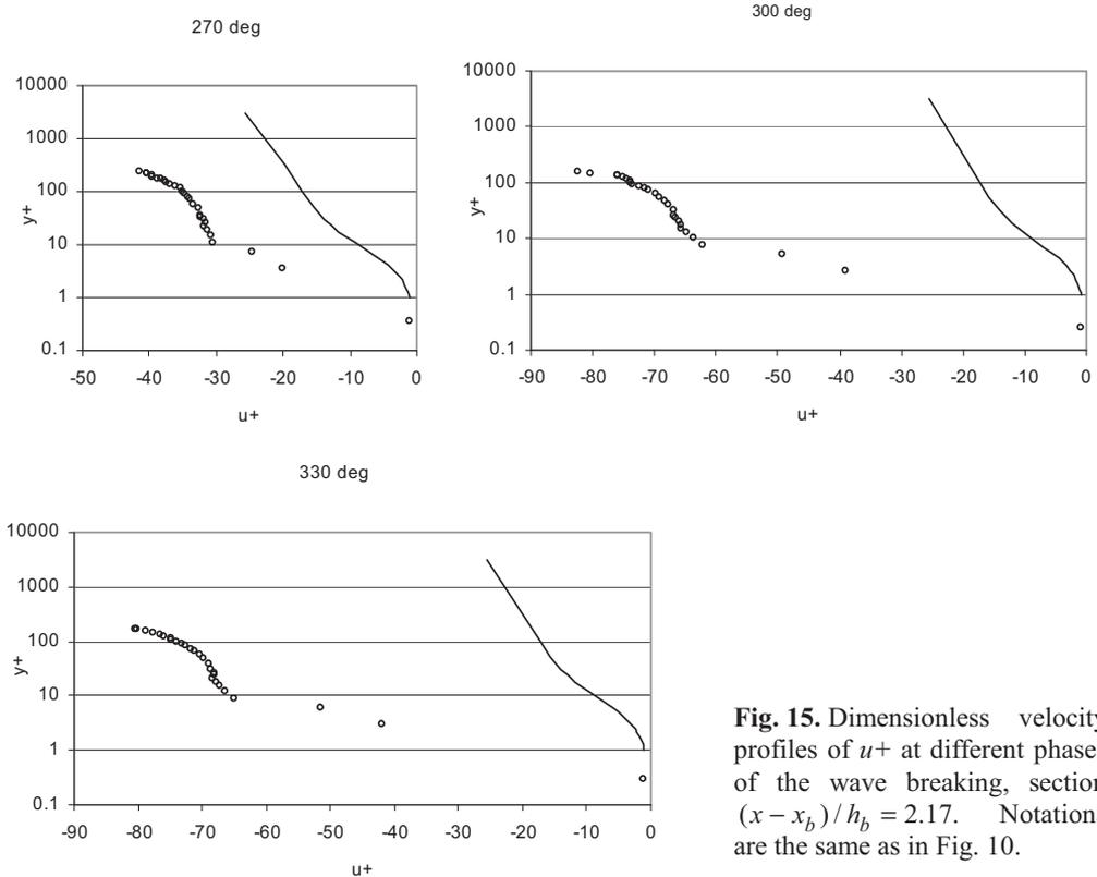
**Fig. 15.** Dimensionless velocity profiles of  $u^+$  at different phases of the wave breaking, section  $(x - x_b)/h_b = 2.17$ . Notations are the same as in Fig. 10.
