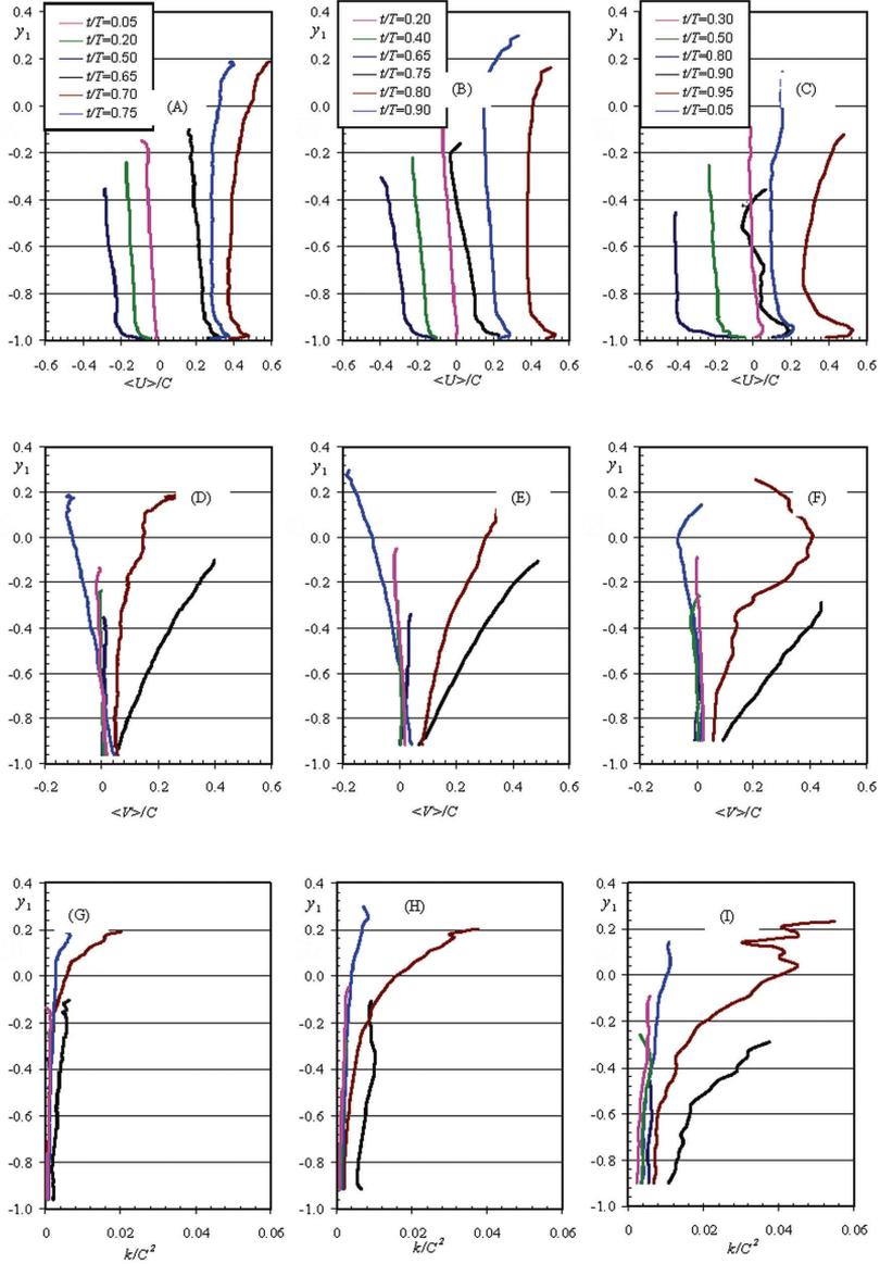
**Fig. 6.** Ensemble-averaged horizontal (A–C) and vertical (D–F) velocity and turbulent kinetic energy (G–I) profiles; left column:  $(x - x_b) / h_b = -2.36$ ; middle column:  $(x - x_b) / h_b = 0.09$ ; right column:  $(x - x_b) / h_b = 2.17$ .
