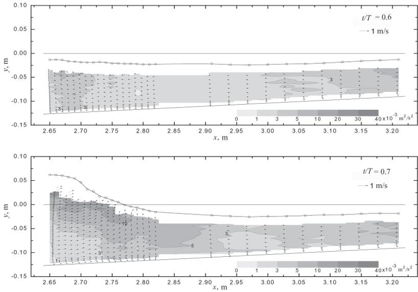
**Fig. 11.** Turbulent kinetic energy and velocity field at  $t/T = 0.6$  and  $0.7$ .
