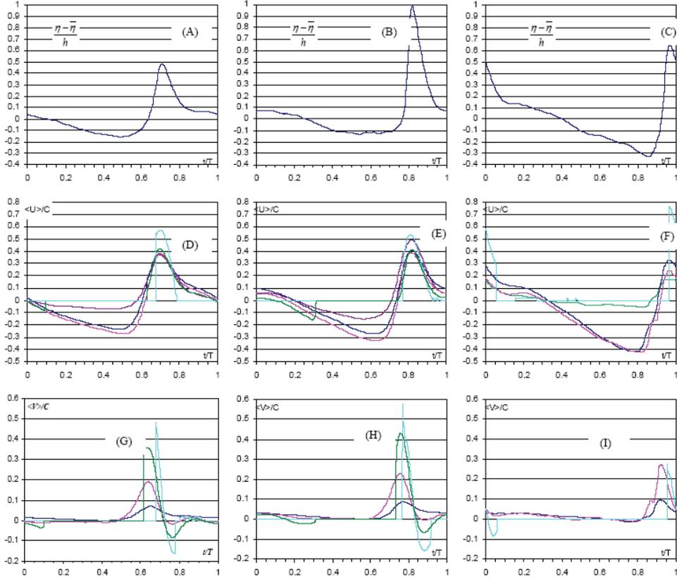
Figure 9 Surface elevation (A-C), horizontal velocity component (D-F) and vertical velocity component (G-I) in cross-sections  $x - x_b / h_b = -2.36$  (left column),  $x - x_b / h_b = 0.09$  (centre column) and  $x - x_b / h_b = 2.17$  (right column). at heights  $(y - \bar{\eta}) / h = -0.99$ , (—)  $(y - \bar{\eta}) / h = -0.89$ , (—)  $(y - \bar{\eta}) / h = -0.54$ , (—)  $(y - \bar{\eta}) / h = -0.17$ , (—)  $(y - \bar{\eta}) / h = 0.18$
