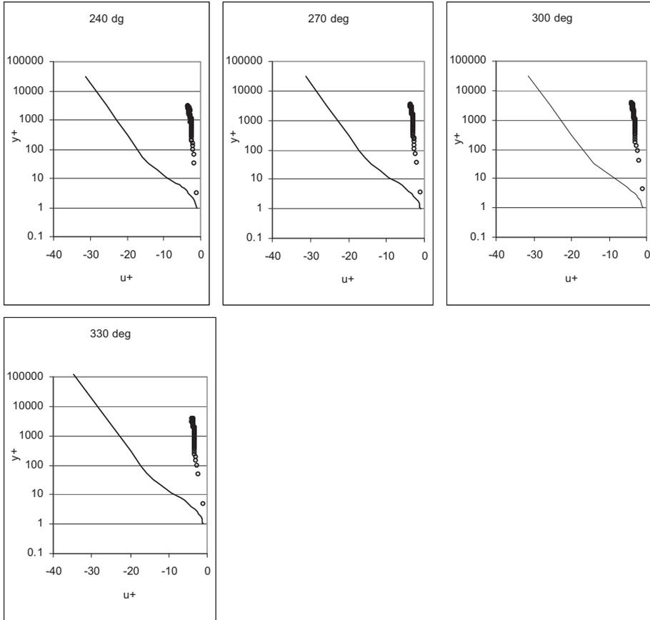
Figure 16 Dimensionless velocity profiles of  $u^+$  at different phases of the wave breaking: section  $(x - x_b)/h_b = -2.36$
