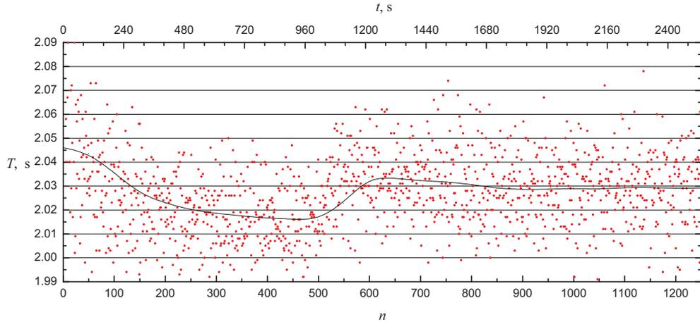
Figure 6 Stabilization of the wave periods after the start of the wave generator
