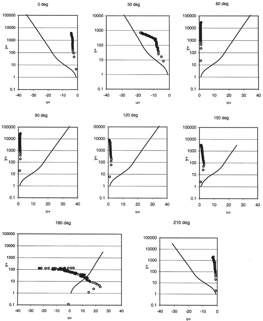
**Fig. 10.** Dimensionless velocity profiles of  $u^+$  at different phases of the wave breaking, section  $(x - x_b)/h_b = -2.36$ ; circles show experimental points, solid line indicates the calculated velocity profile in the assumption of the stationary flow.
