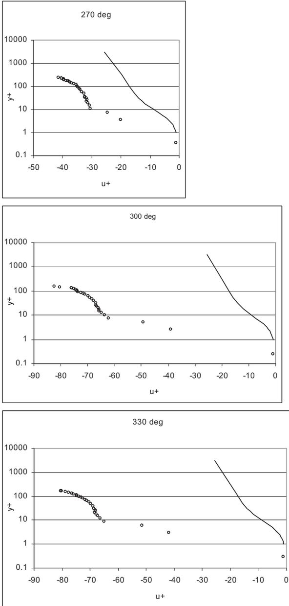
Figure 20 Dimensionless velocity profiles of  $u^+$  at different phases of the wave breaking: section  $(x - x_b)/h_b = 2.17$
