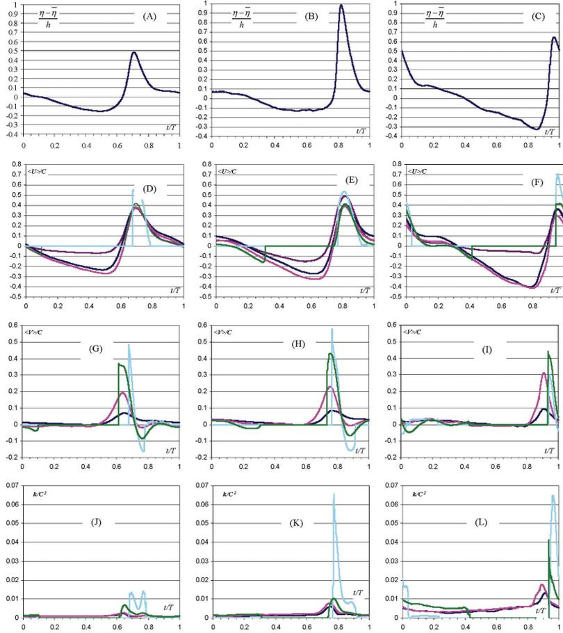
**Fig. 5.** Surface elevation (A–C), horizontal velocity component (D–F), vertical velocity component (G–I) and turbulent kinetic energy (J–L) in cross-sections  $(x - x_b)/h_b = -2.36$  (left column),  $(x - x_b)/h_b = 0.09$  (centre column) and  $(x - x_b)/h_b = 2.17$  (right column) at the heights: —  $(y - \bar{\eta})/h = -0.99$ , —  $(y - \bar{\eta})/h = -0.89$ , —  $(y - \bar{\eta})/h = -0.54$ , —  $(y - \bar{\eta})/h = -0.17$ , —  $(y - \bar{\eta})/h = 0.18$ .
