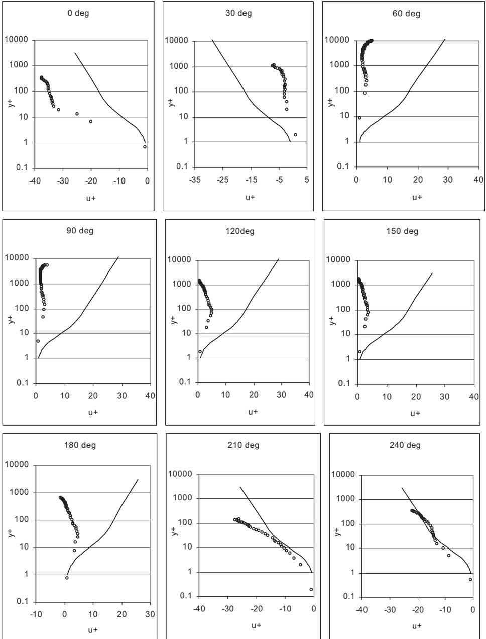
Figure 19 Dimensionless velocity profiles of  $u^+$  at different phases of the wave breaking: section  $(x - x_b)/h_b = 2.17$
