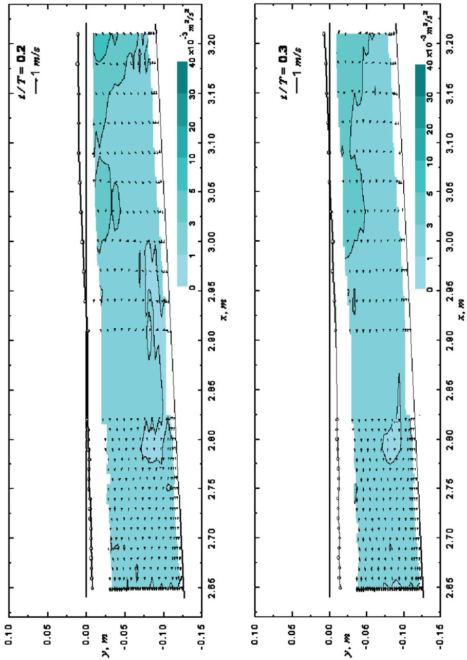
Figure 26 Turbulent kinetic energy and velocity field at  $t/T=0.2$  and  $t/T = 0.3$
