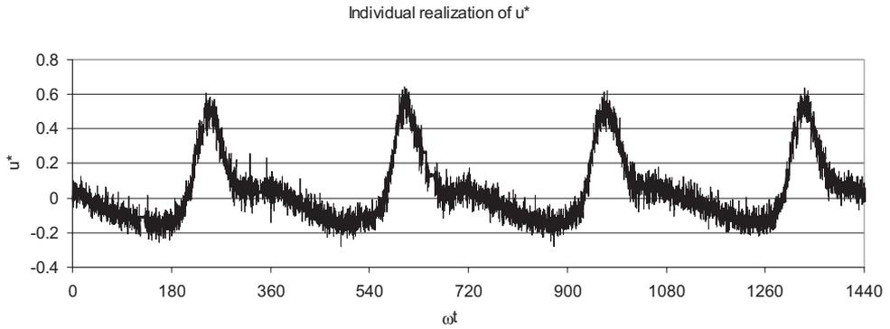
Figure 11 Measured time series of shear velocity before data processing
