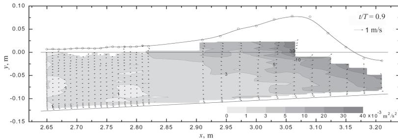
**Fig. 13.** Turbulent kinetic energy and velocity field at  $t/T = 0.9$ .
