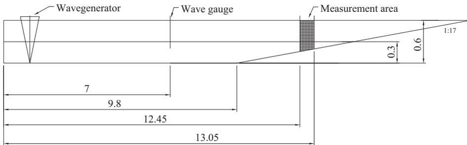
Figure 4 Wave flume (measurements in meters)
