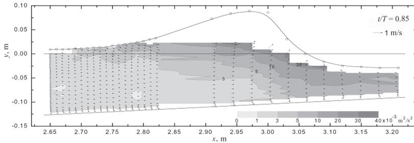
**Fig. 12.** Turbulent kinetic energy and velocity field at  $t/T = 0.8$  and  $0.85$ .
