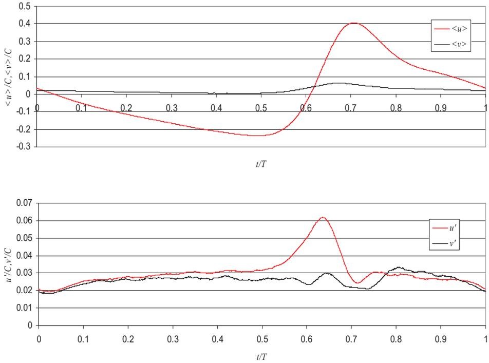
Figure 21 Ensemble-averaged horizontal and vertical components of the local velocity at the point with coordinates  $(x - x_b) / h_b = -2.26$  and  $(y - \bar{\eta}) / h = -0.87$  and the corresponding turbulent ensemble-averaged turbulent fluctuations  $u'$  and  $v'$
