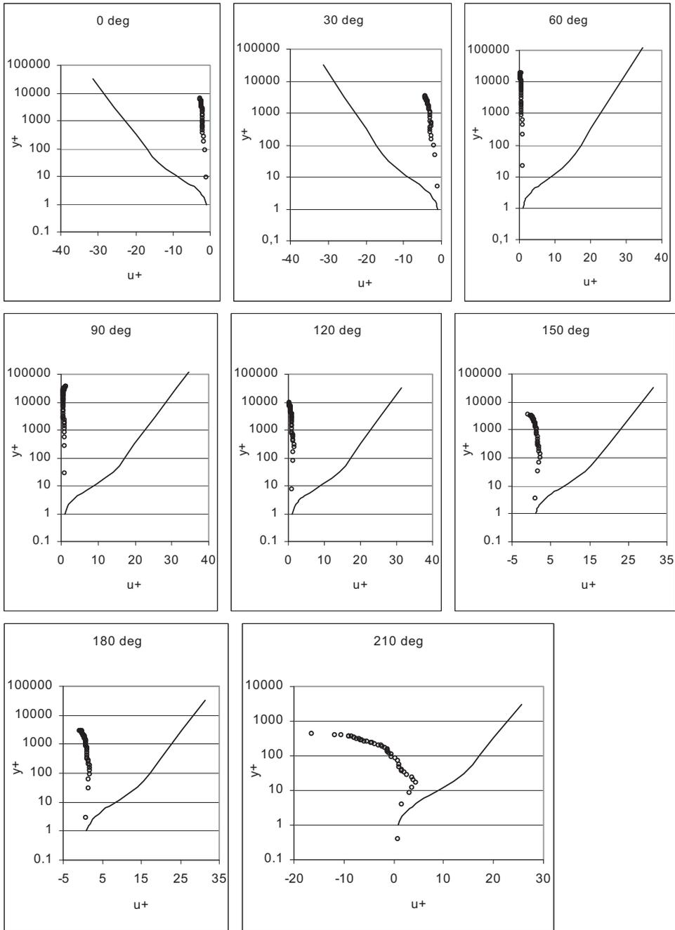
Figure 17 Dimensionless velocity profiles of  $u^+$  at different phases of the wave breaking: section  $(x - x_b) / h_b = 0.09$
