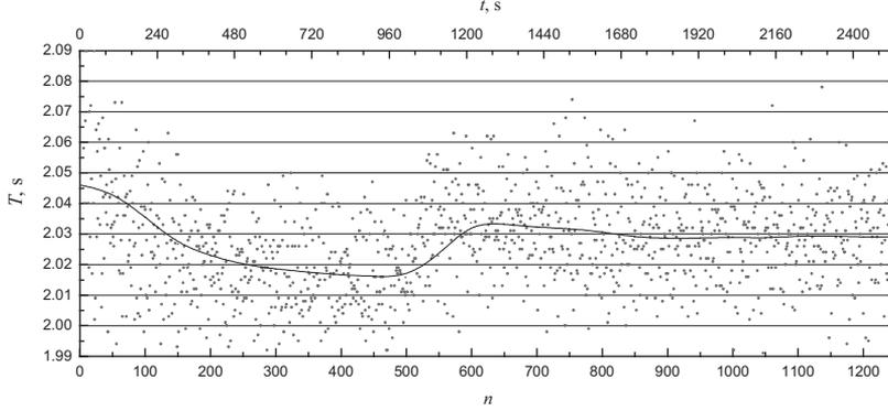
**Fig. 2.** Stabilization of the wave periods after the start of the wave generator;  $n$  – number of the wave.
