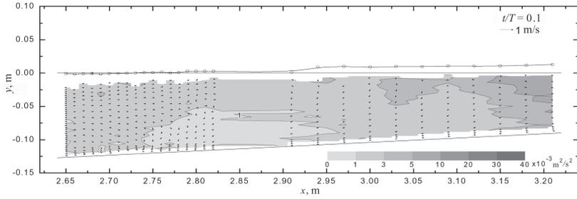
**Fig. 8.** Turbulent kinetic energy and velocity field at  $t/T = 0.0$  and  $0.1$ .
