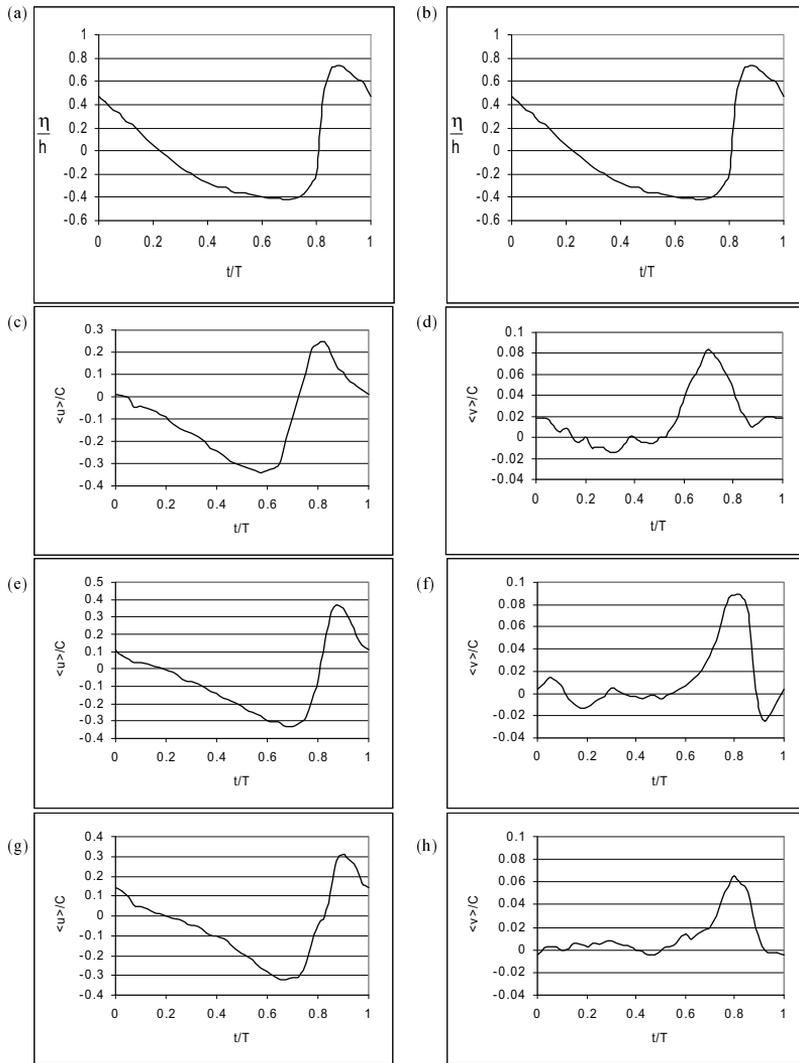
**Fig. 2.** Ensemble-averaged horizontal (left) and vertical (right) velocities at different locations above the surf zone bed: (a), (b) wave profiles; (c), (d)  $z/h = 0.522$ ; (e), (f)  $z/h = 0.352$ ; (g), (h)  $z/h = 0.131$ .
