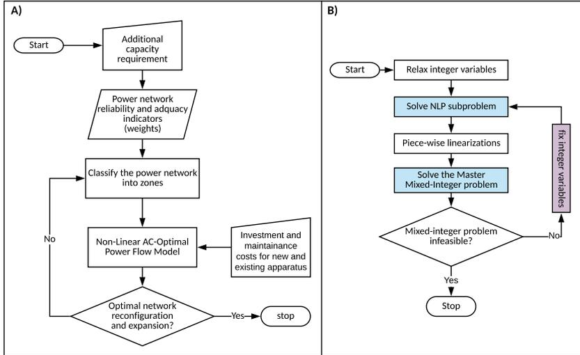
Figure 12 – Flow chart demonstrating the process for (a) expansion planning considering reconfiguration (b) Outer Approximation algorithm
