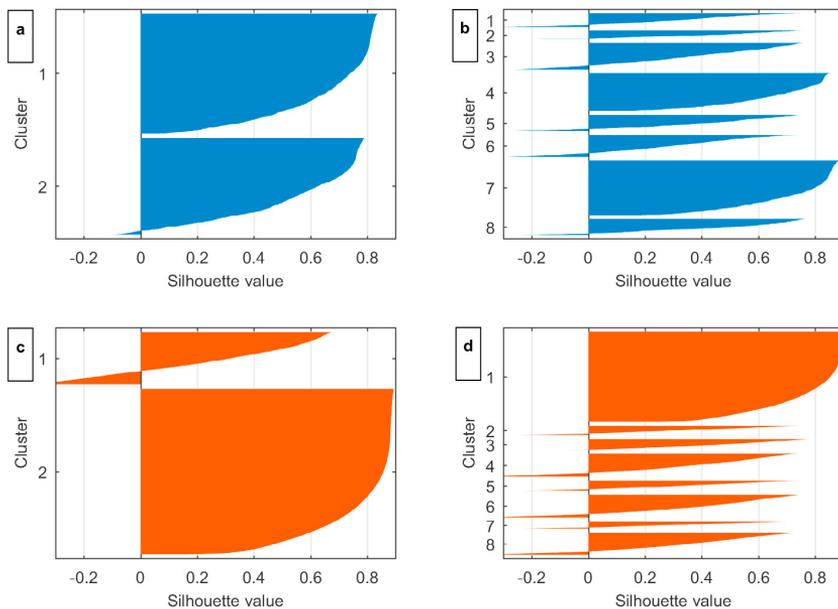
Fig. 5. Silhouette plots of aggregated data: (a) wind turbine data and 2 clusters (b) wind turbine data and 8 clusters (c) wind park data and 2 clusters (d) wind park data and 8 clusters.
