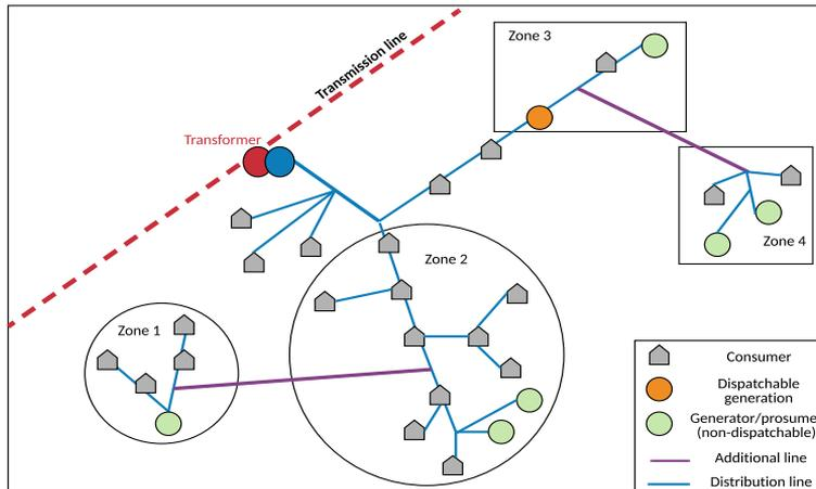
Figure 2 – Power distribution network divided into multiple zones
