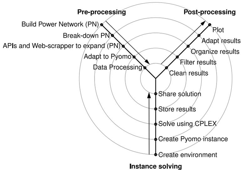
Figure 9 – Decision support system work flow
