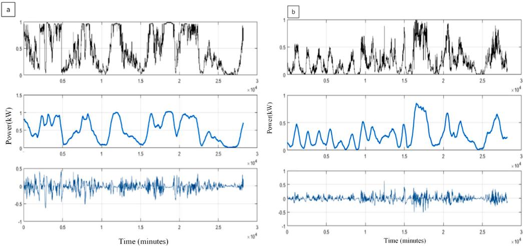
Fig. 3. (a) wind turbine power data; (b) wind park aggregated data.
