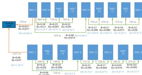
Fig. 1. Layout of the analysed wind farm.
