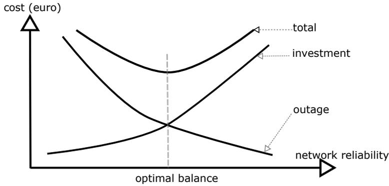
Figure 10 – Relationship between power network reliability and cost
