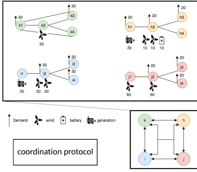
Figure 7 – An instance demonstrating the coordination protocol for four microgrids-  $k, h, i, j$
