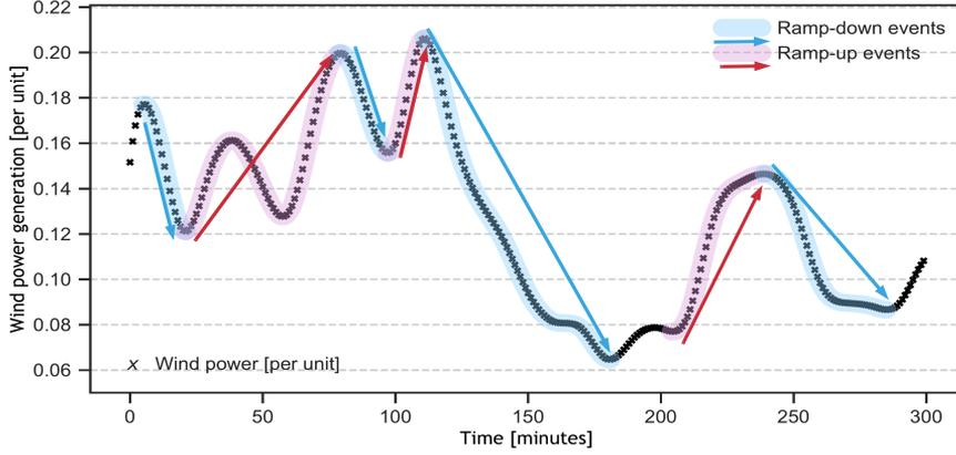
Figure 6 – Wind ramp detection with 10% threshold
