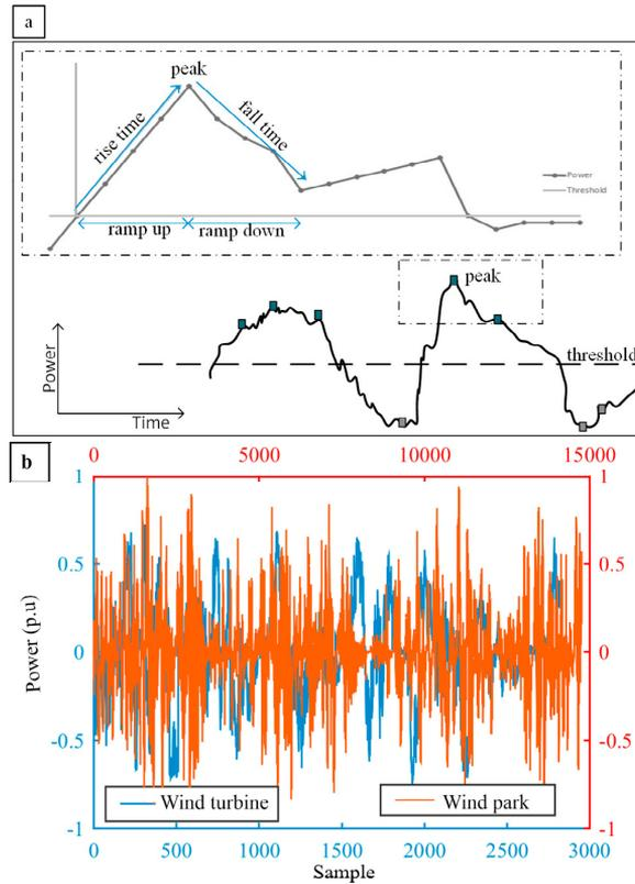
Fig. 1.(a) ramp event (b) wind power swings
