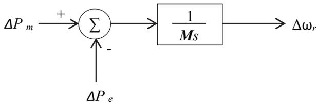
Figure 4.3 Transfer function relating speed and power
