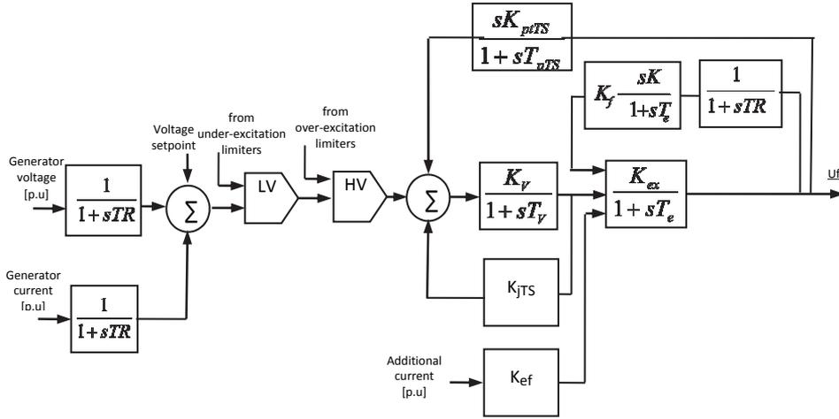
Figure 3.3 Block diagram of automation of a high frequency AC machine excitation system.
