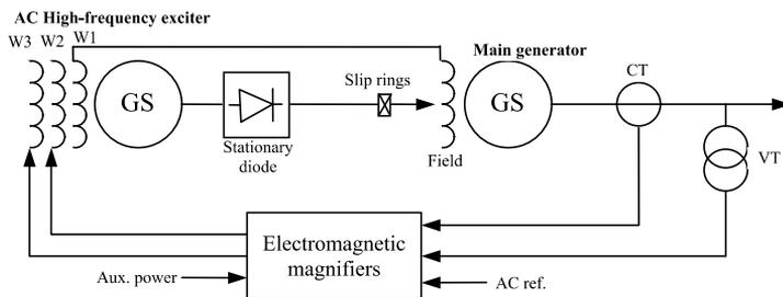
Fig. 5. Excitation system of the high-frequency AC machine.
