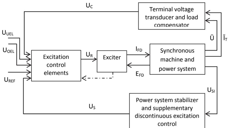
Figure 3.1 General block diagram for a synchronous machine excitation control system
