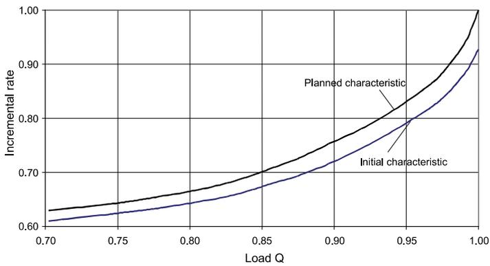
Fig. 1. Initial and planned characteristics of the boiler.
