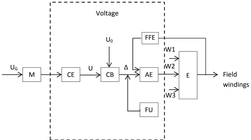
Figure 3.2 AVR block diagram
