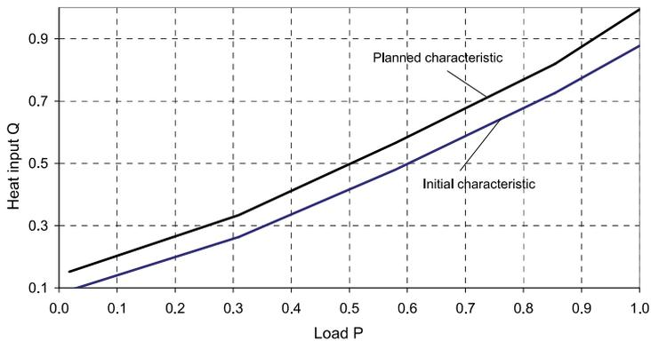
Fig. 2. Initial and planned characteristics of the turbine.
