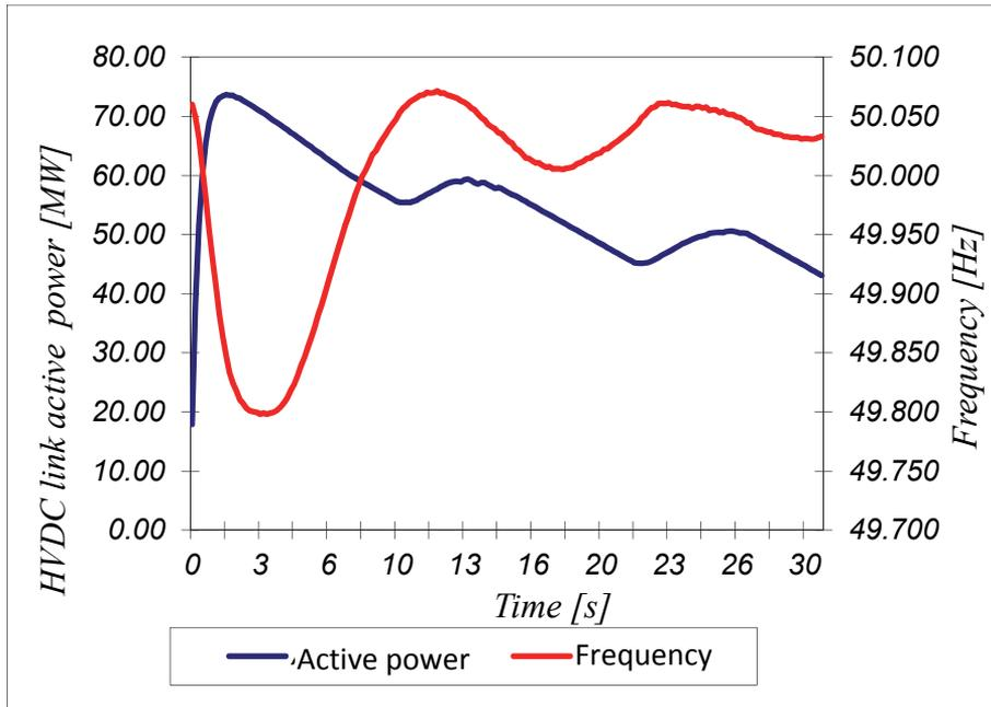
Figure 5.6. Active power fluctuations of HVDC and Estonian power system frequency during HVDC link switch on
