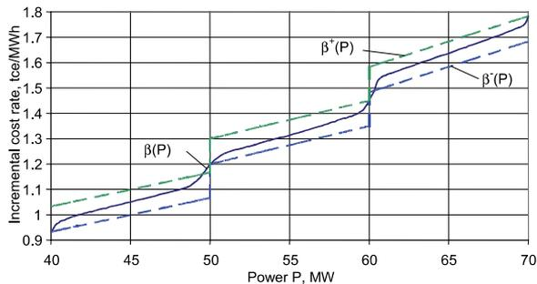
Fig. 5. Initial and planned incremental fuel cost rate characteristics (in relative power units) of a power unit.
