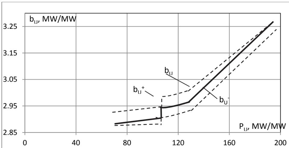
Figure 6.4 Uncertainty zone of the incremental fuel cost characteristic of the double power unit
