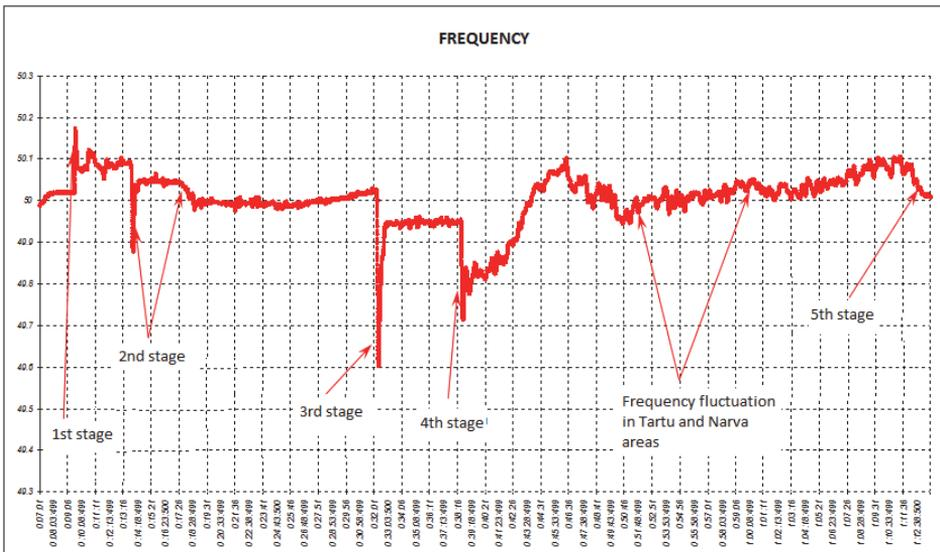
Figure 5.5. Frequency change in the Estonian power system during the isolated operation
