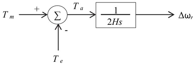
Figure 4.2 Transfer function relating speed and torques
