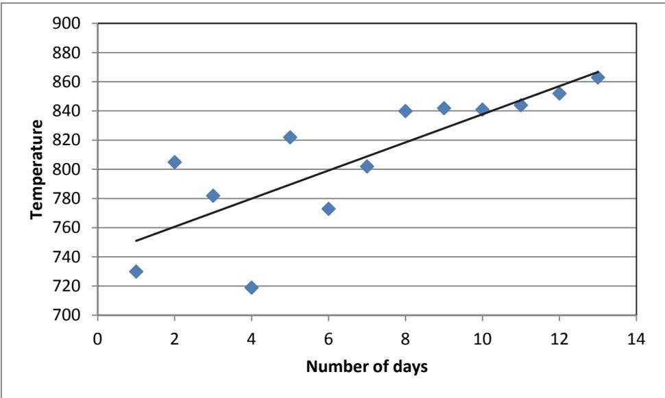
Figure 6.2. Temperature change in the reversing chamber after yearly maintenance
