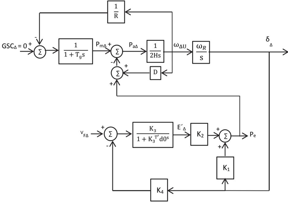
Figure 2.4 Block diagram of a generator with the governor speed regulation
