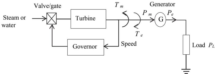
Figure 4.1 Generator supplying isolated load
