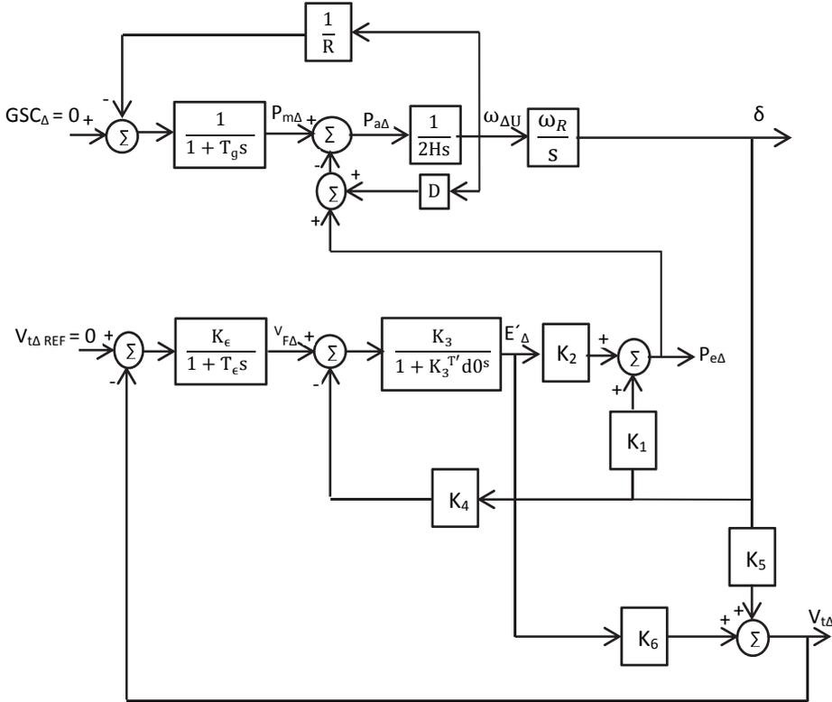
Figure 2.5 Block diagram of a generator with a governor and a voltage regulator
