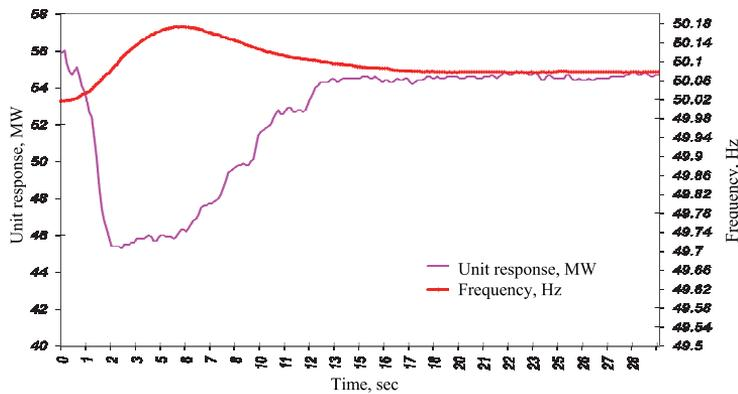
Fig. 2. Response of the large unit to failure produced by network event.
