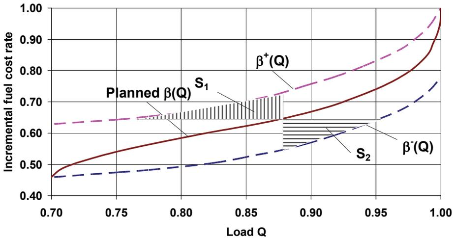
Figure. 6.5. Initial (lower and upper) and planned characteristics of a boiler
