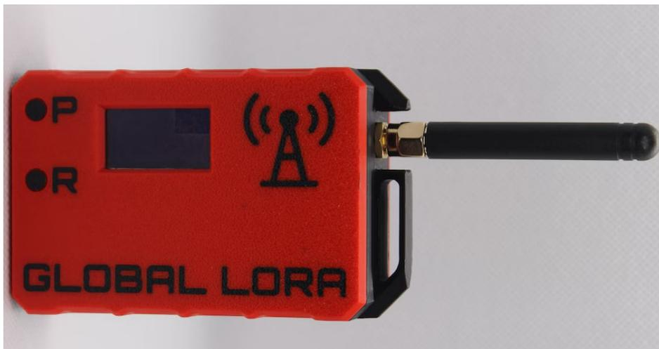
Figure 3.6 TerraNode Meshtastic device [47]
