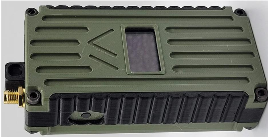
Figure 3.3 3D printed case for RAK4631 with RAK19007 base board [43]
