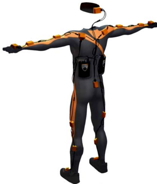
Figure 4.3. Suit with 17 inertial sensor modules [23].
