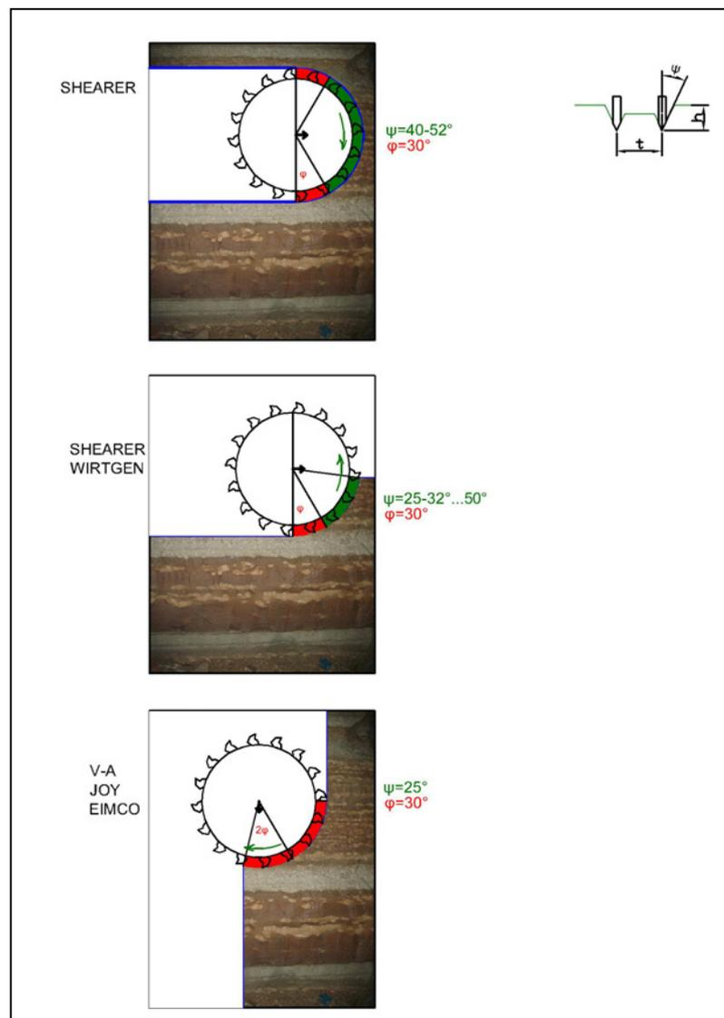
Figure 3: Oil shale cutting principles 1-3
