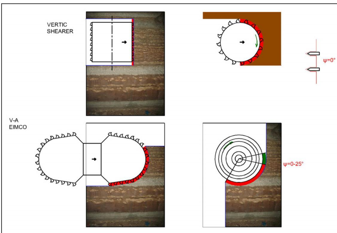
Figure 4: Oil shale cutting principles 4-5
